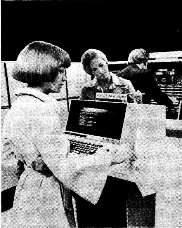
*The UNIVAC 1100/40, introduced in 1975 as the successor to the 1110, features semiconductor primary and extended storage, twice the primary storage capacity of the 1110, and up to one million words of directly addressable extended storage.*
