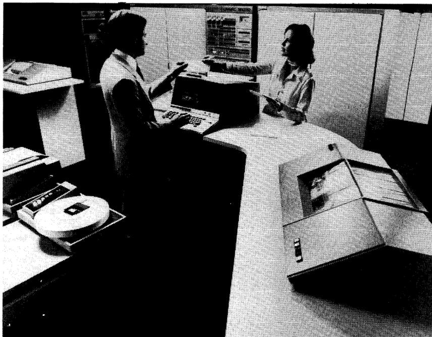
*The UNIVAC 1100/80, introduced in November 1976, is Sperry Univac's most powerful computer to date and is designed to compete directly against the IBM System/370 Model 168. The 1100/80 is the first 1100 Series computer to employ high-speed buffer storage. It can have up to 16 million bytes of main memory and is available in both uniprocessor and dual-processor configurations.*
