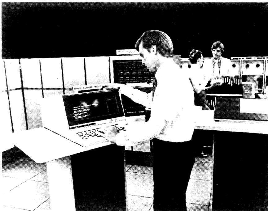
*UNIVAC 1100/20 configurations feature up to 524K words of semiconductor main memory, a CRT system console, and an optional Communications/Symbiont Processor with expanded communications capabilities. Rental for 1100/20 systems ranges from about \$25,000 to as much as \$80,000 for a large system.*
