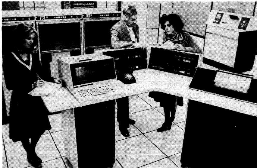
*The UNIVAC 1100/10 was introduced as a lower-cost alternative to the 1100/20. It is now available with a choice of three main memory speeds (875, 1000, or 1125 nanoseconds), and the fastest of these raises the 1100/10's processing power to the level of the 1100/20.*
