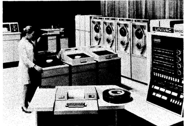
*This closeup of the 9400 console also shows three of UNIVAC's 2311-compatible 8411 Disc Drives.*
