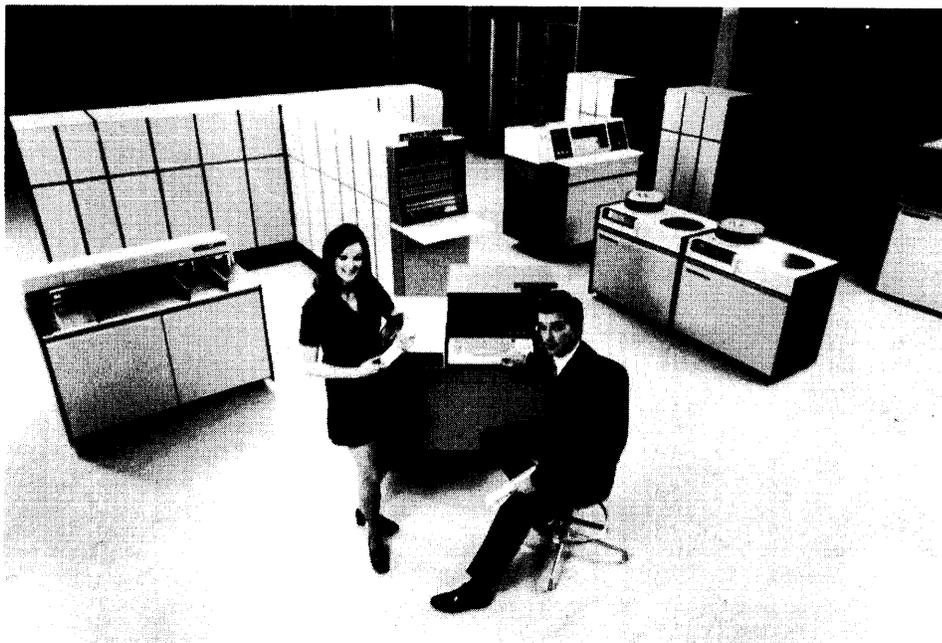
*This view of a fairly small, disc-oriented UNIVAC 9700 configuration shows the CRT-equipped System Console in the foreground and the Central Processor at left rear.*
