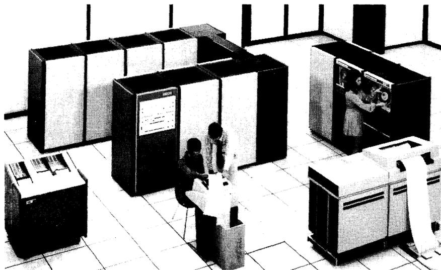
*The Sigma 8 computer system is oriented toward real-time and scientific applications. It was developed for use in process control, manufacturing, education, health care, research, and other high-technology environments.*
