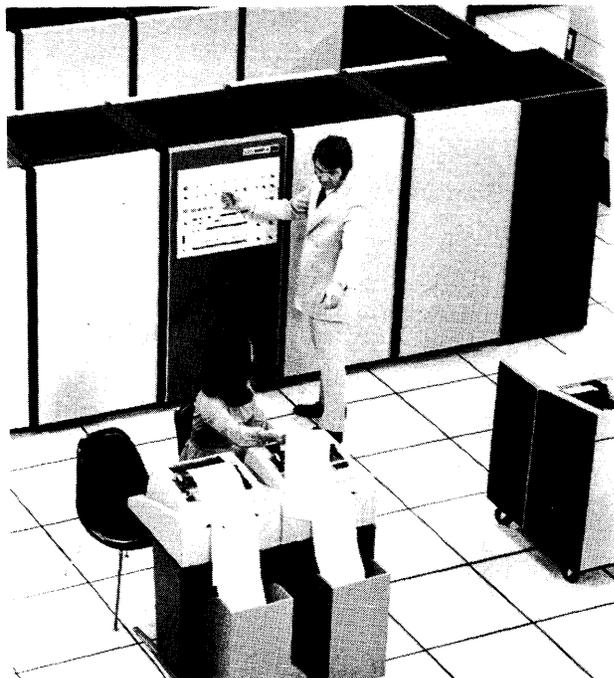
*The top-of-the-line Sigma 9 system, designed for general-purpose business and scientific applications, offers up to 2 million bytes (524K 32-bit words) of core storage with a 900-nanosecond cycle time.*
