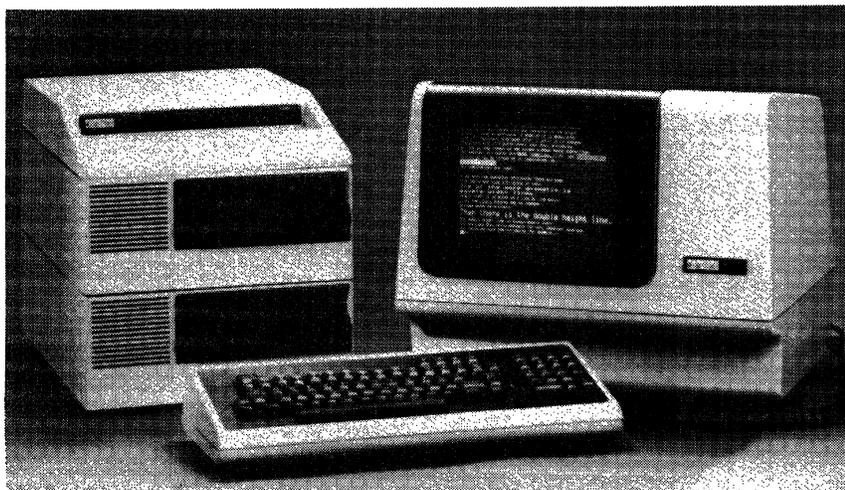
The PDT 11-150 shown here with dual diskette drives on the left is the top of the line of Digital Equipment's user-programmable terminal family. All models employ the LSI-11 microprocessor, making them fully compatible with the DEC PDP-11 minicomputer series.
