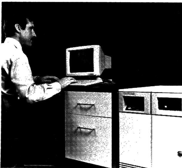
*The 6000 Series is Four-Phase's new 32-bit office information system. Composed of the System 6300 and System 6600 (shown here), the Series 6000 run under a Unix-derived operating system that is based on and compatible with Unix System V. The Series 6000 provides support for up to 128 workstations.*
