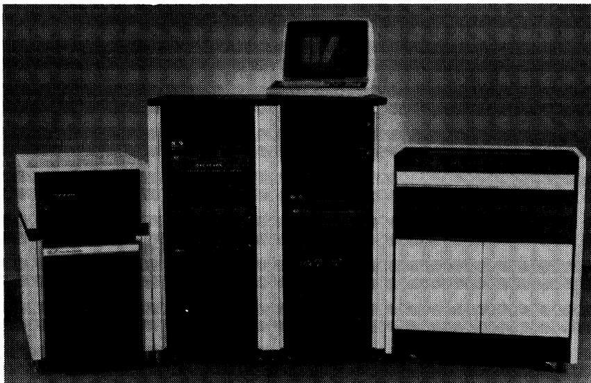
*Four Phase's newest interactive processing system is the IV/95, which includes (from left to right): a Model 8281 80MB disk drive; the IV/95 processor, with Four Phase's new ergonomically designed terminal sitting on top of it; and the Model 8154 1000-lpm printer.*
