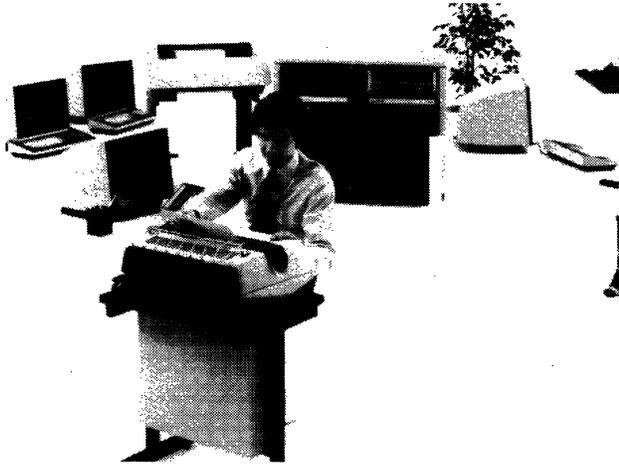
Four-Phase's new System IV/60 features high processing speeds and total compatibility with existing Four-Phase software including the new Multifunction Executive. Positioned as a mid-range processor, a IV/60 with 192K bytes of main memory can support up to 24 1920-character video terminals, up to 22.5 megabytes of disk storage, and a variety of printers.
