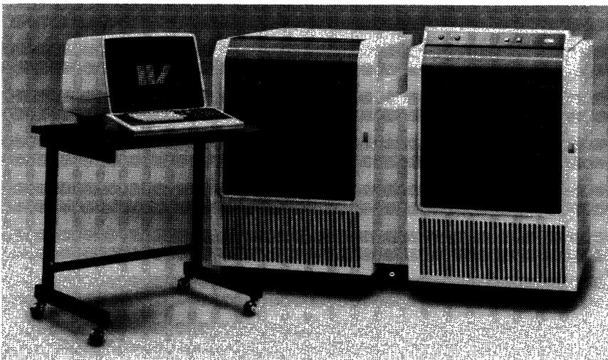
*The Series 5000 family from Four-Phase provides the multi-site user with up to 6MB of RAM memory, up to 2.2 billion bytes of disk storage, and support for up to 128 of the company's Fastrak intelligent workstations with printers. Broadband local area networking capabilities are available to Series 5000 users through Four-Phase's Net IV LAN. A personal computing feature, touch-sensitive display, and voice store and forward capabilities can also be added to the Series 5000.*
