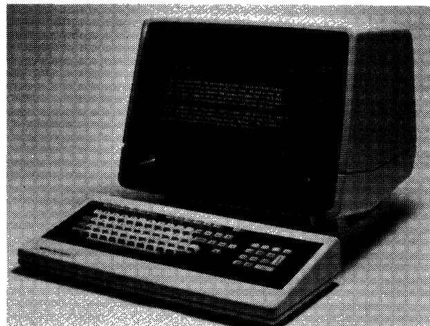
*A new ergonomically designed keyboard/display was designed for use with Four Phase's Series IV/80 and IV/95 systems. The new unit features a redesigned keyboard, palm rests, tiltable screen with anti-glare filter, optional amber character read-out (green read-out is standard), and a new charcoal and white cabinet.*
