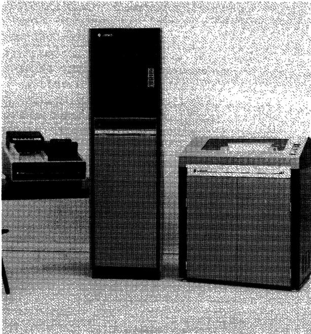
Typical Unitech peripherals include (from left) a card reader, magnetic tape drive (UT-1 and UT-4 only), and line printer. The Data General minicomputer is housed in the central cabinet along with the tape drive.
