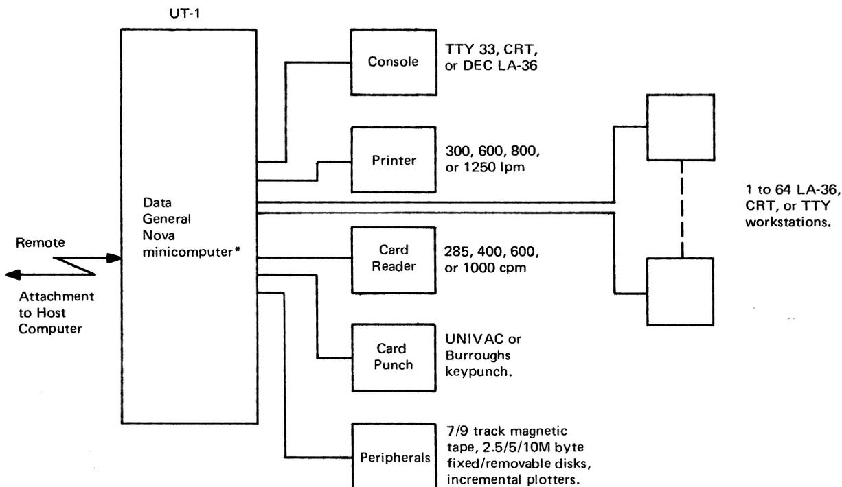
\*A microprocessor-based version is available; this version supports only the console, printer, card reader, and card punch.
