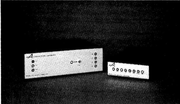
The Avanti Models 120 and 170 interface converters shown here represent the two types of physical characteristics of the seven models.
