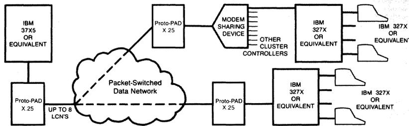
Figure 2. Dynapac's Proto-PAD X.25 allows IBM 37X5 or compatible machines to communicate with 327X controllers over an X.25 link.
