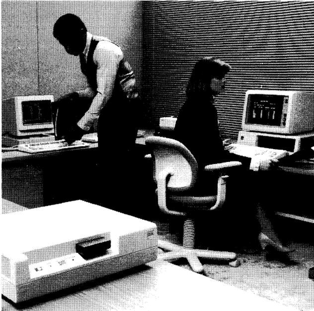
IBM's 3708 Network Conversion Unit, pictured in the foreground in the photo to the above, consists of a base unit and a plug-in cartridge for system microcode.
