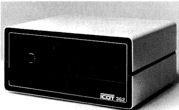
*Icot's 362 protocol converter emulates an IBM 3274 21C or 51C cluster controller. The unit will allow up to 16 asynchronous ASCII devices to emulate IBM 3270 displays and printers. The synchronous link to the host supports the SNA/SDLC protocol. The 362 will support two host lines; the second line is available as an option.*
