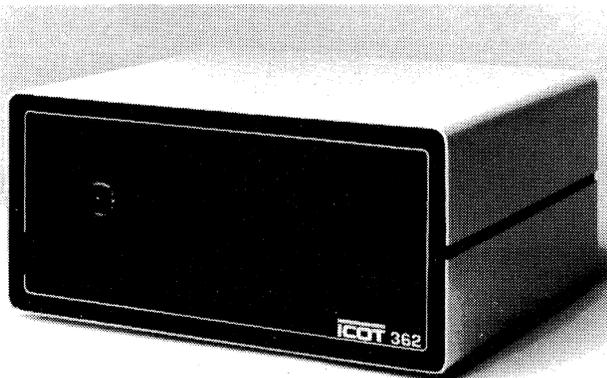
*Icot's 362 protocol converter emulates an IBM 3274 21C or 51C cluster controller. The unit will allow up to 16 asynchronous ASCII devices to emulate IBM 3270 displays and printers. The synchronous link to the host supports the SNA/SDLC protocol. The 362 will support two host lines; the second line is available as an option.*
