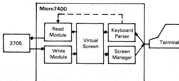
Figure 1. Micro7400 functional block diagram.
