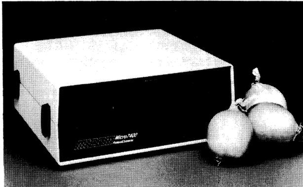
*The Micro7400 protocol converter emulates an IBM 3274 controller and allows asynchronous devices to function as 3270-type terminals and printers with an IBM-compatible host processor.*
