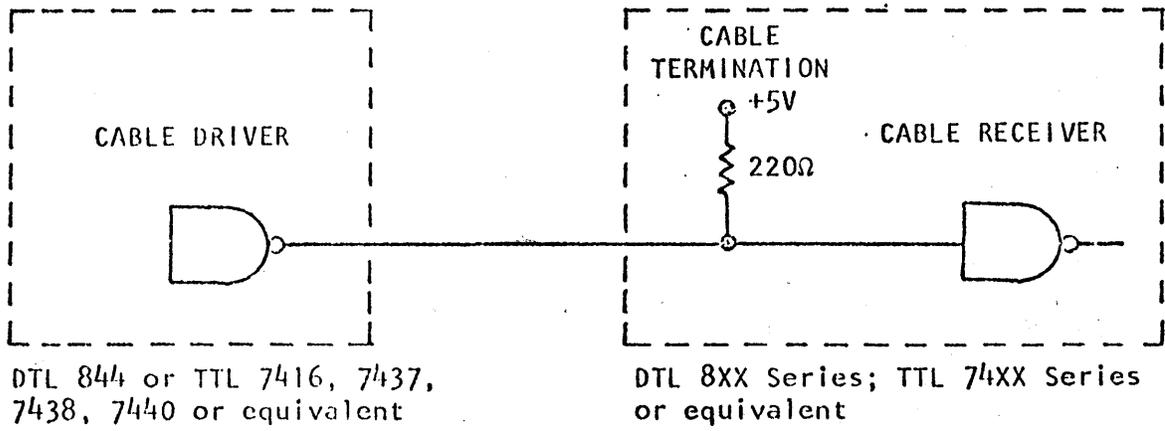
Figure 1-3. Interface Circuits
