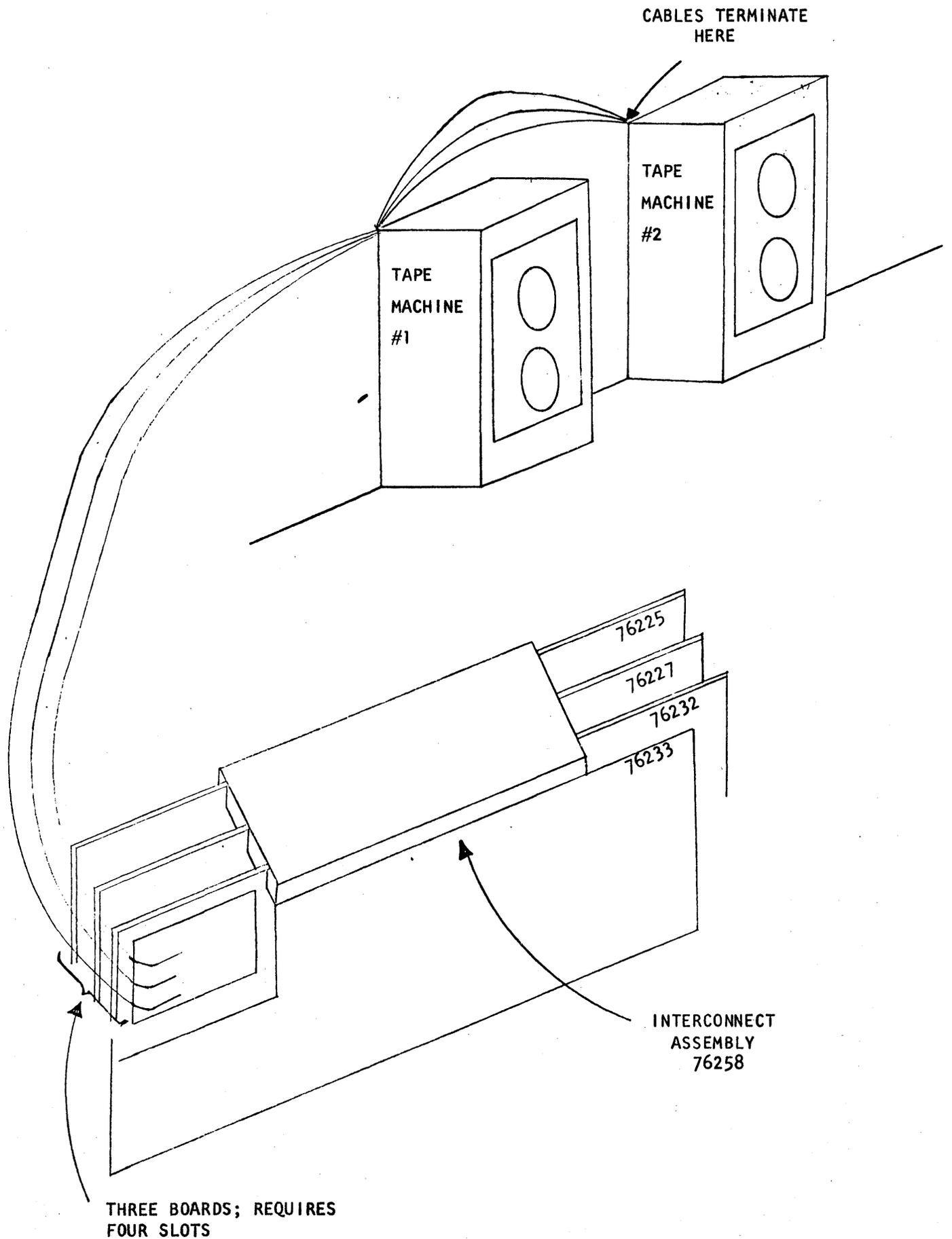
Figure 1-1. Installation of Model 5091 NRZI Controller
