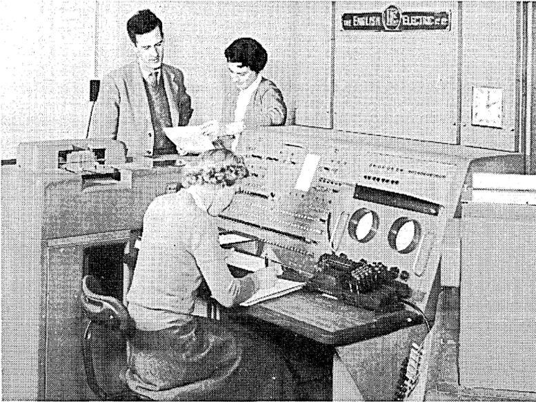
Fig. 13.3 The control desk of an English Electric DEUCE computer. First delivered in 1955, this machine was the production version of the NPL Pilot ACE. Input was via the punched-card reader to the left of the photograph. The black hand-punch lying on the right of the control desk was no doubt only for quick card edits.
