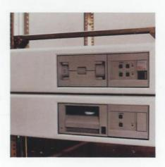
Working with the customer, Digital integrated third-party disk drives with the VAXstation 3200 workstations, communications modules and memory. The entire package was designed to reside in yet another third-party cabinet, and the entire solution was supported by Digital.
