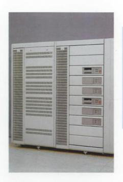
Working with the customer, Digital provided a two-cabinet solution. One cab contained two FATBOX CPUs, the other contained 204 synchronous communications lines with SIMPACT 1622 and 3222 communications modules. Careful redesign for air flow and emissions requirements are part of the Digital services provided on any specially-configured system.
