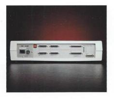
DECserver 250 meets the open office acoustic requirements of Digital Standard 104 (55db), and is fully compliant with UL, CSA and FCC regulations.
