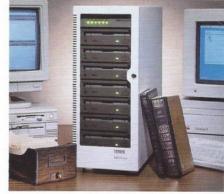
the other with seven. With the four-drive version, you can add hard disk and magneto-optical devices external to the InfoTower cabinet, or combine already existing CD-ROM drives into it.
