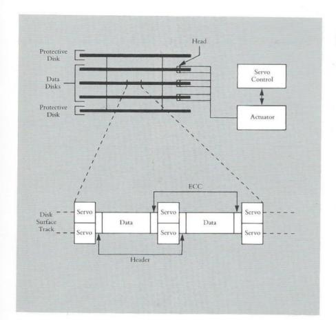
The RA60's "fully embedded servo" positioning system frees you from routine maintenance and ensures that a disk pack written on one drive can be read on any other.
