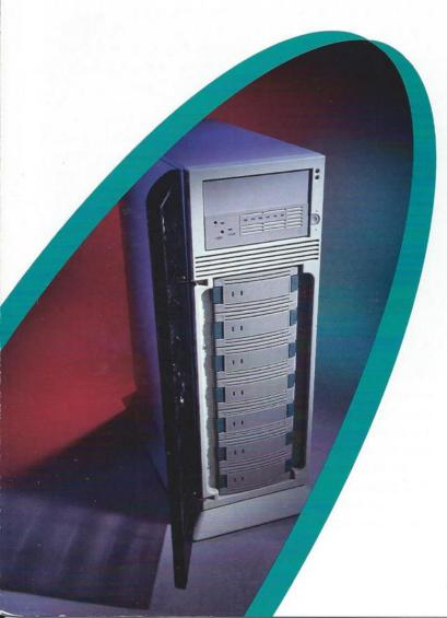
You can't afford to slow down — or stop — if a component or disk fails. So stay up-to-speed with StorageWorks RAID Array Subsystems. Disk mirroring and Parity RAID, combined with redundant, hot-swappable components and drives, ensure your data is available when you need it. While controller-based RAID, disk striping and battery protected write-back cache actually boost application performance.
