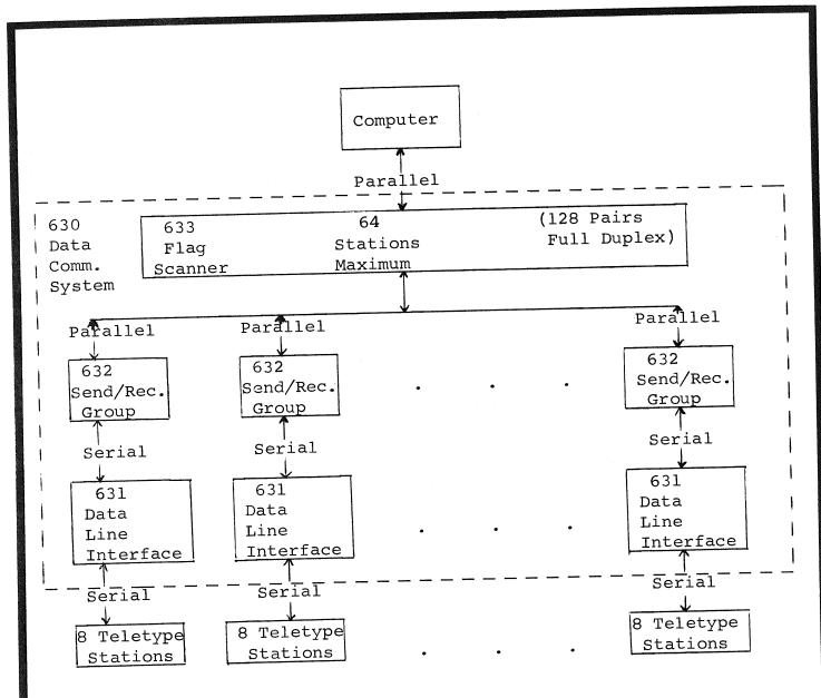
The above 630 System has a maximum capacity of eight (8) groups (8 stations per group) or 64 stations. (128 pairs of wires for Full Duplex operation).
