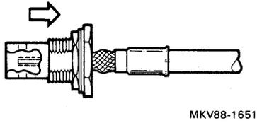
21. Slide the ferrule to the rear of the connector and crimp it onto the cable.
