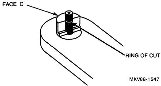
8. Rotate the tool clockwise until cutting stops.
