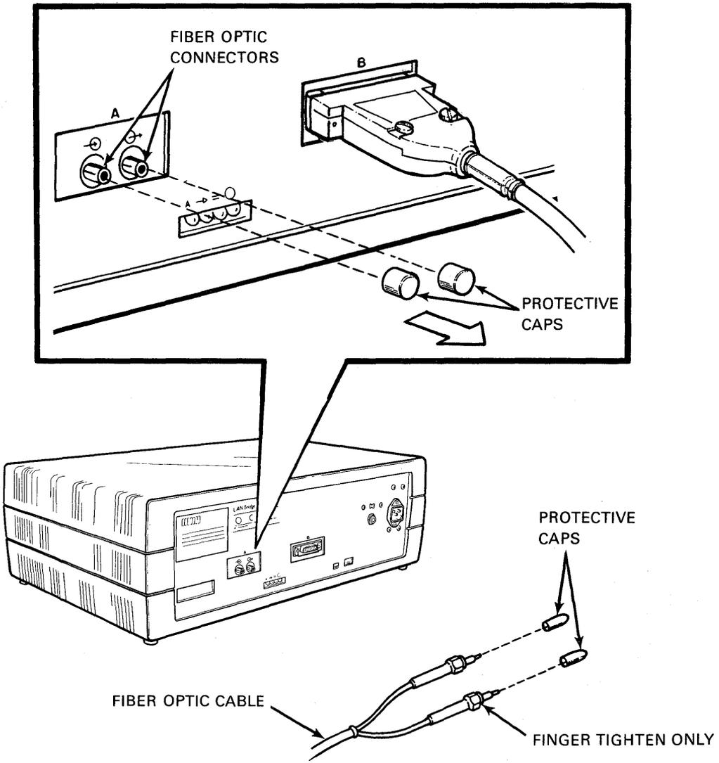
Figure 16 Fiber Optic Cable Attachment
