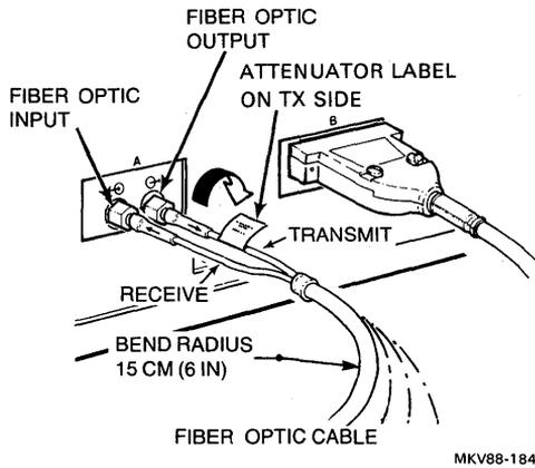
Figure 18 Connecting Fiber Optic Cable to DEBET-RH/RJ
