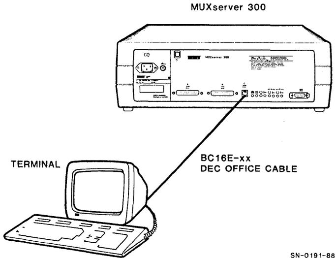
**Figure 12 Supervisor Port Connection**
