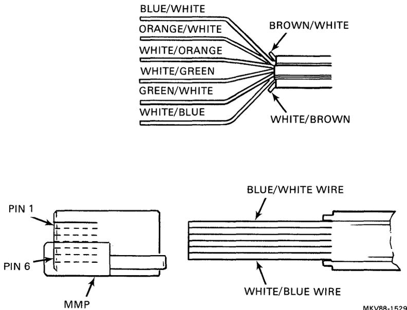
5. Insert the cable into the MMP connector and push it in as far as it will go (about 1/4 inch).
