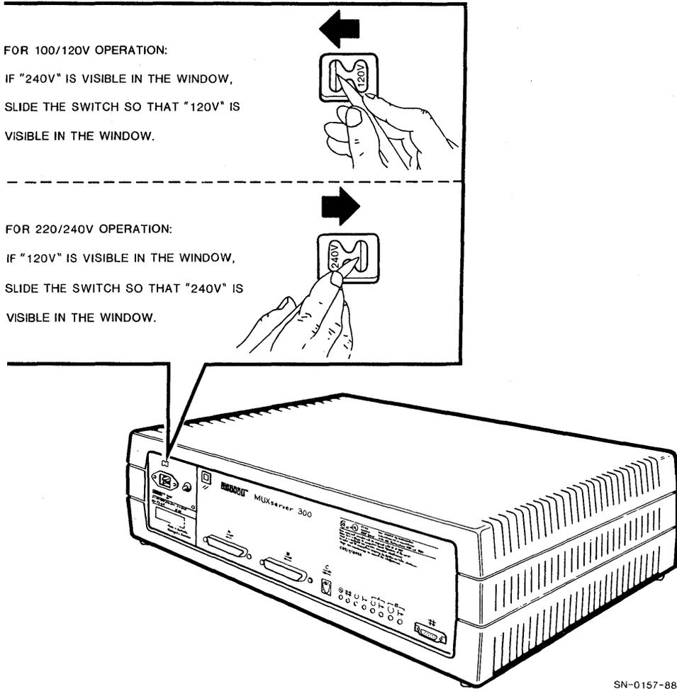
Figure 8 Selecting Operating Voltage
