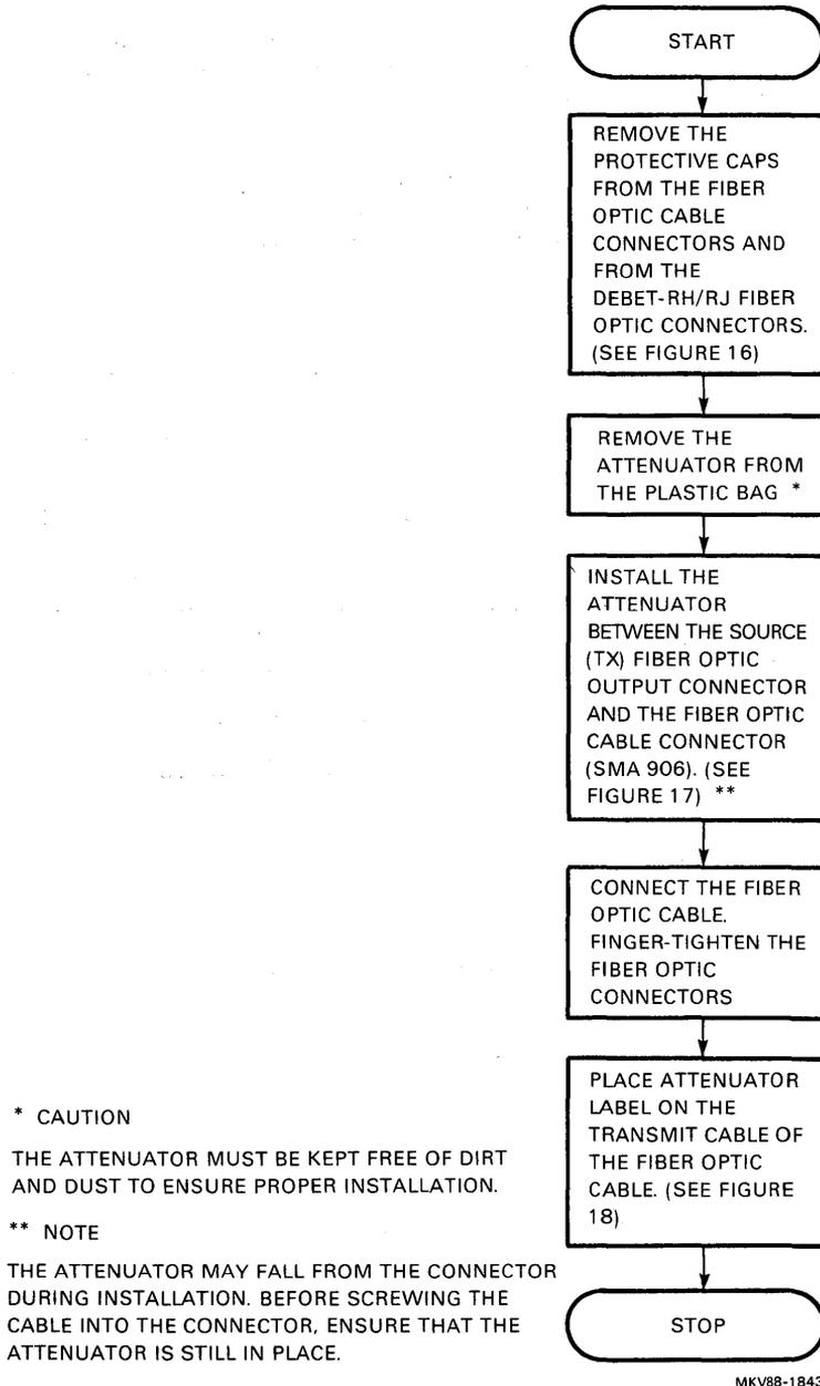
Figure 6 DEBET-RH/RJ Attenuator Installation Flowchart
