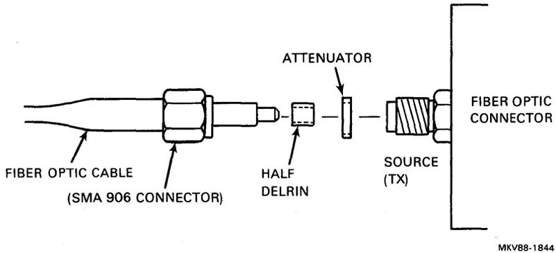
Figure 17 Installing the Attenuator
