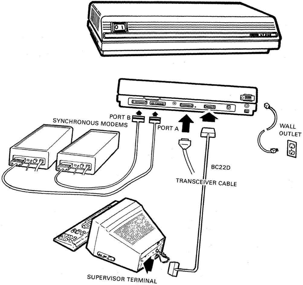
Figure 5 Front and Rear Panels of the MUXserver 100
