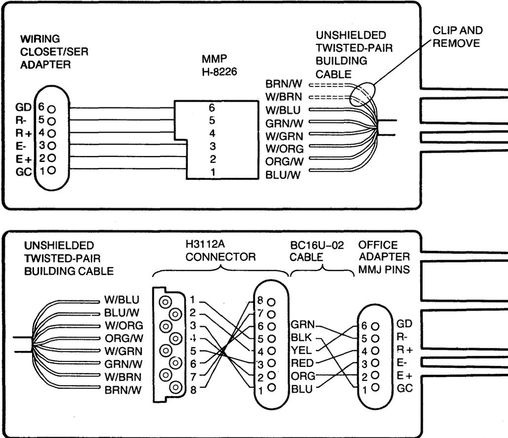
Figure 16 AT&T Unshielded TP Connections (Sheet 1 of 2)
