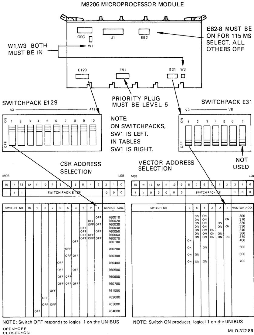
Figure 5 M8206 Microprocessor Module Configuration
