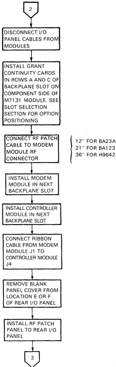
Figure 5 Installation Flowchart for DTQNA in BA23A, BA123, and H9642 Systems (Sheet 2 of 5)
