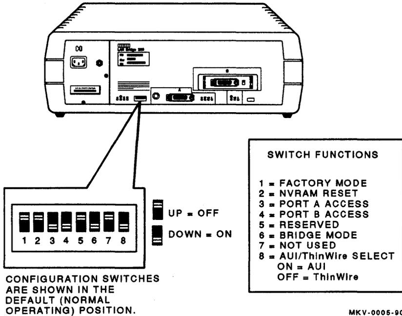
Figure 7 Configuration Switch Settings
