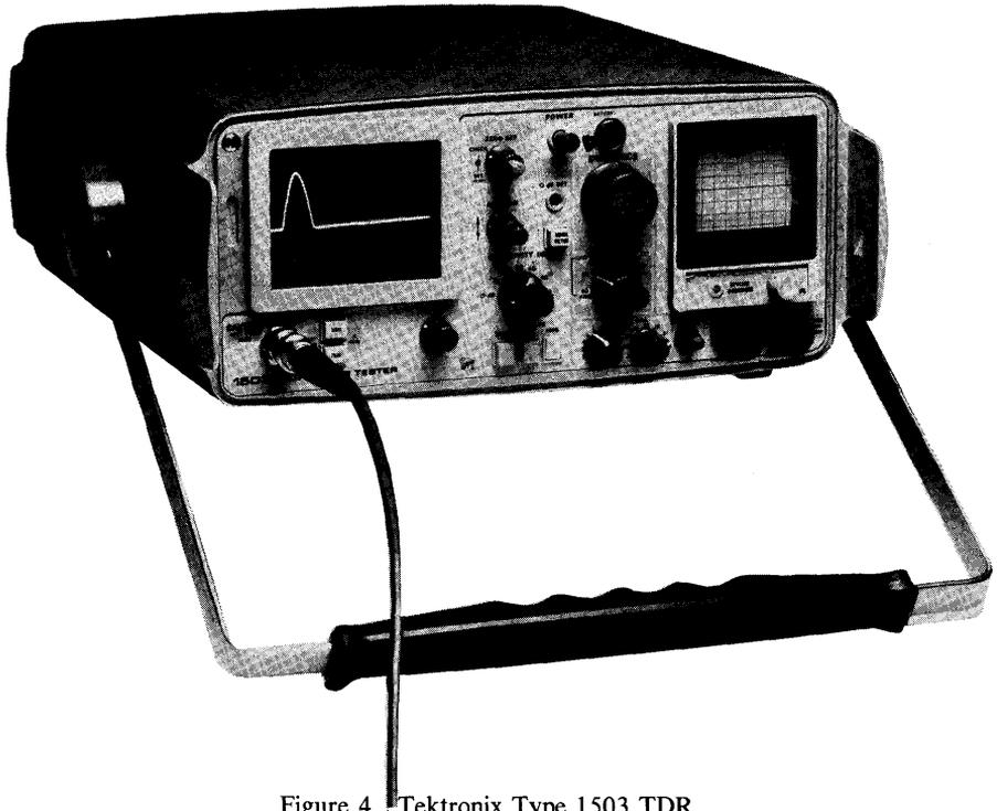
Figure 4 Tektronix Type 1503 TDR
