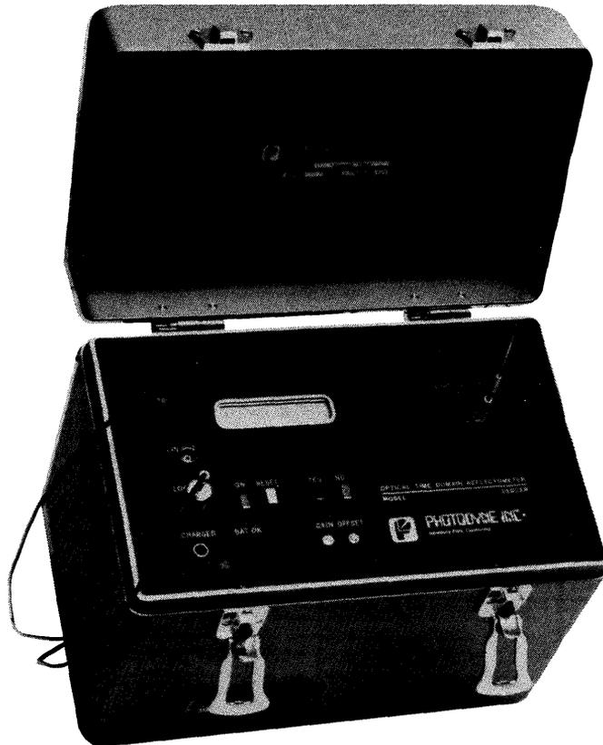
Figure 6 Photodyne Model 5500 FOTDR
