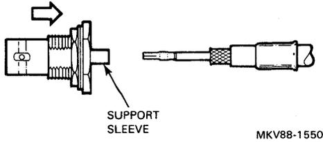
20. Slip the support sleeve under the braid and over the dielectric and foil shield. The center conductor must be flush or within 1/16 inch of the end of the connector.
