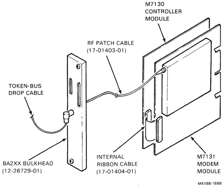
Figure 9 DTQNA Internal Installation in BA2XX Systems (DTQNA-BA)
