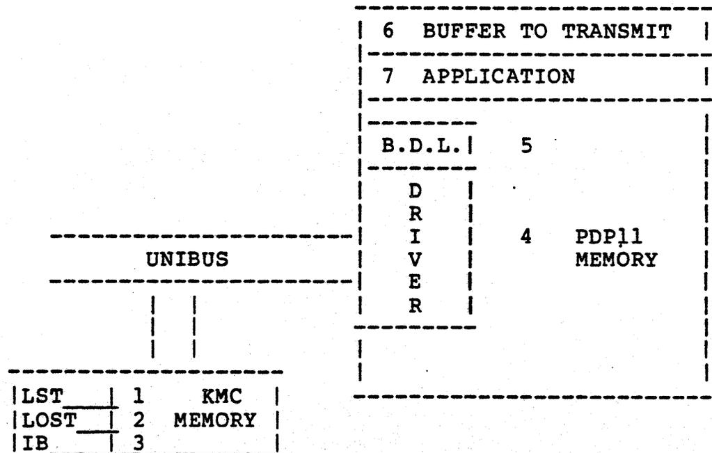
Application program (7) passes to driver (4) a request for a message to be transmitted. It specifies the BDL MEMBER (5) that contains the address and character count of the buffer to be transmitted.
