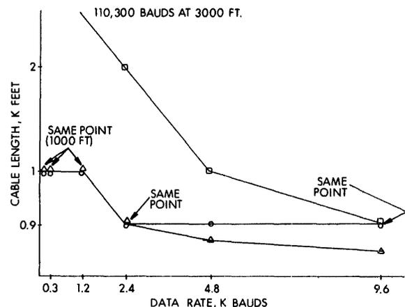
□ Cable is 3 twisted pair, no. 22 AWG stranded, each pair shielded, Belden no. 8777, DEC P/N 91-07723; shields connected to common leads at both ends.
