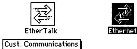
Select the Ethernet icon to enable your Macintosh computer to use TCP/IP to communicate with other TCP/IP hosts on the network. (AppleTalk is already being used to communicate with the AppleShare® File Server and LaserWriter.)
