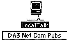
The box beneath the icon displays your network zone. If your gateway is located in another zone, direct the pointer to the zone box and hold down the mouse button. A pop-up menu appears with a list of zone names as shown in Figure 6-4. Keeping the mouse button down, slide the pointer to the list and highlight the appropriate zone. When you let go of the mouse button, the pop-up menu disappears and the zone name you selected appears in the box beneath the icon.
