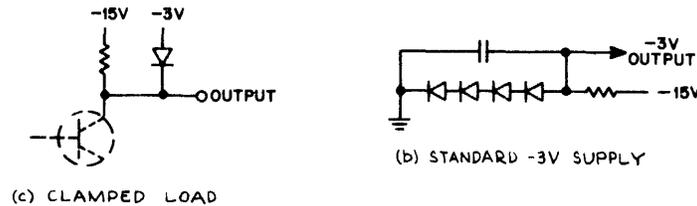
Figure 4-1 Clamped Load and Standard Power Supply
