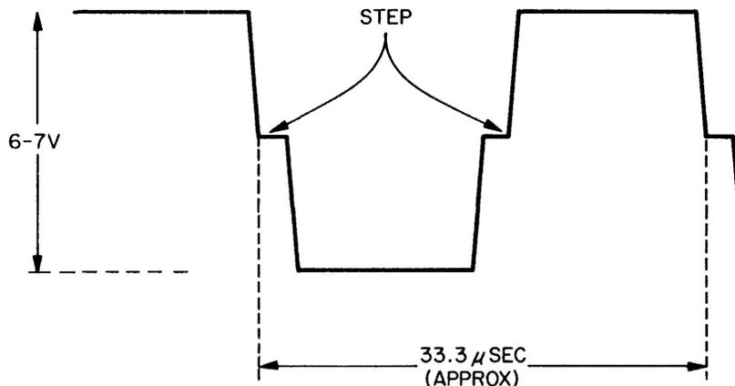
NOTE: The normal pulse period indicated in step g will vary with the speed of the tape. Vernier measurements and adjustments should be performed with the tape advancing in the forward direction.
