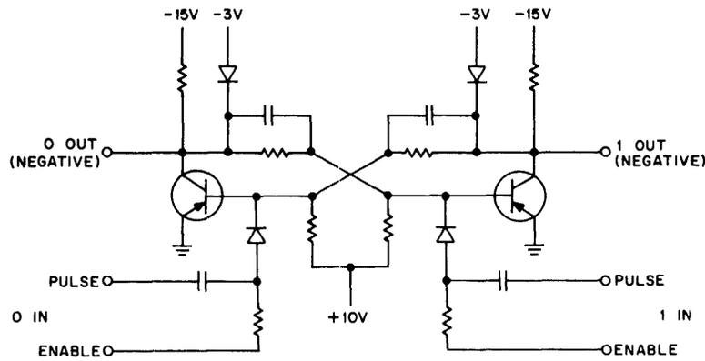
Figure 4-5 Basic Flip-Flop
