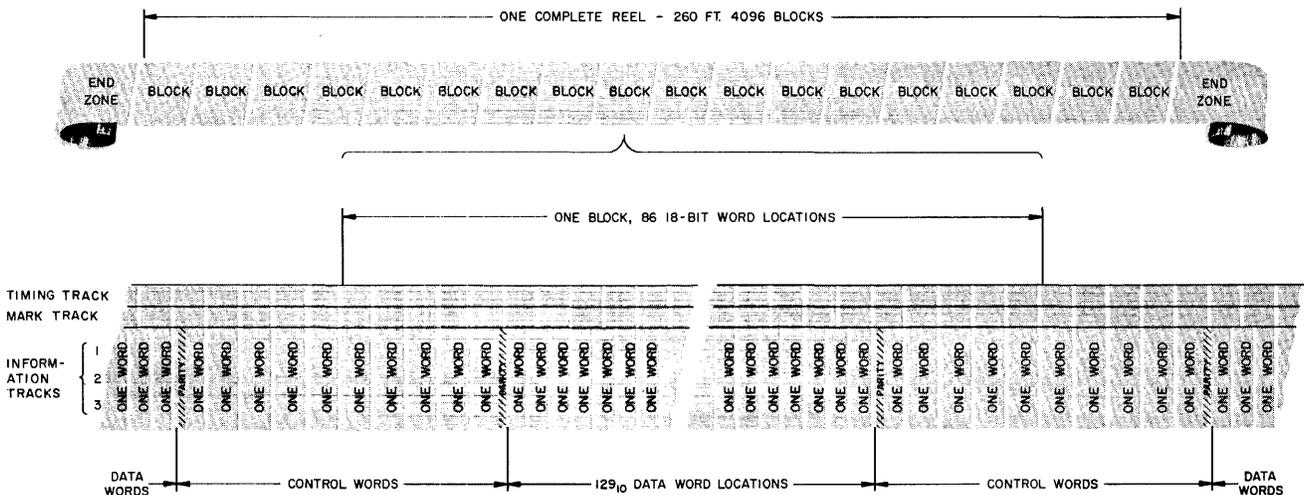
Figure 2-3 DECTape Control and Data Word Assignments
