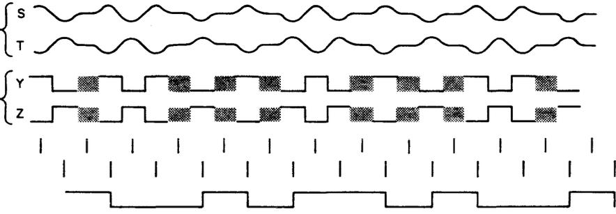
Figure 3-2 Read/Write Waveforms
