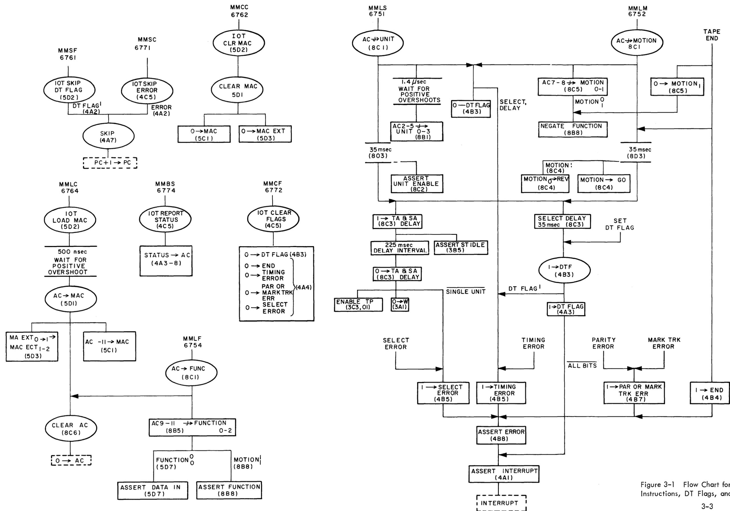
Figure 3-1 Flow Chart for Computer Instructions, DT Flags, and Error Flow
