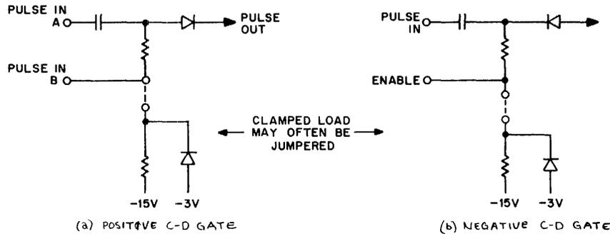
Figure 4-4 Capacitor-Diode (C-D) Gates
