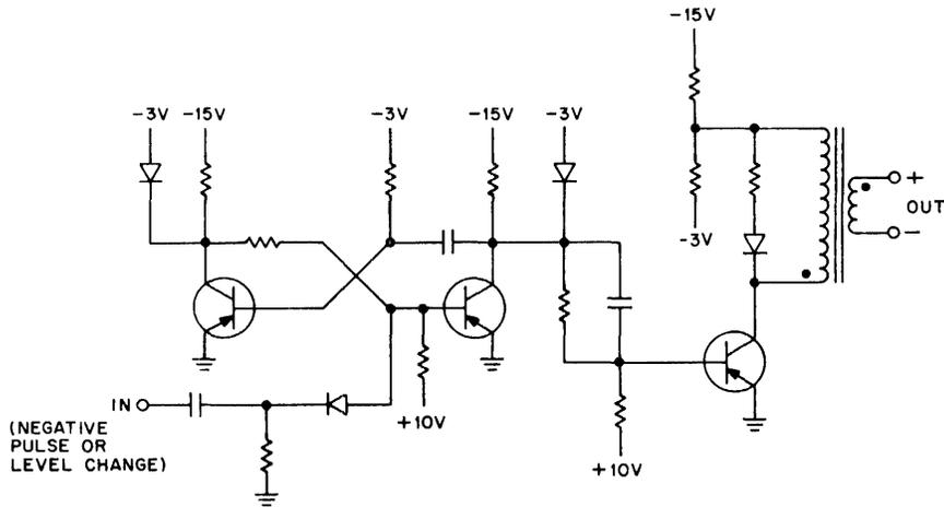
Figure 4-6 Basic MV-Type Pulse Amplifier
