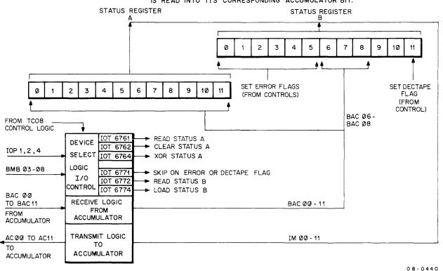
Figure 2-6 TC08 Control Section
