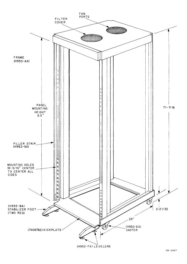
Figure 4-1b H950 Frame, Dimension Diagram
