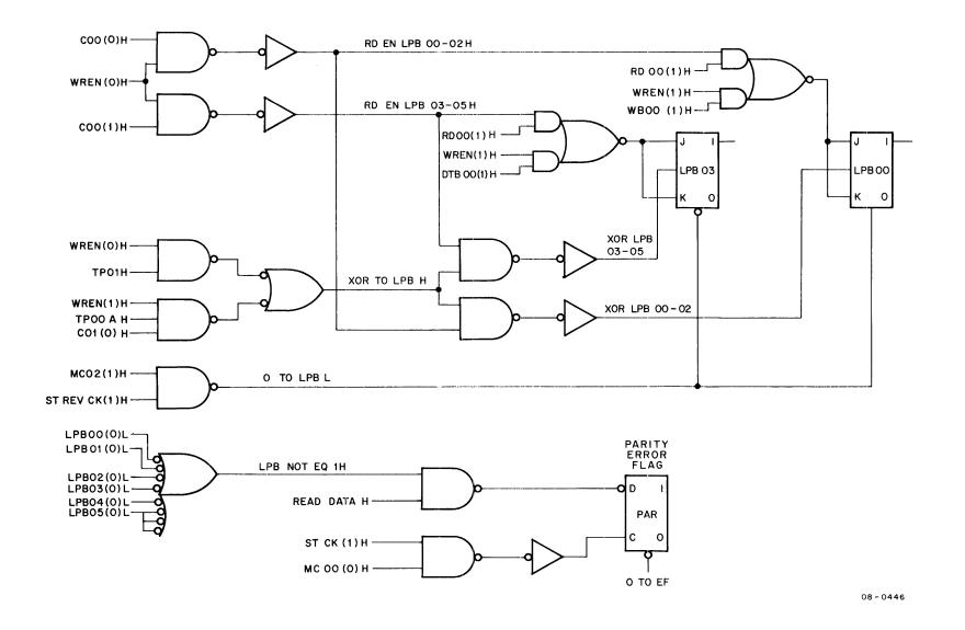
Figure 3-10 The Longitudinal Parity Buffer
