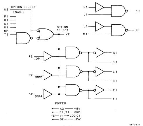
Figure 6-9 The M102 Device Selector
