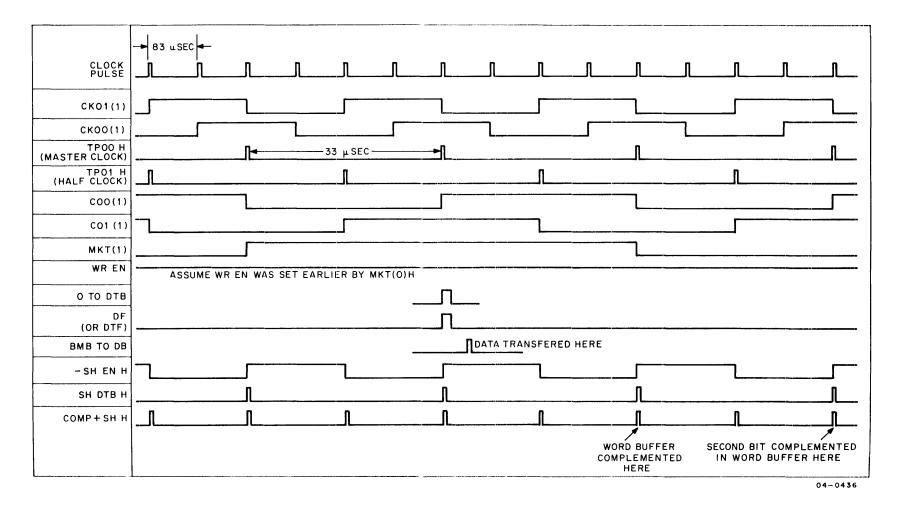
Figure 3-16 Write Timing and Mark Track Timing Diagram
