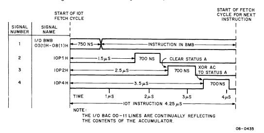
Figure 3-5C Command Register Timing with PDP-8/I
