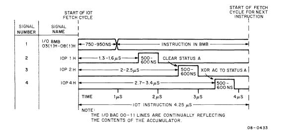
Figure 3-5A Command Register Timing with PDP-8/L
