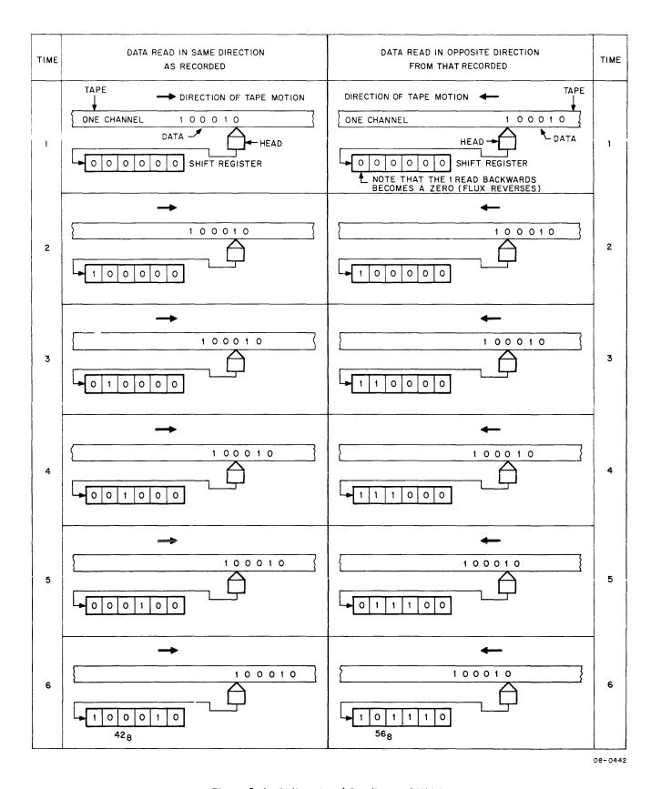
Figure 2-4 Bidirectional Reading and Writing
