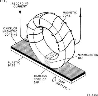
Figure 3-1 Simplified Diagram of the Magnetic Recording Process
