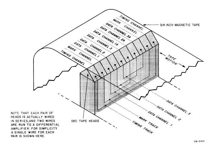
Figure 2-1 DECtape Heads and Tape Channels
