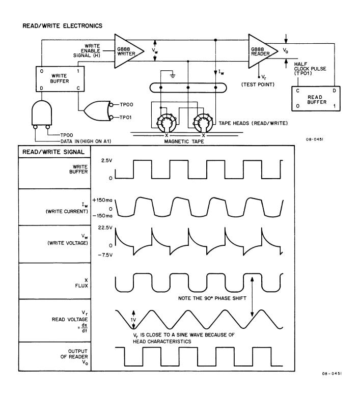
Figure 3-2 DECtape Read/Write Electronics and Waveforms
