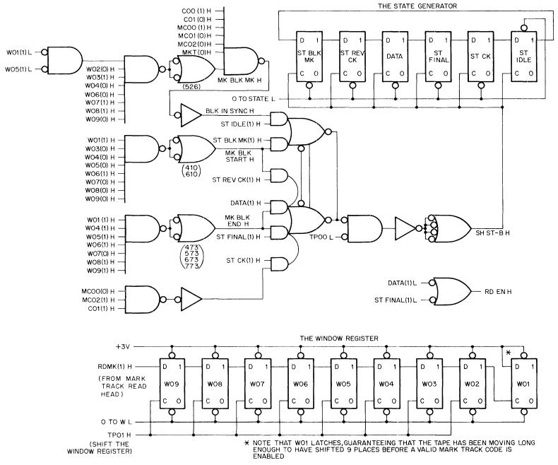
Figure 3-8 The Window Register and State Generator
