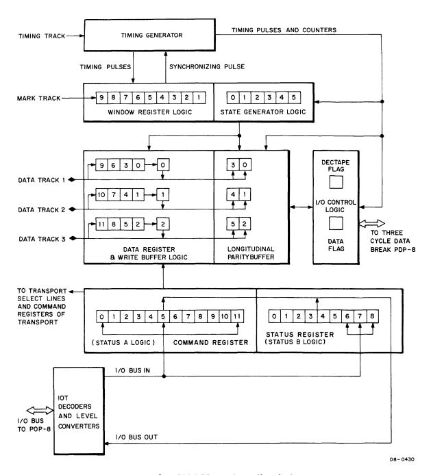
Figure 3-3 The TC08 DECtape Controller Block Diagram
