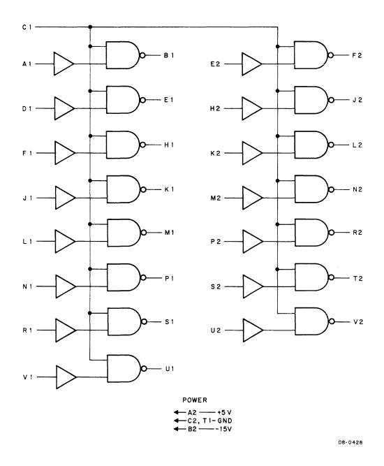
Figure 6-8 The M100 Bus Data Interface Module, Logic Diagram
