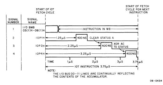
Figure 3–5B Command Register Timing with PDP-8
