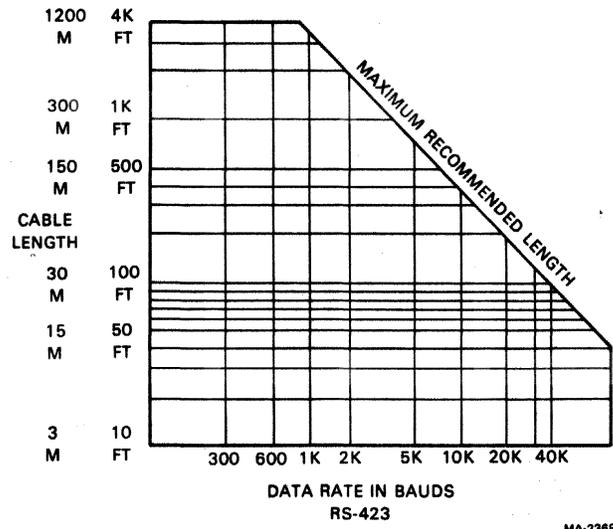
Figure 4-19 Data Rate and Cable Length for RS-423
