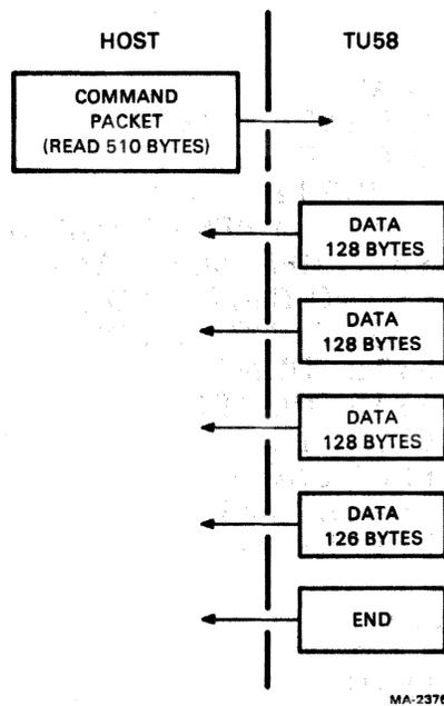
Figure 3-1 Read Command Packet Exchange
