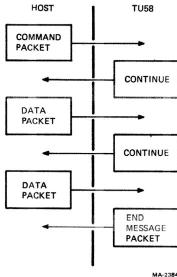
Figure 1-2 An Exchange in Radial Serial Protocol
