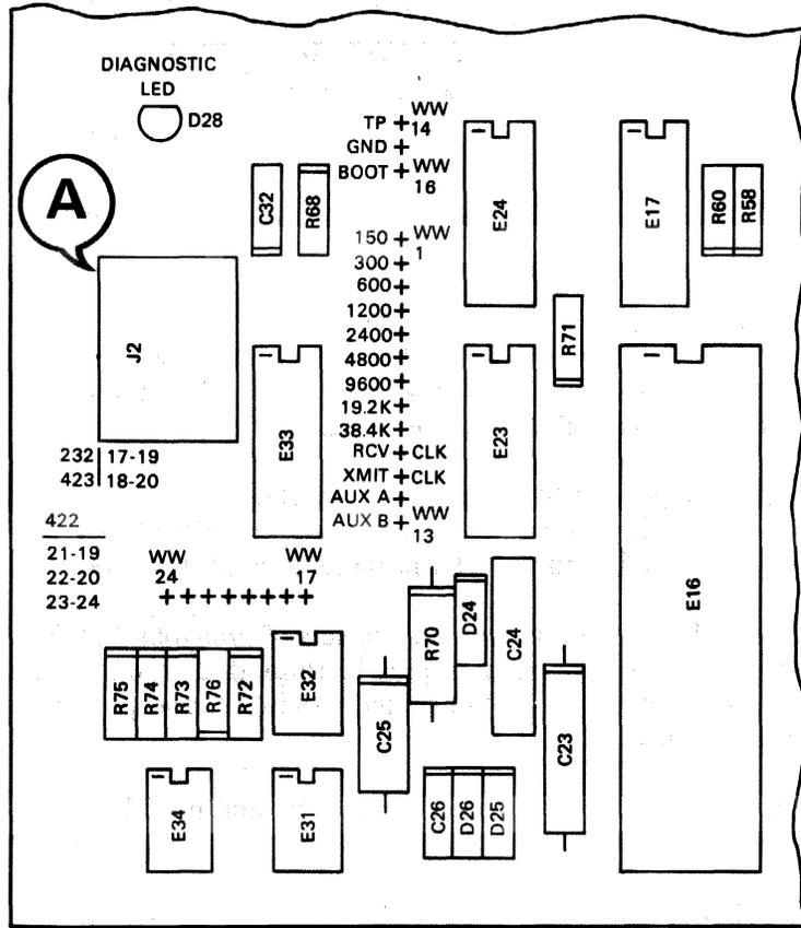
Figure 4-20 Interface Selection Jumper Pin Locations
