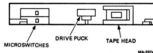
Figure 2-5 View Into Tape Drive Cartridge Slot
