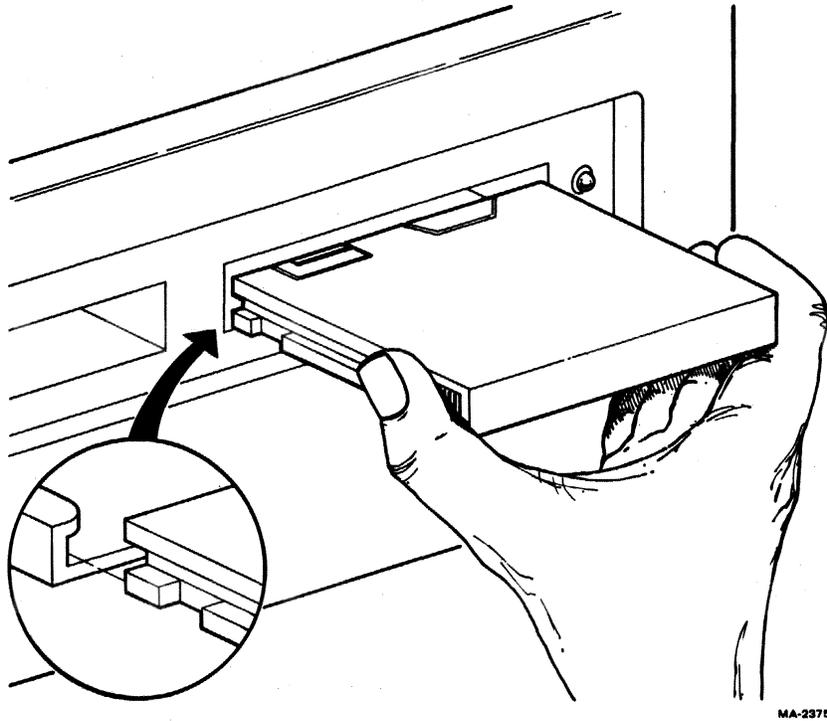
Figure 2-3 Cartridge Loading
