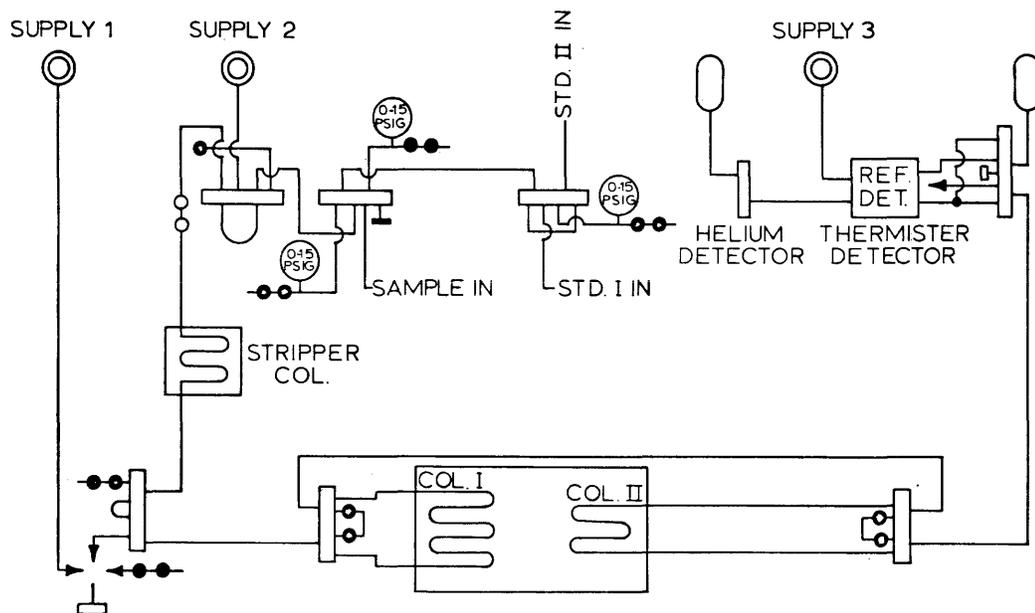
Figure 6 Schematic of the Fully-Automated Three-Column Gas Chromatograph
