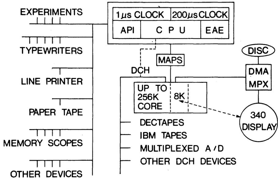
Fig. 1 Typical large PDP-9T configuration, showing the variety of peripheral devices that may be attached to the system.
