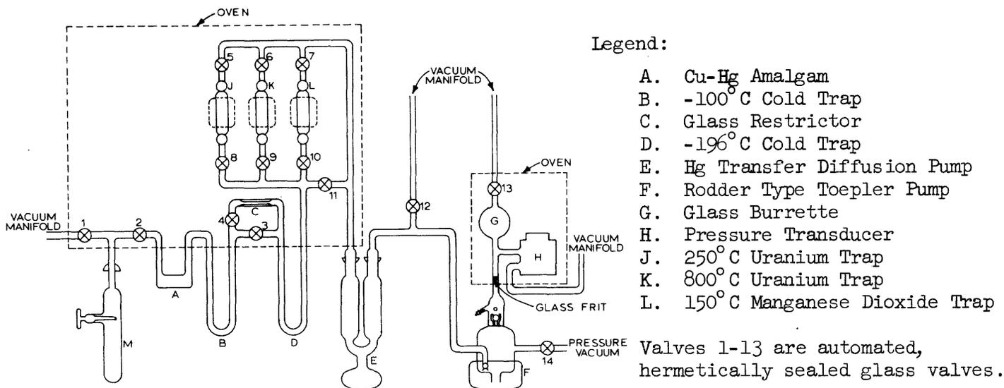
Figure 5 Schematic of the Apparatus for the Simultaneous Determination of Carbon, Hydrogen and Nitrogen in Organic Compounds
