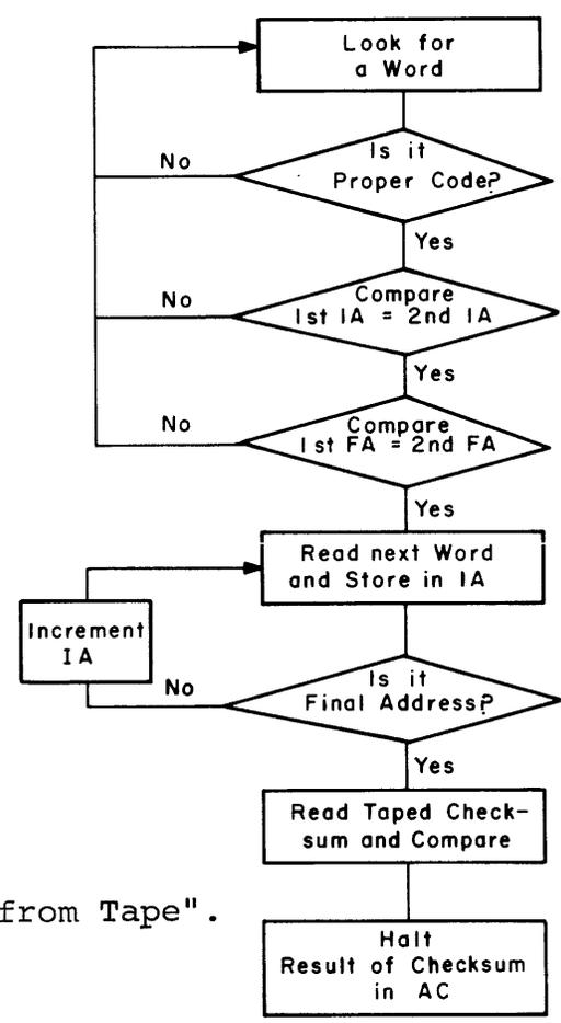
Fig. 6 Flow chart of "Read from Tape".
