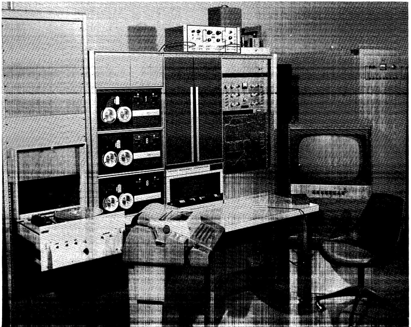
Figure 4 Picture showing system configuration. From left to right is the stepping recorder, teletype, DEctape units, PDP-8 computer, light pen, function box, and 21" oscilloscope.
