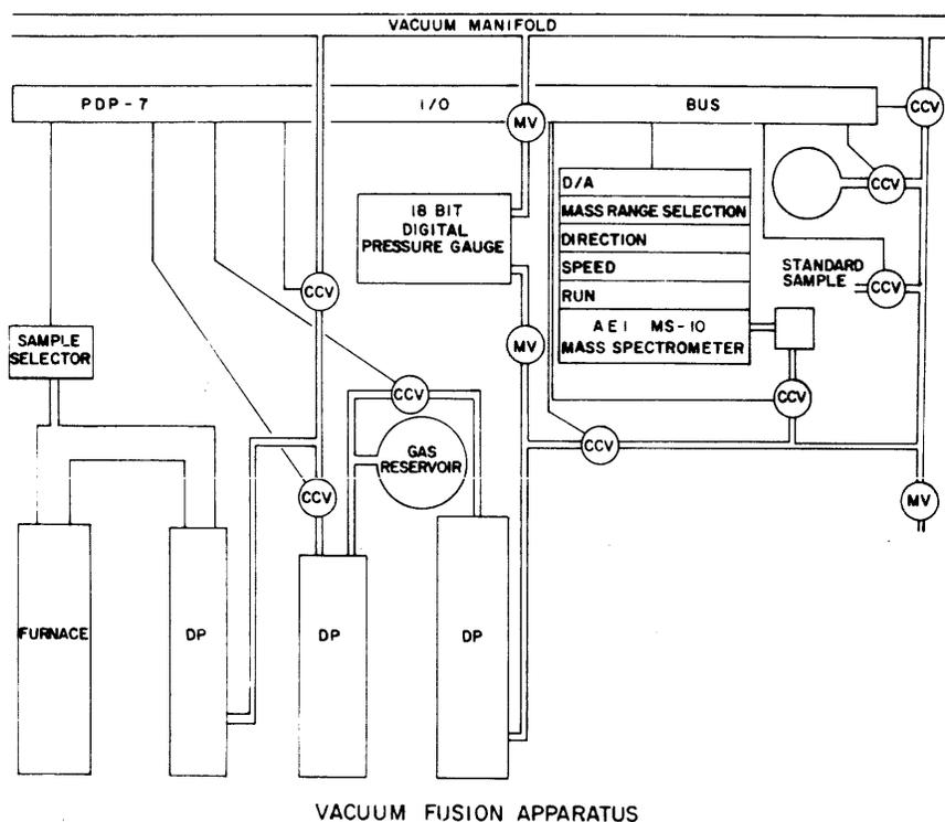
Figure 8 Schematic of Vacuum Fusion Apparatus
