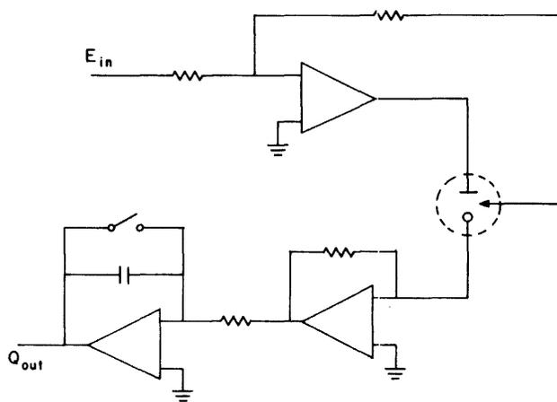
**Figure 2** Analog electrochemical potentiostatic control circuit. Operational amplifiers are all analog devices type 201.
