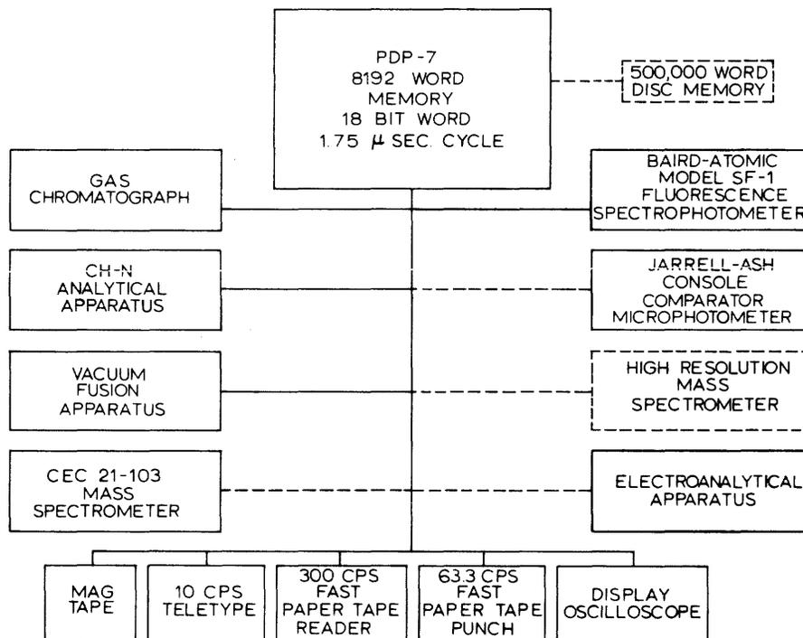
Figure 1 PDP-7 and Instrumentation System
