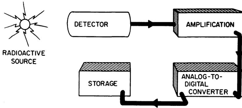
Figure 1. Experimental arrangement for a scintillation spectrometer.
