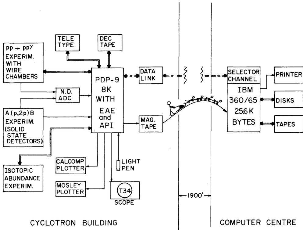
Fig.1 Manitoba Cyclotron computer system. The dashed line indicates that the fast data link is not yet operational.
