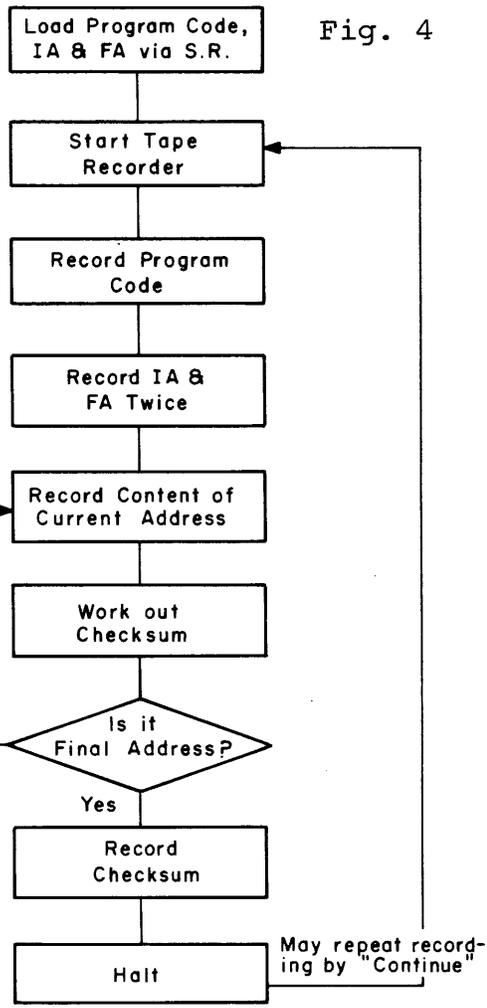
Fig. 4 Flow chart of "Record on Tape".
