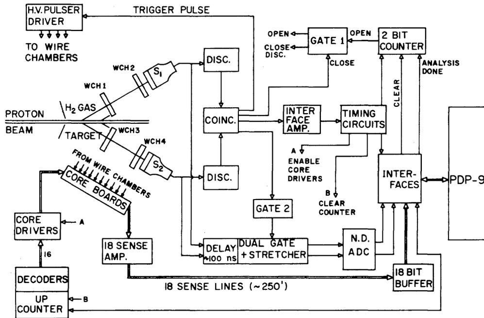
Fig.2 Proton-proton bremsstrahlung equipment and interfaces.
