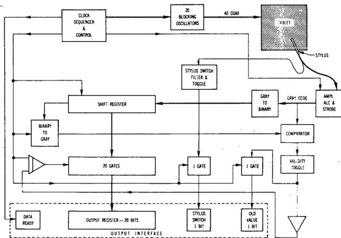
The pulses are encoded by the tables as serial x, y Gray-code position information which is sensed by the high-input impedance, pen-like stylus from the epoxy-coated tablet surface. This information is strobed from Gray to binary code, assembled in a shift register, and gated in parallel to an interface register.
