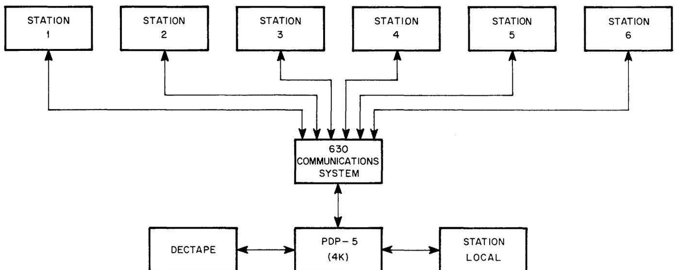
A special time-shared programming system has been developed providing each control area with immediate access to the central processor computer, and allowing ease of interpretation of data by computer users.
