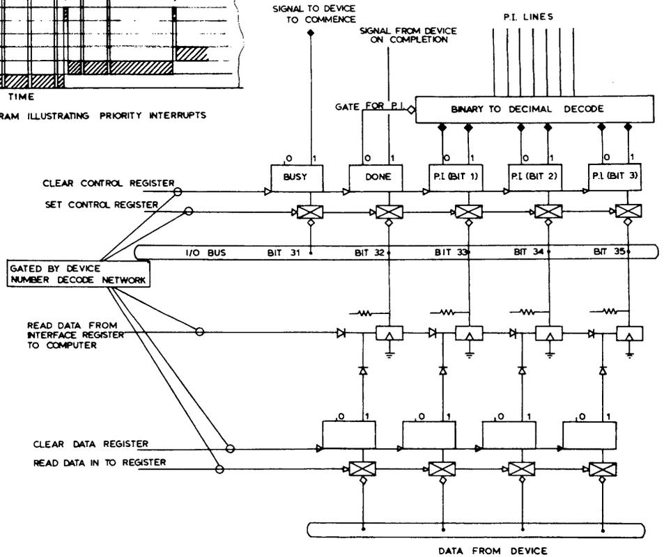
FIGURE 2: SIMPLIFIED LOGIC DIAGRAM SHOWING TYPICAL ARRANGEMENTS OF CONTROL AND DATA REGISTERS
