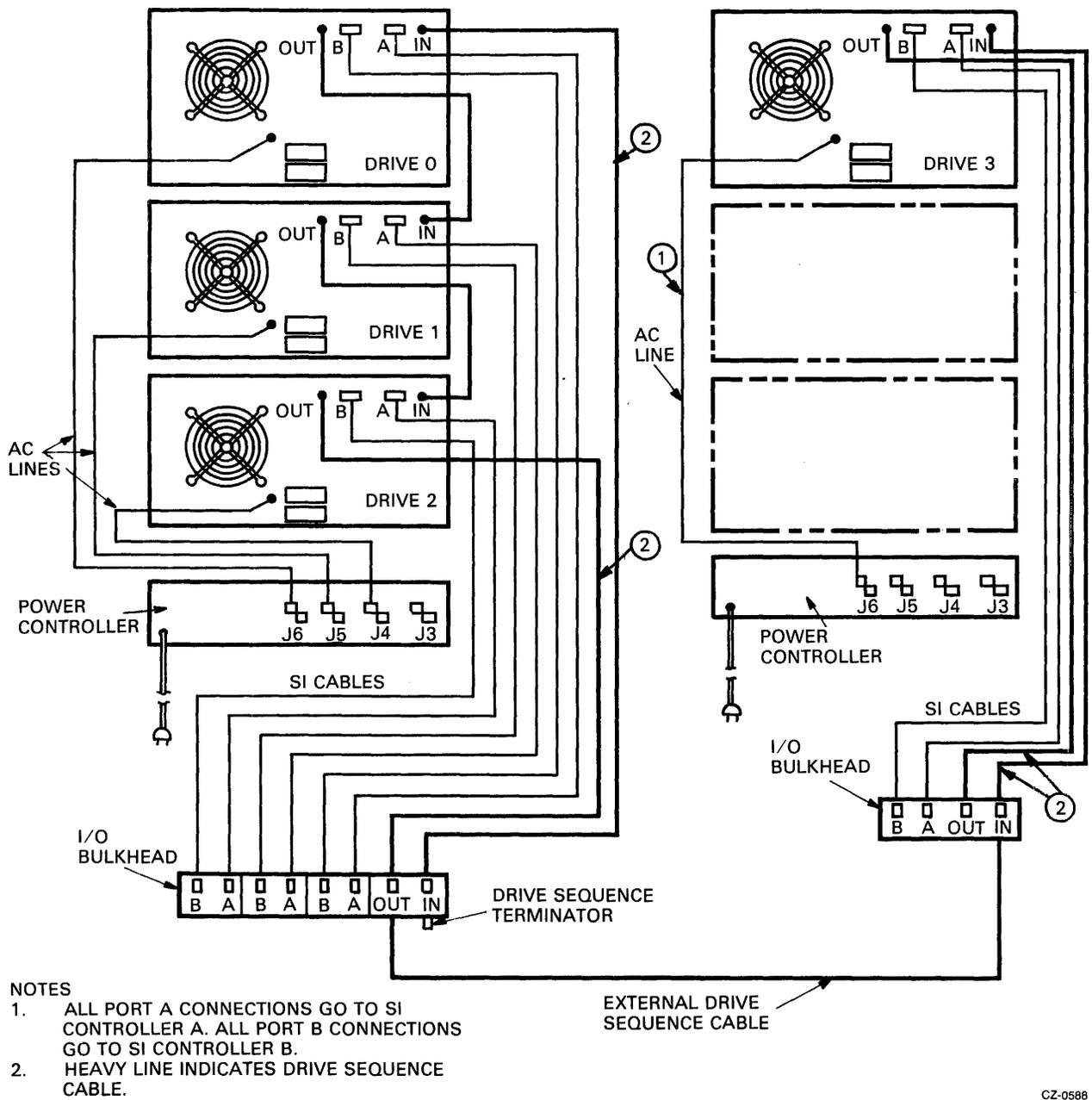
Figure 2-35 Cabling for the Three- and Four-Drive System
