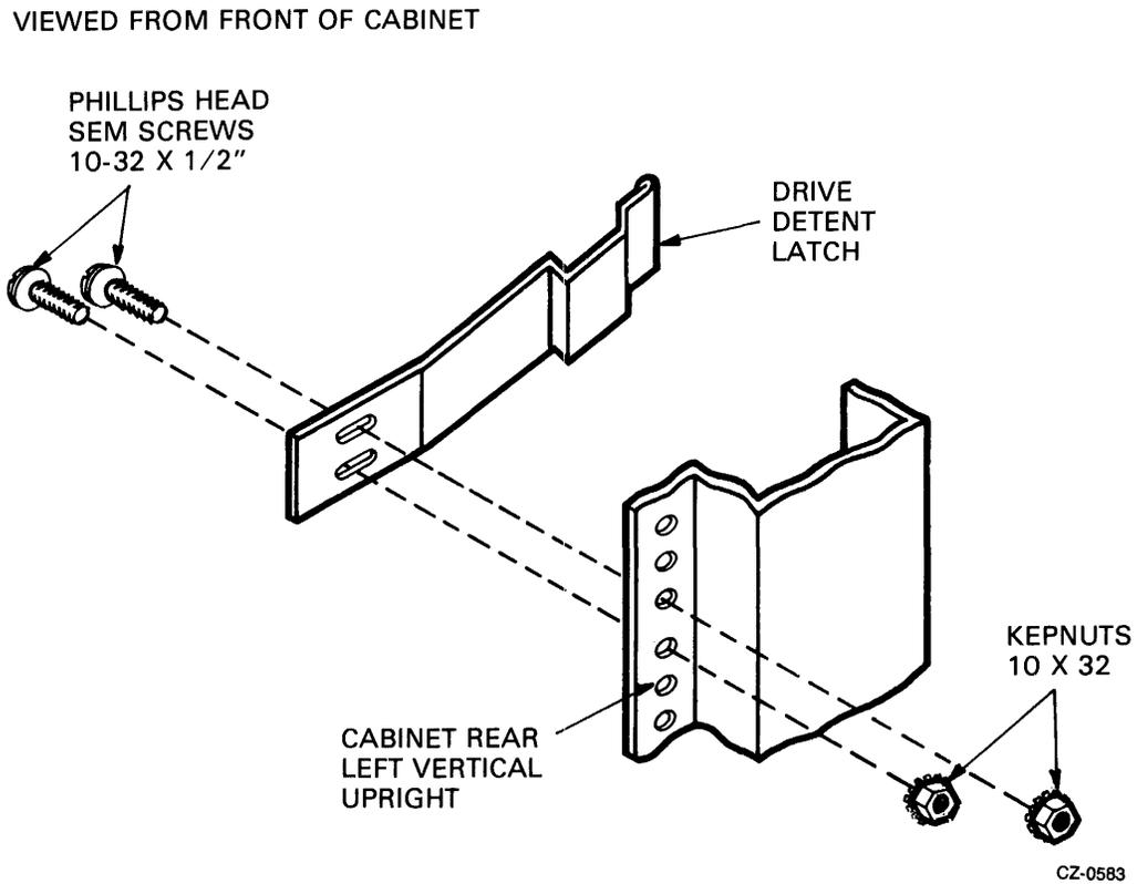
Figure 2-27 Installation of Drive Detent Latch
