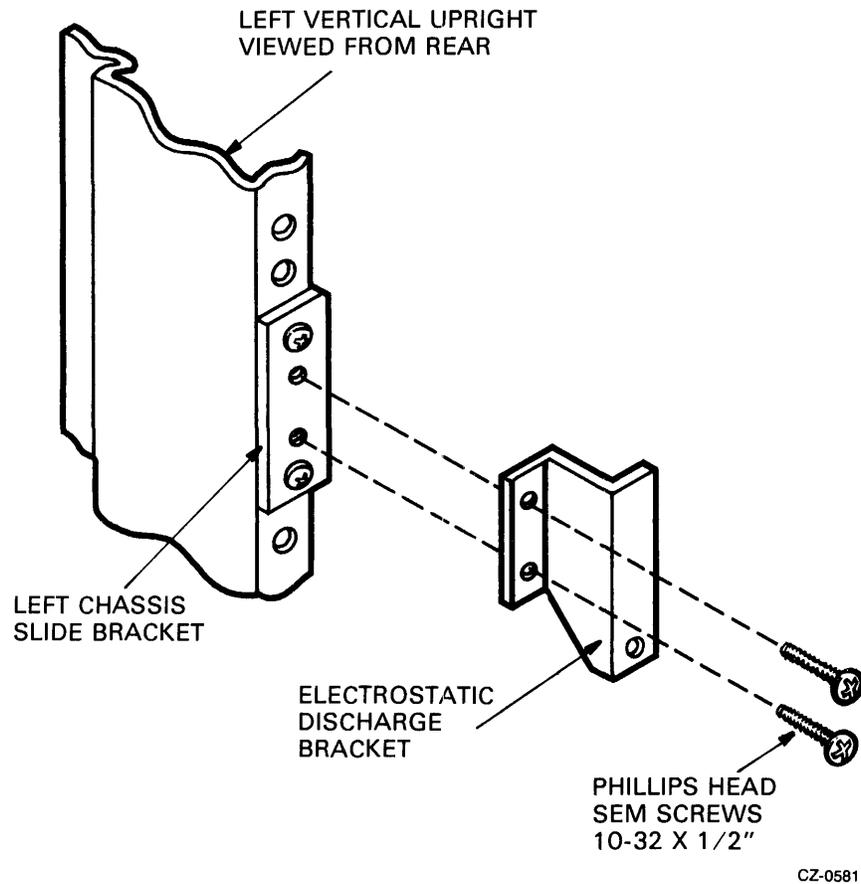
Figure 2-25 Mounting the Electrostatic Discharge Bracket
