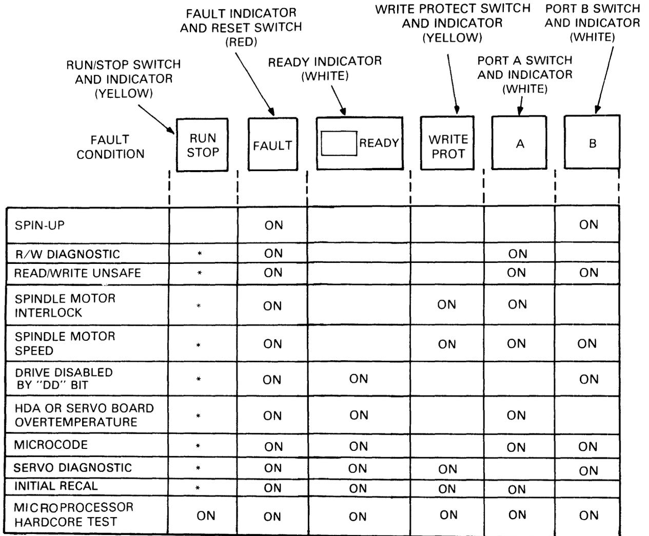
\*THE INDICATOR STATE WILL BE THE SAME AS IT WAS BEFORE THE FAULT SWITCH WAS PUSHED
