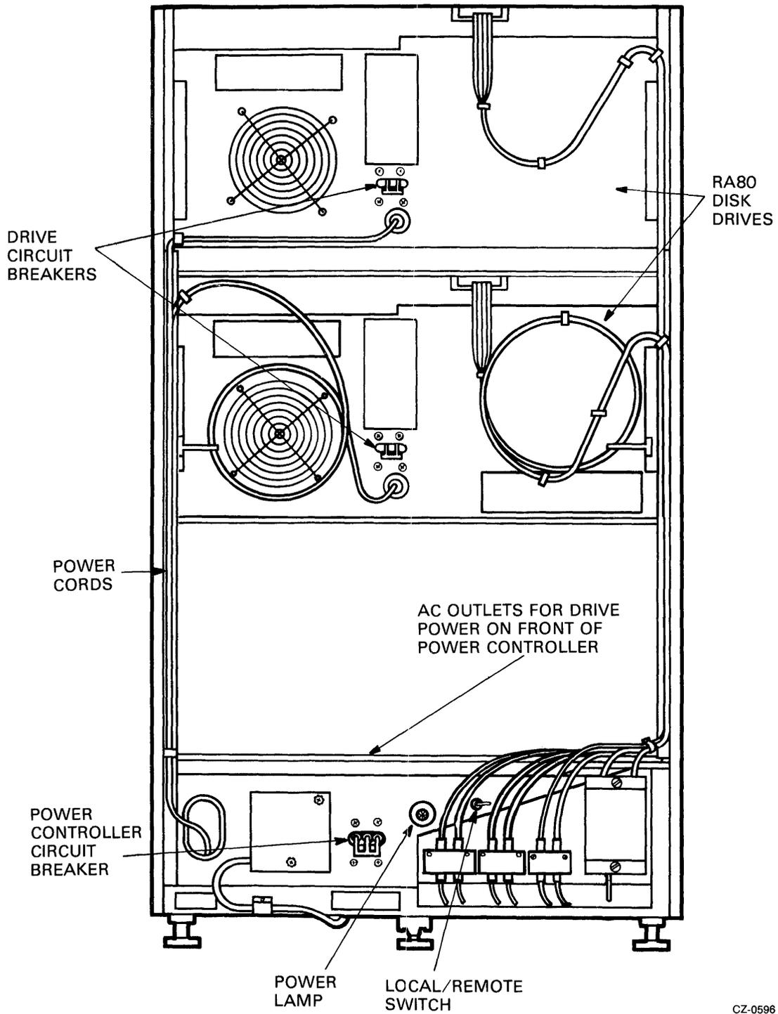
Figure 3-2 Circuit Breakers
