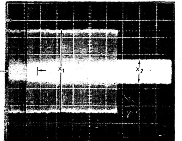
d. Head correctly aligned at CYL 105. Amplitudes are equal.
