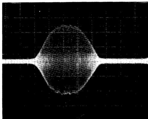
Figure 5-12 Read/Write Head Alignment Waveforms
