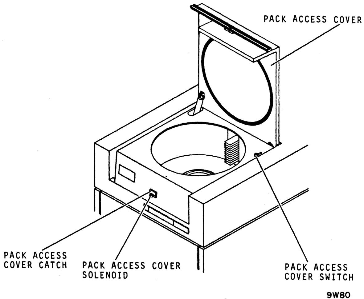
Figure 3-16. Pack Access Cover Switch and Solenoid
