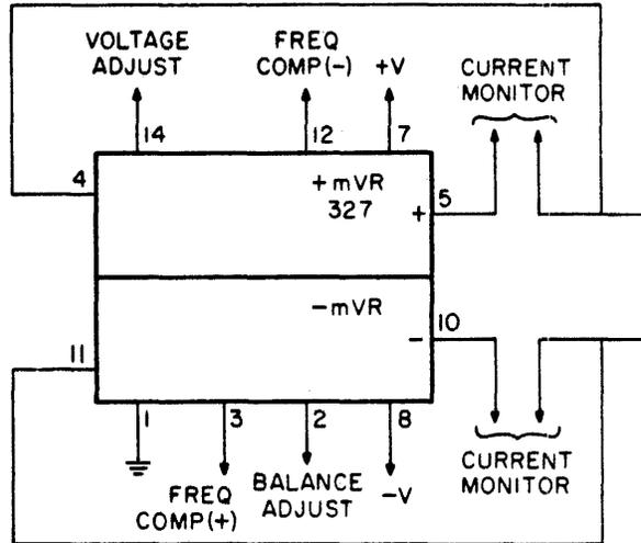
REPLACE m WITH NOMINAL VOLTAGE AS DETERMINED BY VOLTAGE AND BALANCE ADJUST COMPONENTS.
