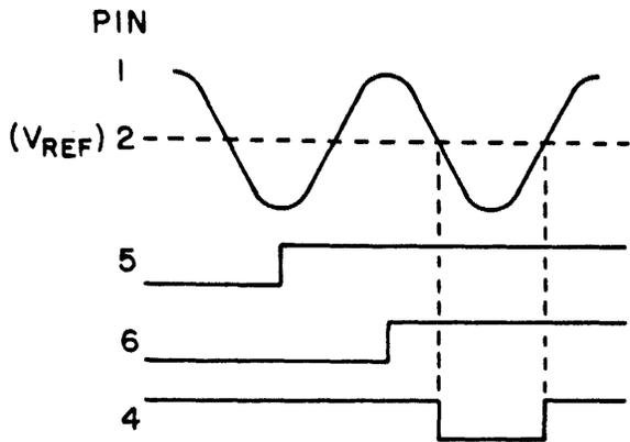
PIN 4 IS LOW ONLY IF G1 AND G2 ARE HIGH AND PIN 1 IS MORE NEGATIVE THAN PIN 2. G2 IS COMMON TO BOTH CONVERTERS.
