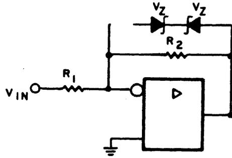
$$V_{OUT} = - \frac{R_2}{R_1} V_{IN}$$
