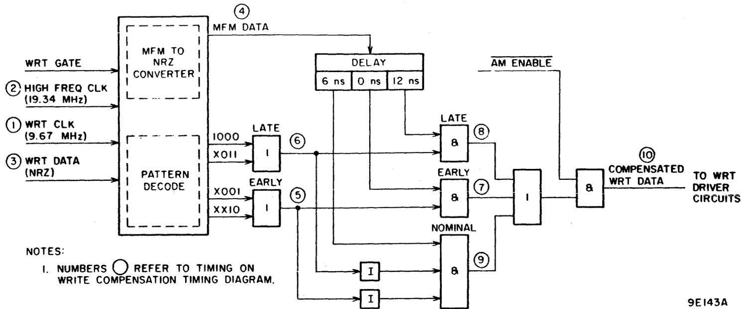
Figure 3-72. Write Compensation/NRZ to MFM Converter Circuits
