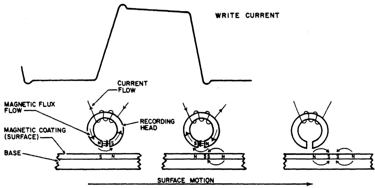
NOTE: RELATIVE HEAD TO SURFACE MOTION, RECORDING (WRITE OPERATION)
