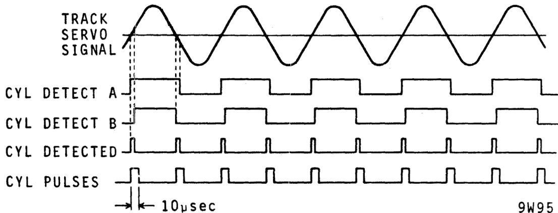
Figure 3-36. Cylinder Crossing Detection
