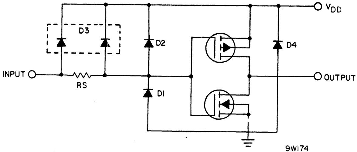
Figure 4-13. Diode-Resistor Input Protection
