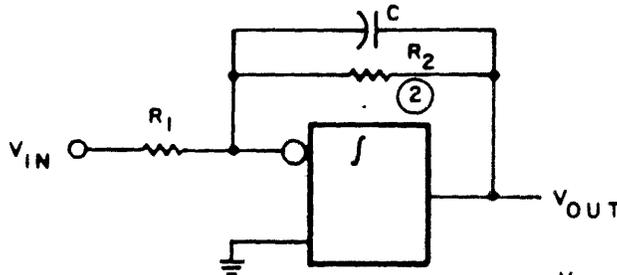
$$V_{OUT} = - \frac{1}{R_1 C} \int V_{IN} dt$$
