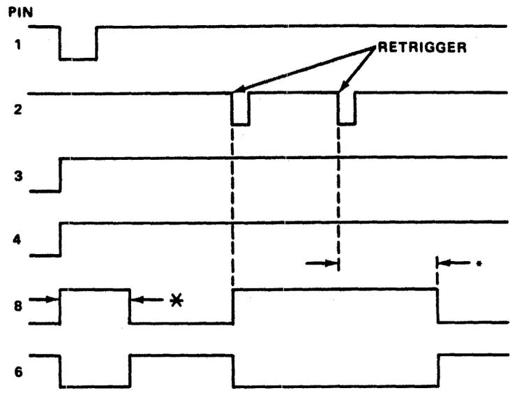
\* PULSE WIDTH DETERMINED BY RC TIMING NETWORK
