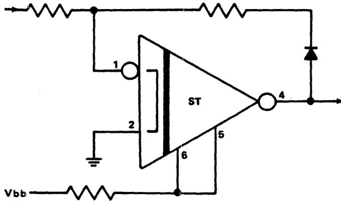
162 DUAL DIFFERENTIAL RECEIVER USED AS A SCHMITT TRIGGER WITH EXTERNAL FEEDBACK NETWORKS AND FIXED BIAS ENABLING G1 AND G2 STROBE INPUTS'
