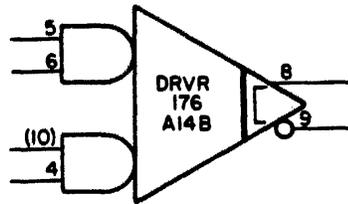
The pin number in parentheses (10) denotes a pin that is common to other section(s) of the microcircuit. In this case, the symbol for the "A" section of the driver would show pin 10 without the parentheses.
