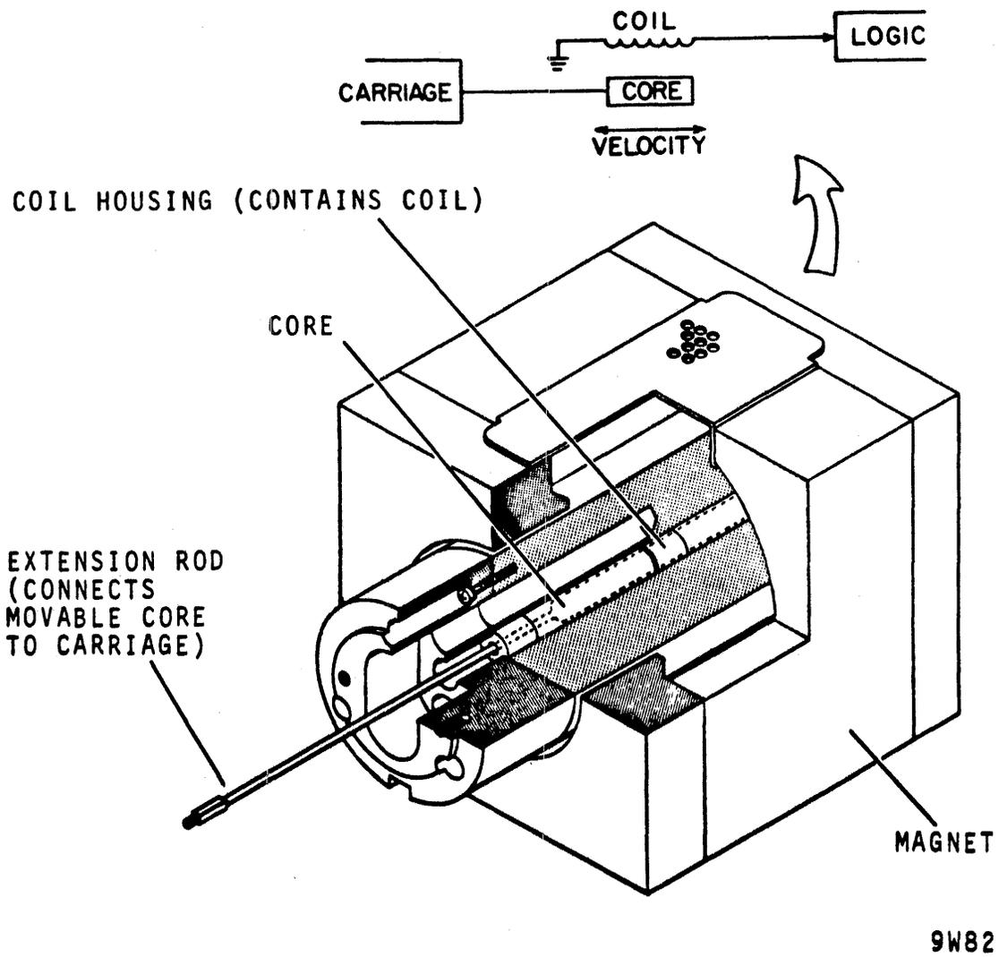
Figure 3-19. Velocity Transducer Assembly
