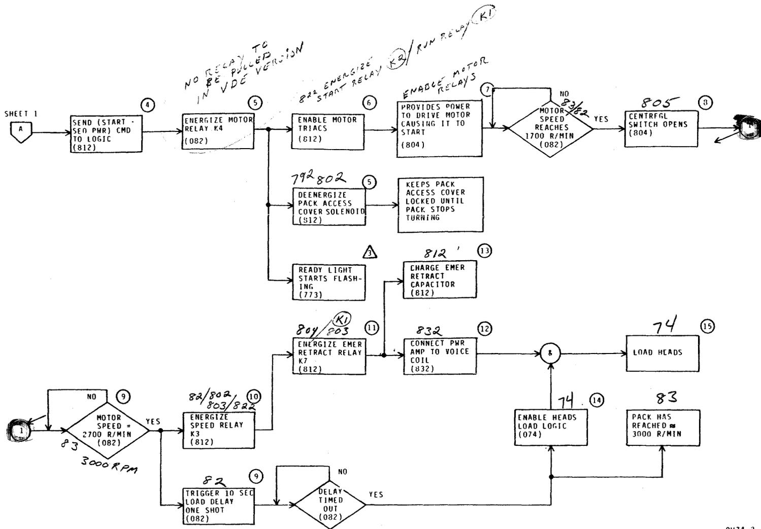
Figure 3-6. Power On Sequence Flow Chart (Sheet 2)
