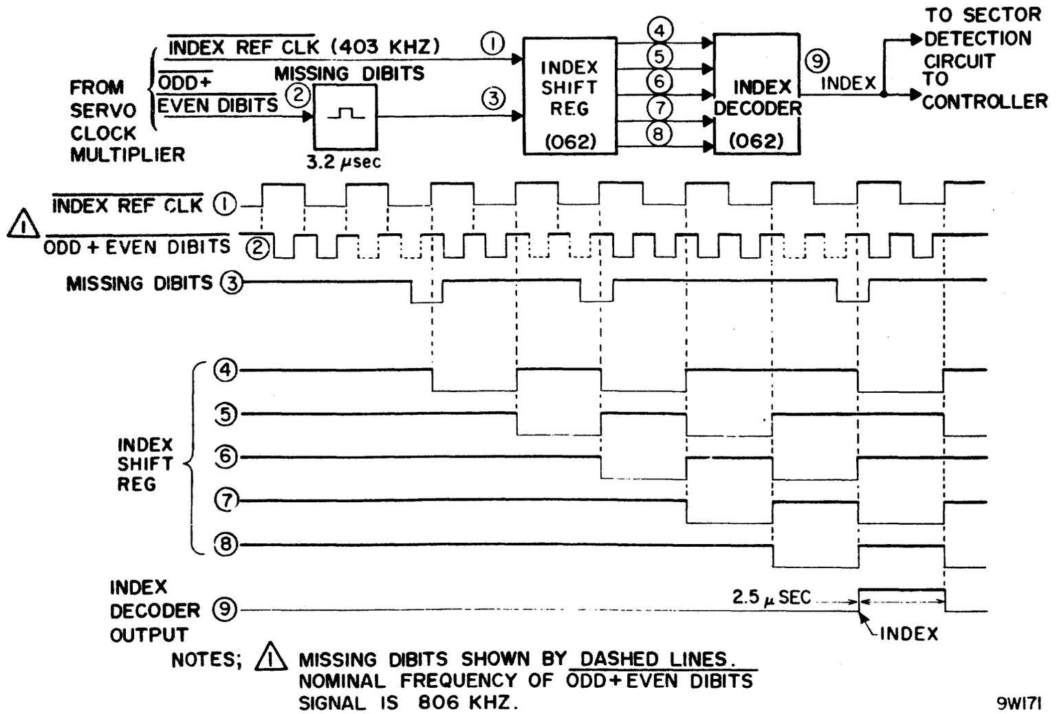
Figure 3-54. Index Detection - Logic and Timing
