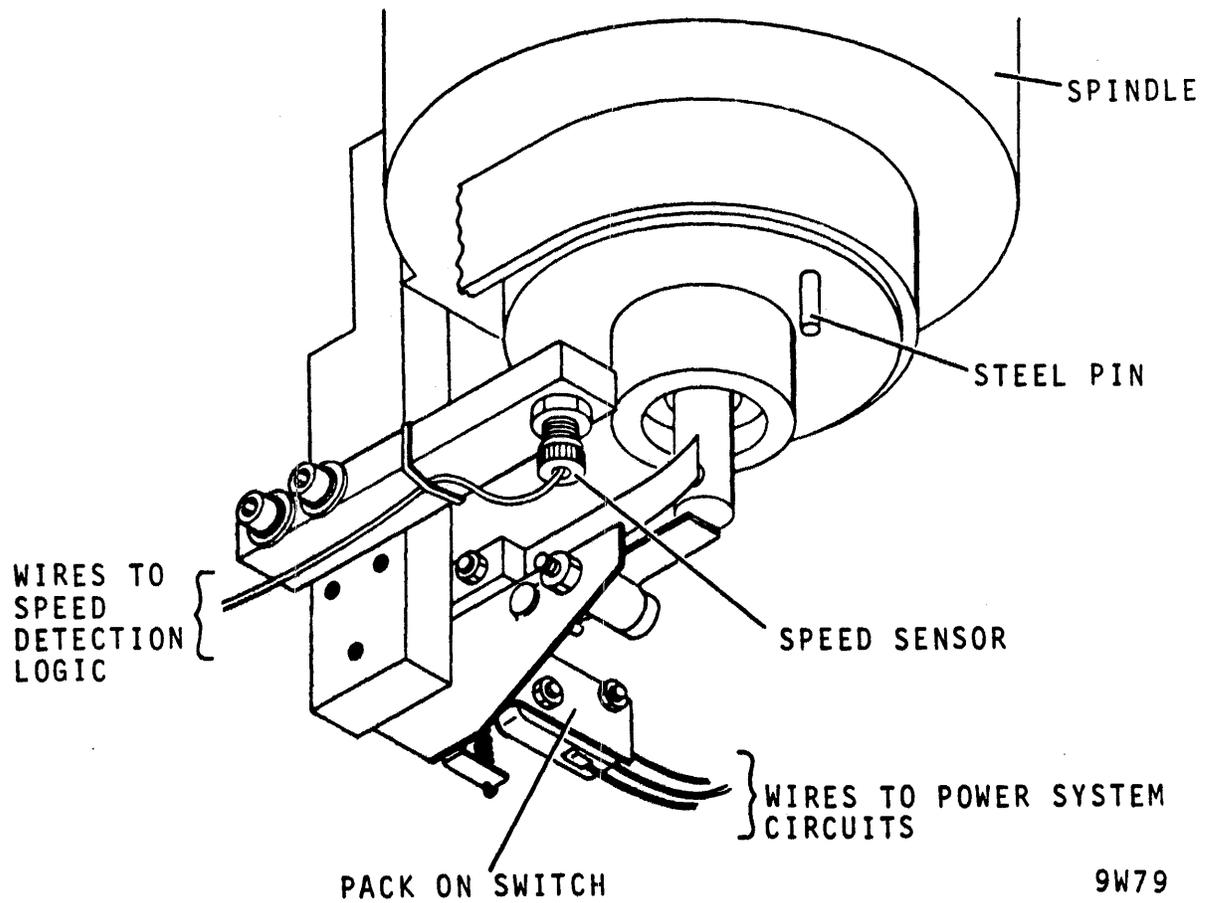
Figure 3-15. Speed Sensor and Park On Switch Assemblies
