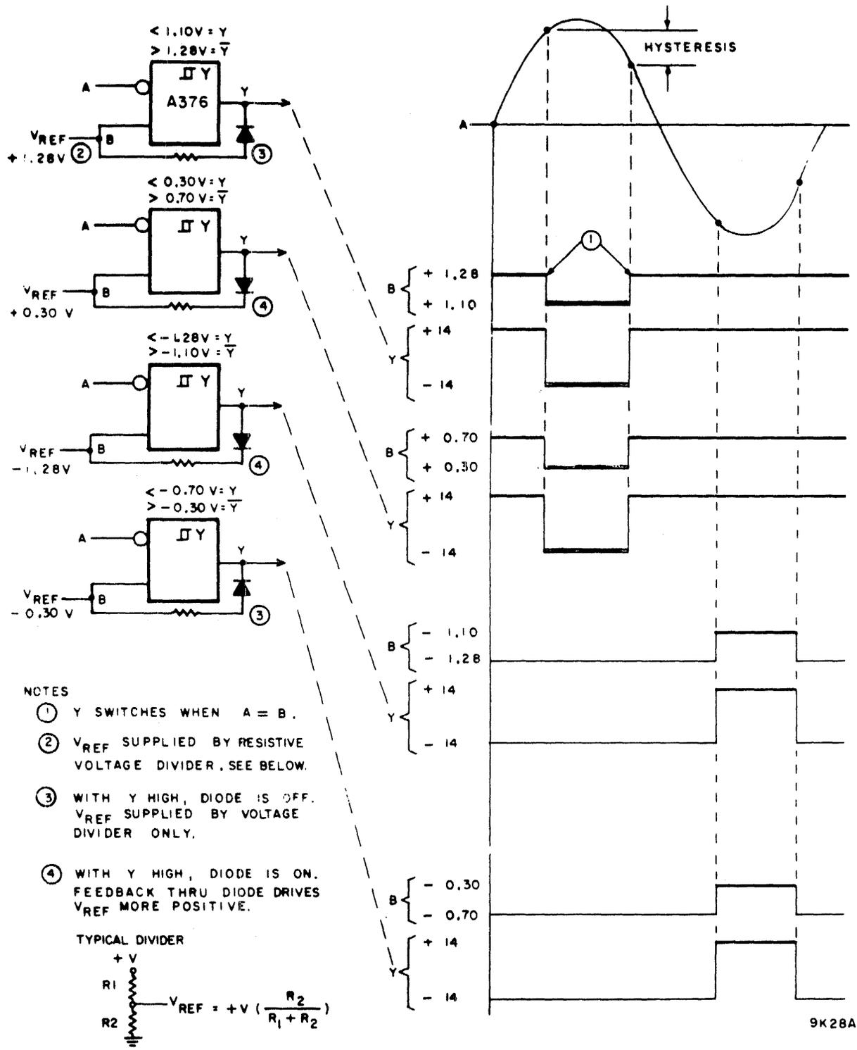
Figure 4-20. Op Amp Used as Schmitt Trigger
