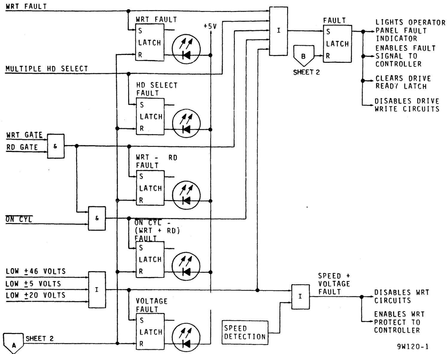
Figure 3-75. Fault and Error Detection Logic (Sheet 1 of 2)
