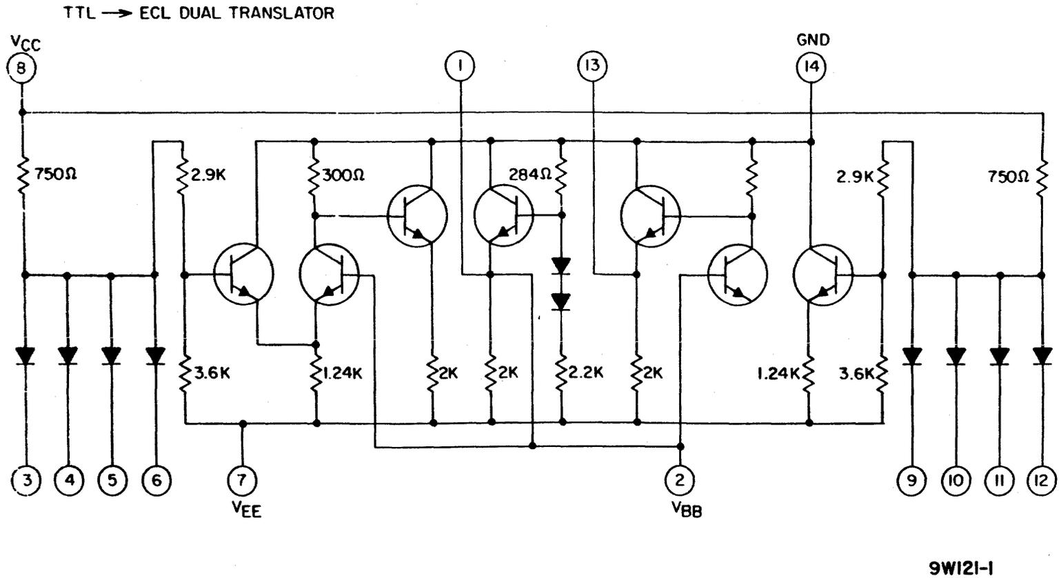
Figure 4-7. TTL/ECL Interface (Sheet 1 of 2)
