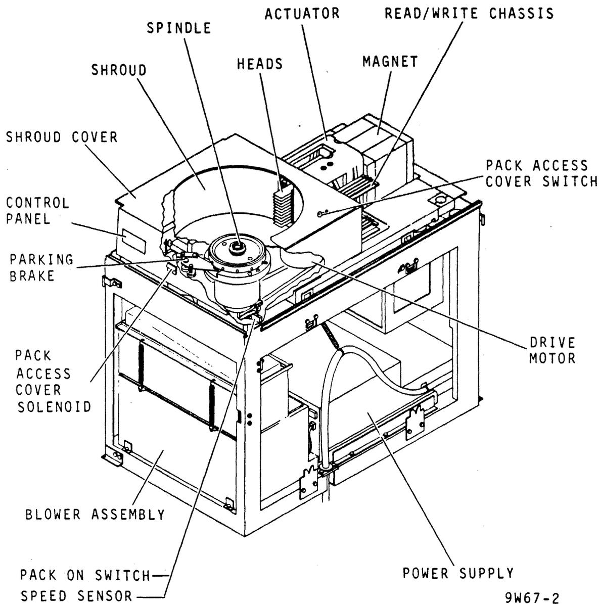
Figure 1-2. Drive Assemblies (Sheet 2 of 2)
