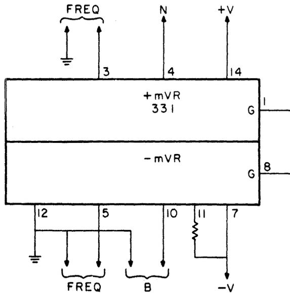
REPLACE m WITH NOMINAL VOLTAGE AS DETERMINED BY BIAS (B) AND BALANCE (N) COMPONENTS
