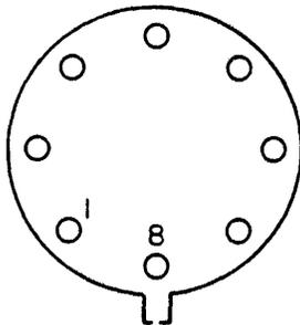
PIN 4 CONNECTED TO CASE
