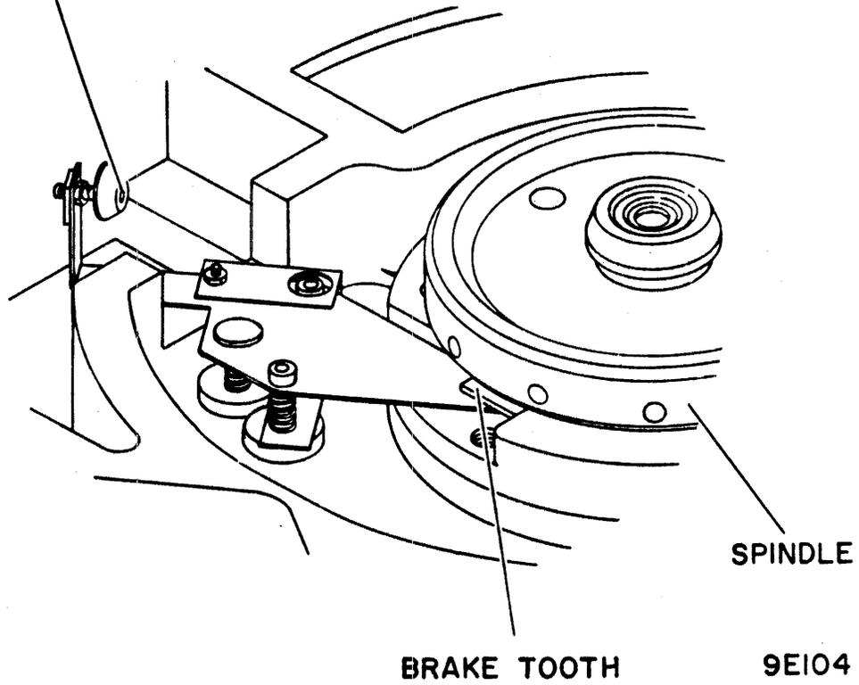
Figure 3-14. Parking Brake Assembly
