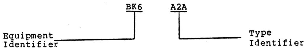
The equipment identifier indicates the basic functional capabilities of the drive. This number will be either BK6 or BK7. The differences between these units can be determined by referring to table 1-1.
