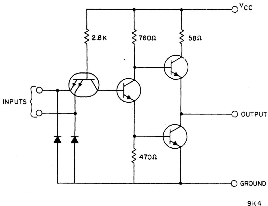
Figure 4-4. TTL NAND Circuit, High-Speed Series
