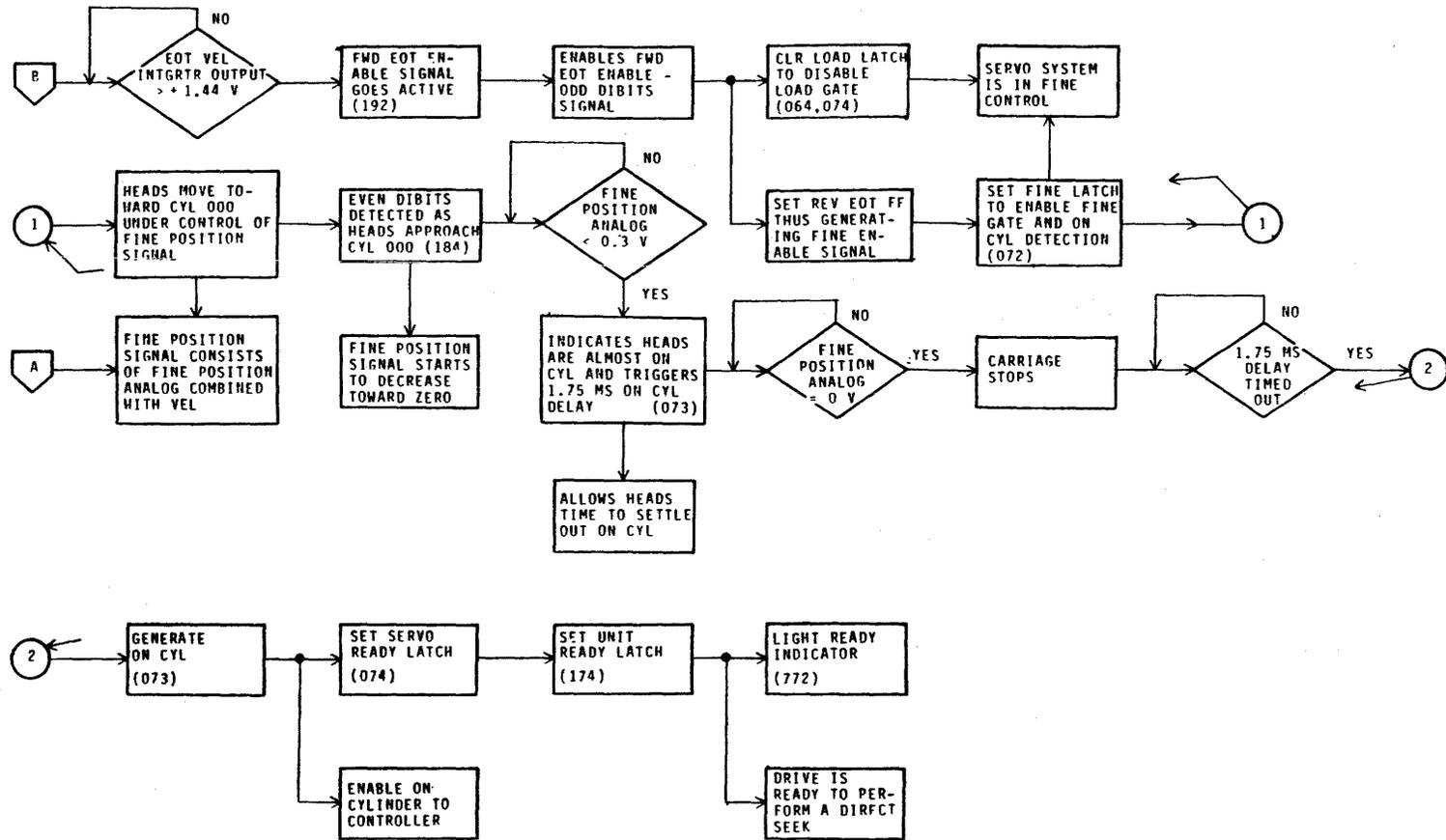
Figure 3-46. Load Sequence Flow Chart (Sheet 2)
