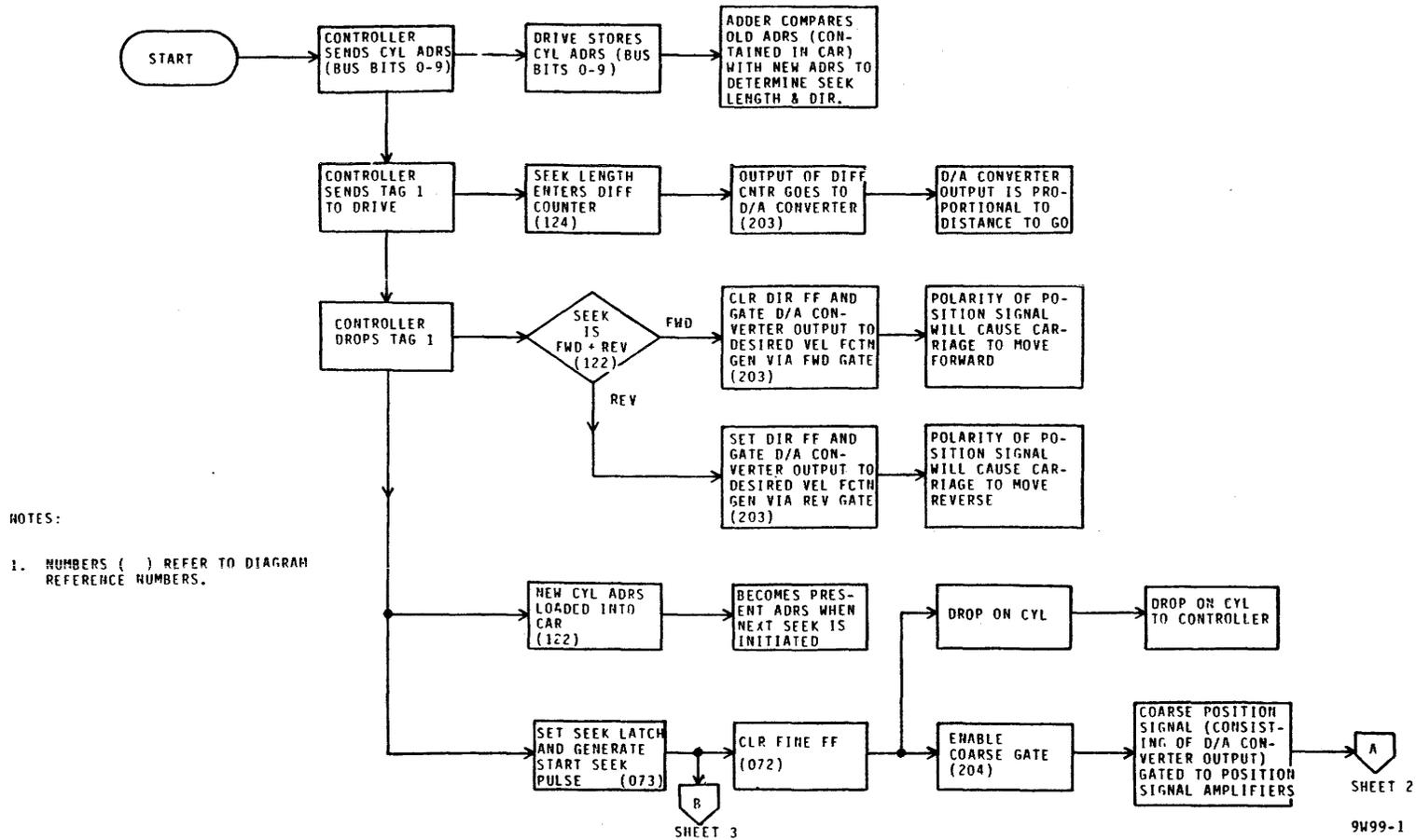
Figure 3-40. Direct Seek Flow Chart (Sheet 1 of 3)
