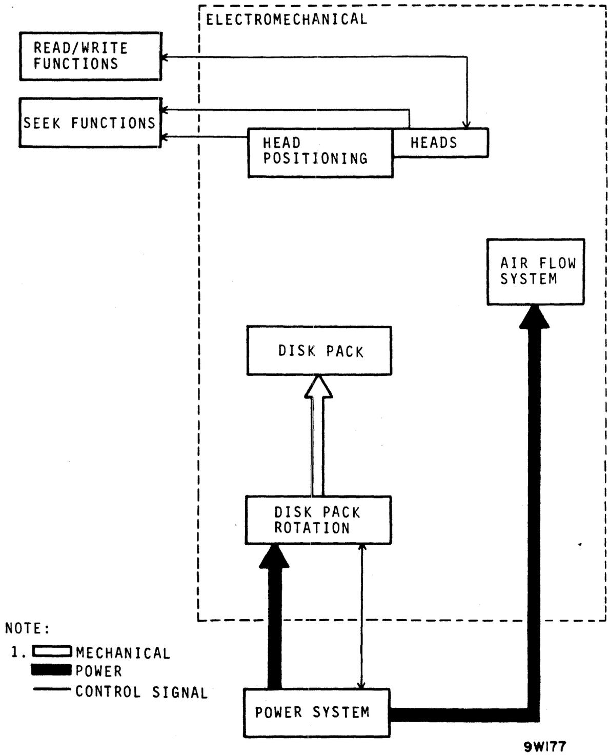
Figure 3-10. Electromechanical Functions Block Diagram
