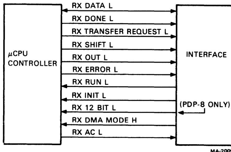
Figure 5-5 Interface to  $\mu$ CPU Controller Signals
