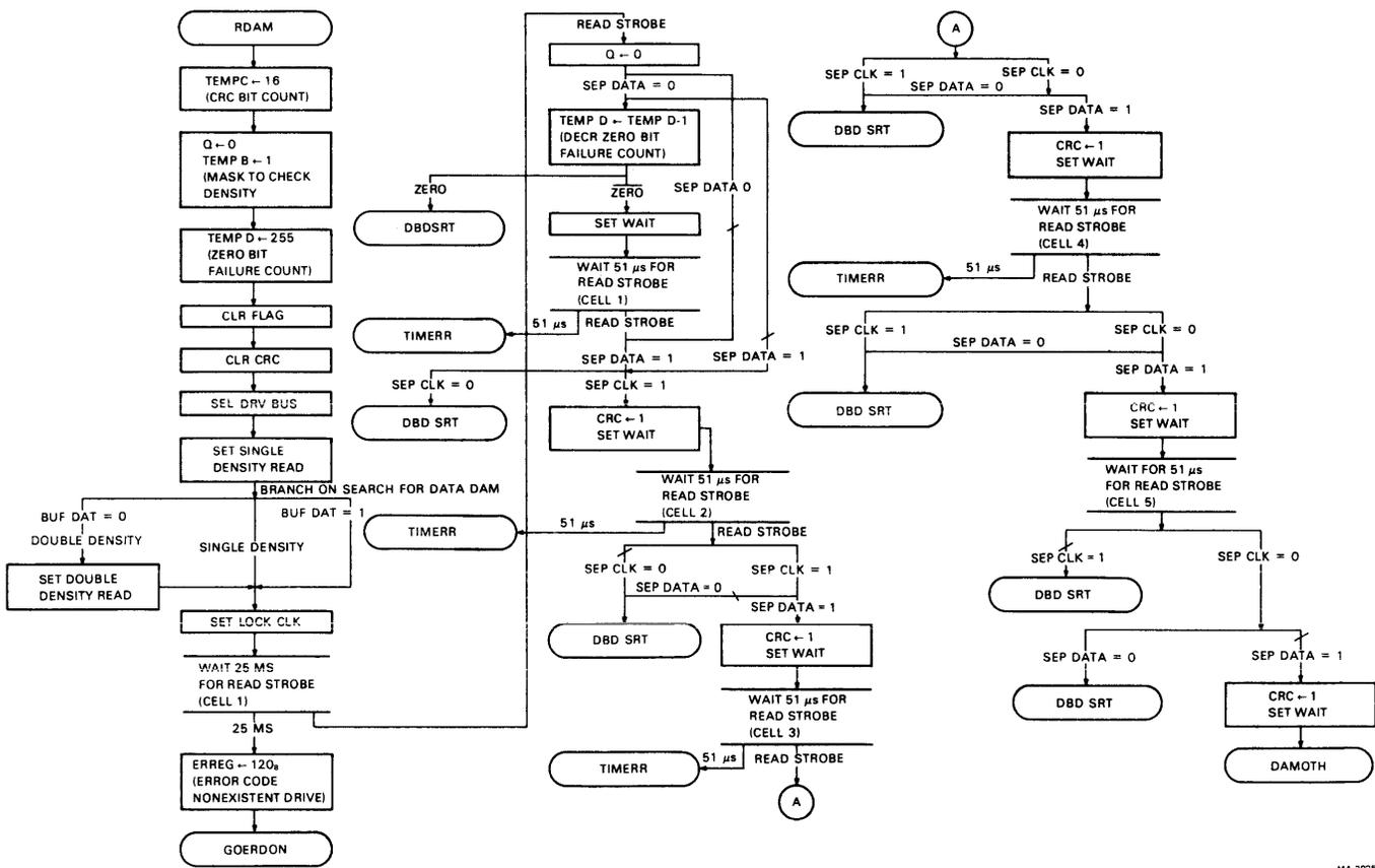
Figure 5-20 Read Address Mask Subroutine Flowchart (Sheet 1 of 3)
