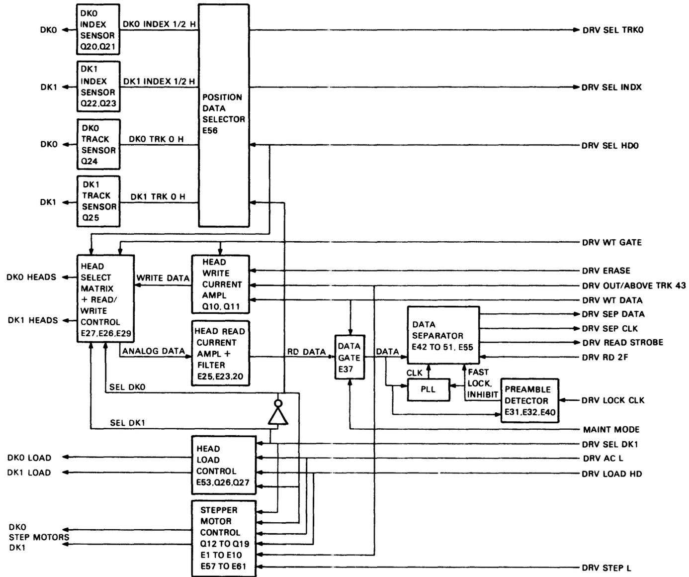
Figure 5-31 Read/Write Electronics Block Diagram
