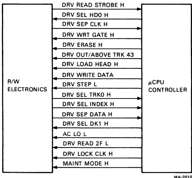
Figure 5-6  $\mu$ CPU Controller to Read/Write Electronics Signals
