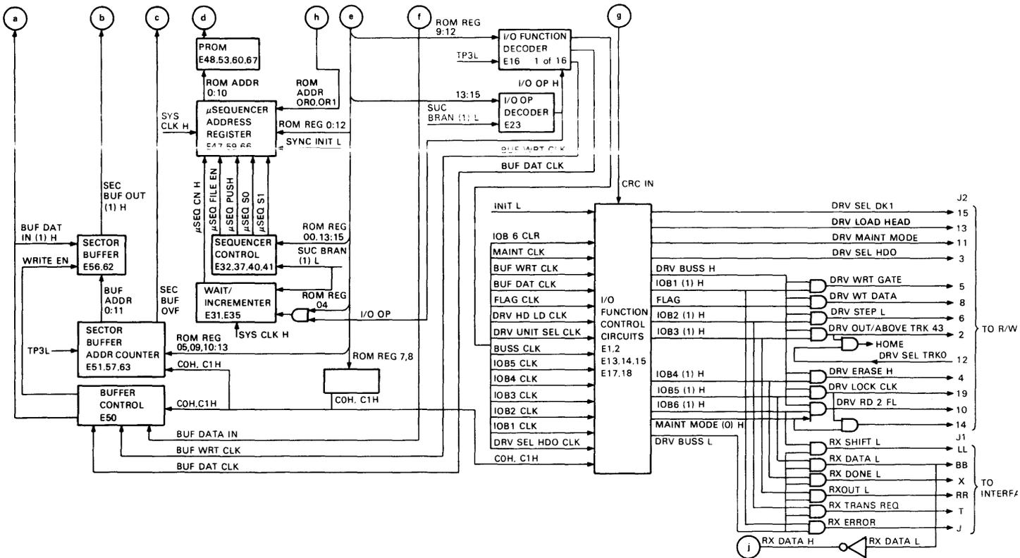
Figure 5-13 μCPU Controller Block Diagram
