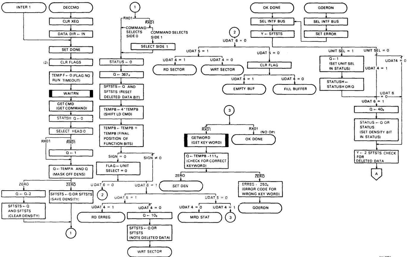
Figure 5-26 Decode Command Routine Flowchart
