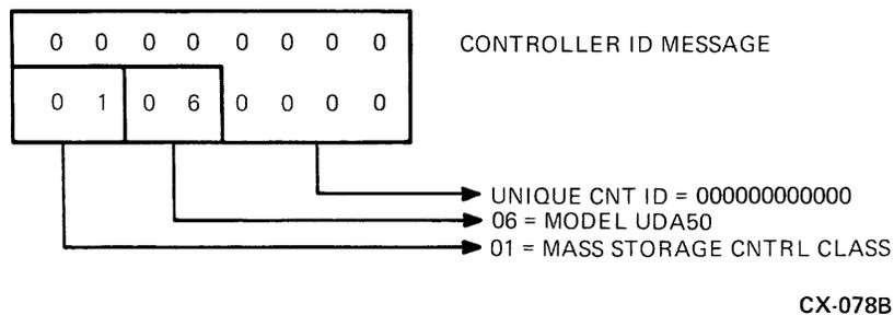
Figure 2-4 Decode of Controller Identification Message
