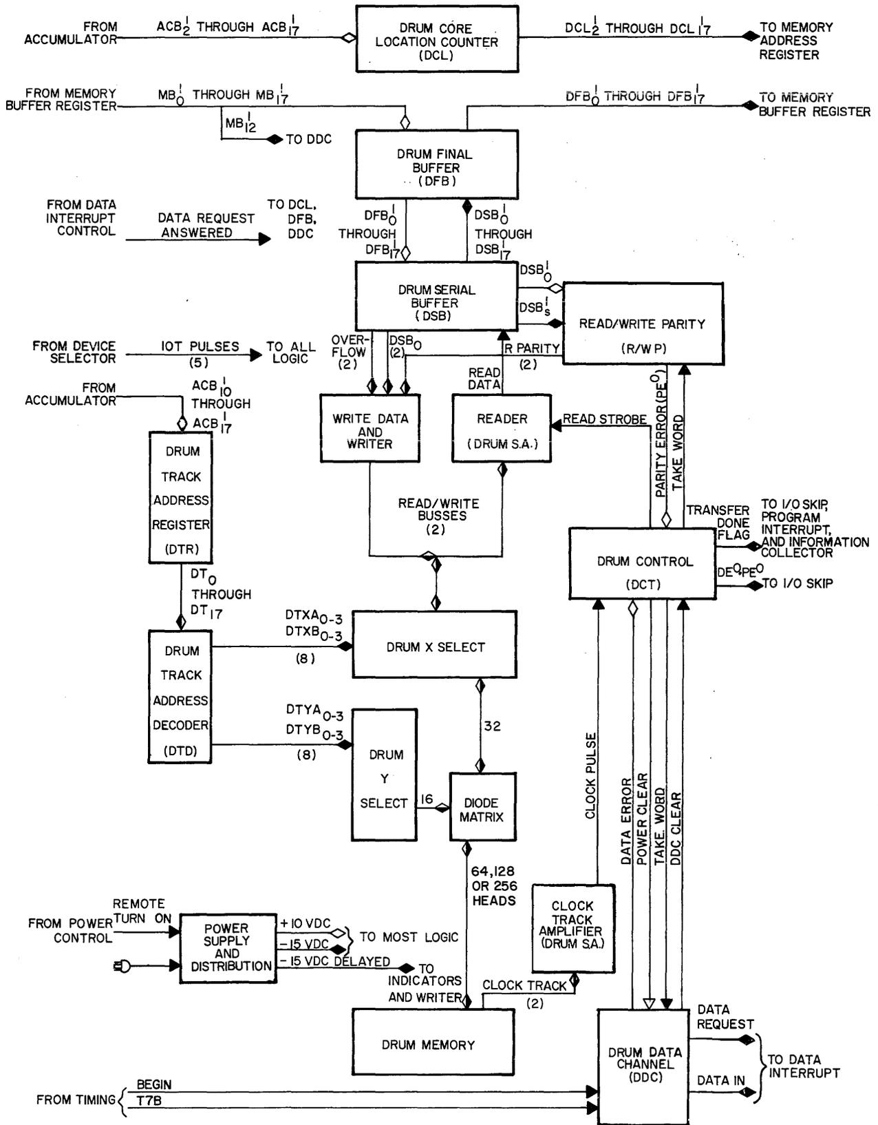
Figure 2-2 Type 24 Serial Drum Block Diagram
