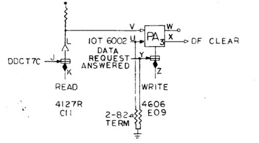
Drum Track Address Register & Decoding (X&Y)
