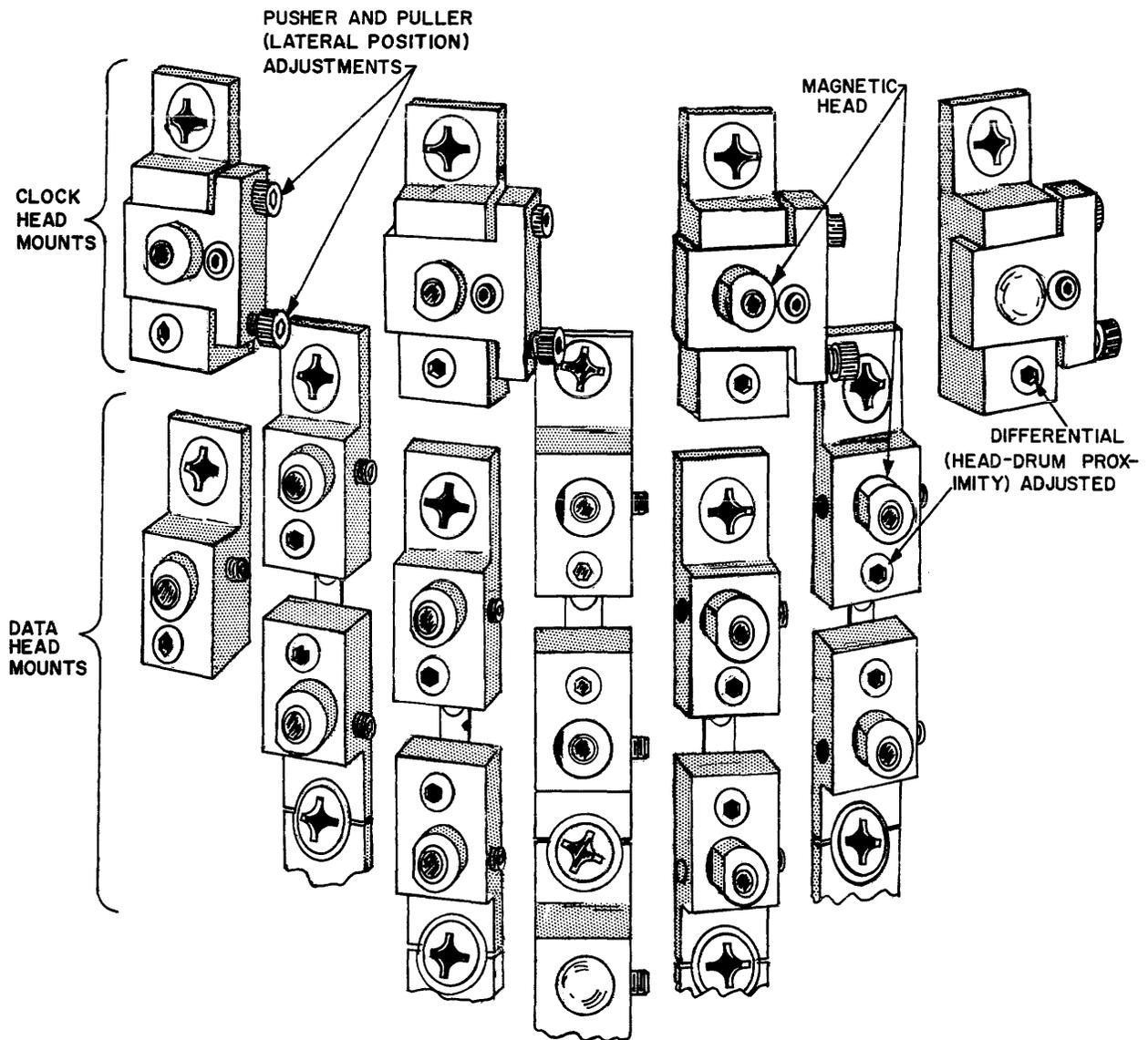
Figure 2-4 Drum Head Configuration
