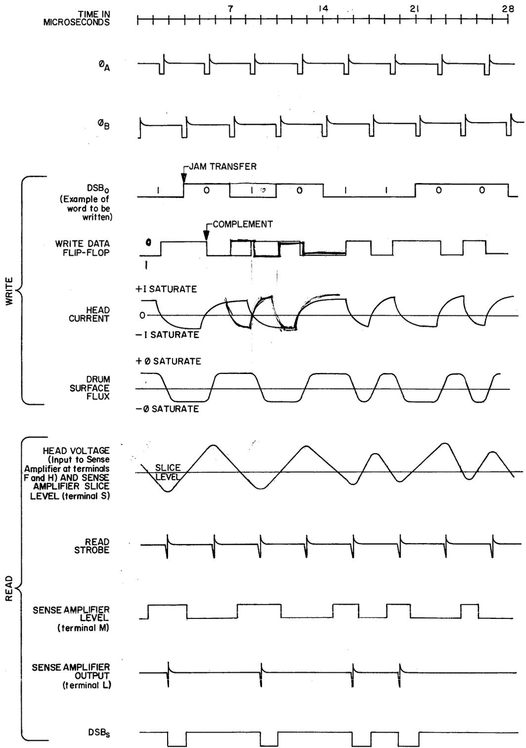
Figure 2-1 Typical Recording and Playback Timing
