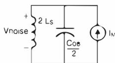
Figure 3 Parasitic Inductance of the Power Switching Stage
