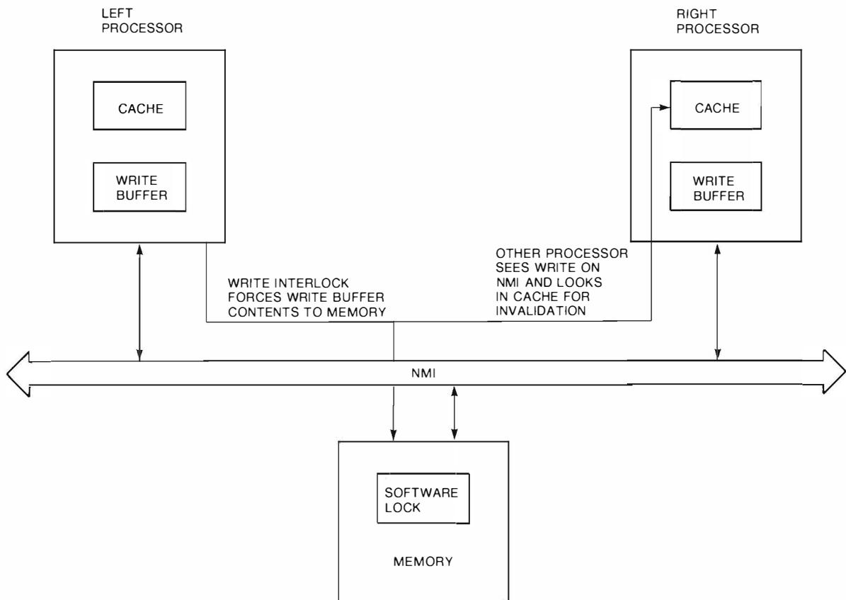
Figure 6 Multiprocessor Coherency
