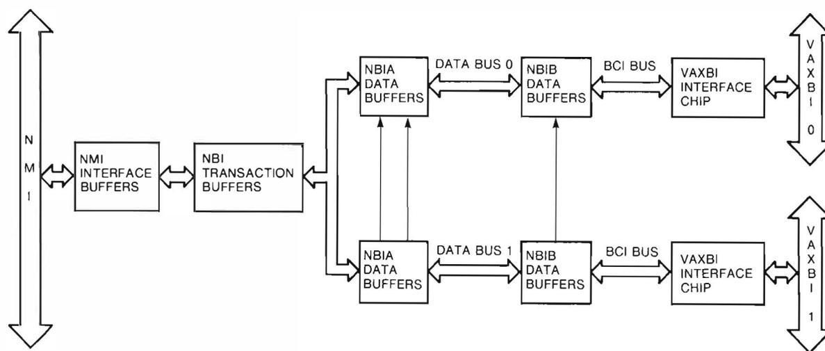
Figure 3 Block Diagram of NBI Adapter
