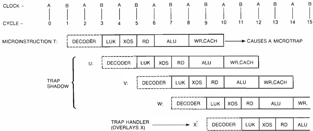
Figure 11 Microtrap Latency
