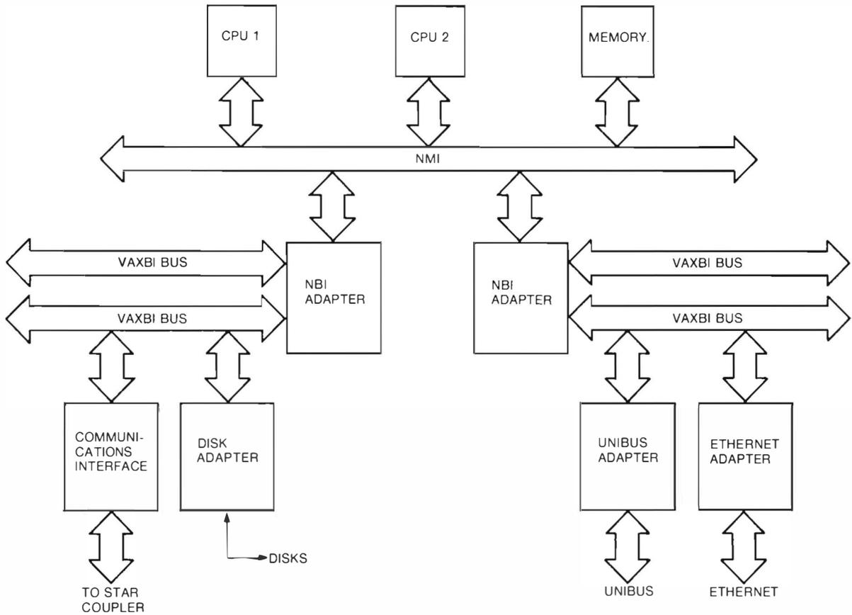
Figure 1 VAX 8800 System with Four VAXBI Buses
