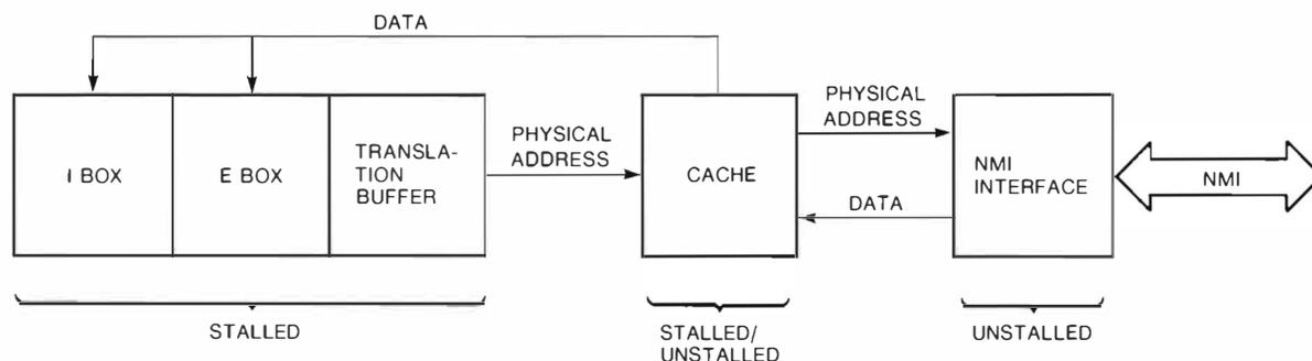
Figure 5 Stalled and Unstalled Logic in C Box
