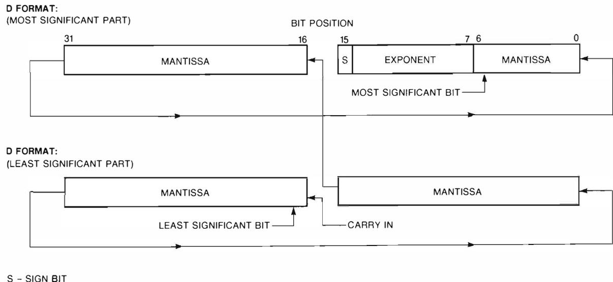
Figure 3 Floating Point Carry for D Format
