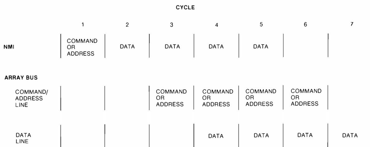
Figure 3 Cycles on NMI Bus and Array Bus
