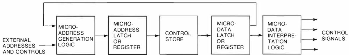
Figure 2 Block Diagram of an Abstract Micromachine
