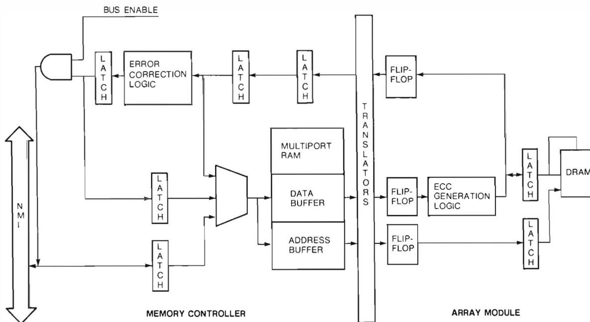
Figure 4 Datapaths in Memory Controller and Array Modules
