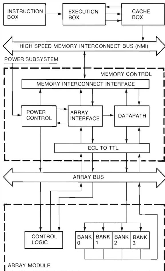
Figure 8 M Box Block Diagram
