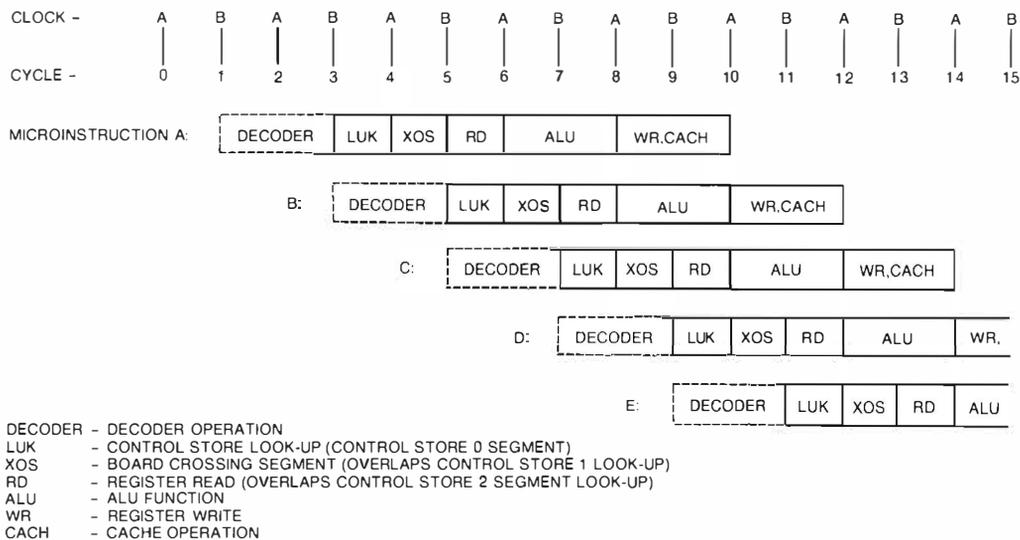
Figure 9 Microinstruction Pipeline of the VAX 8800 CPU
