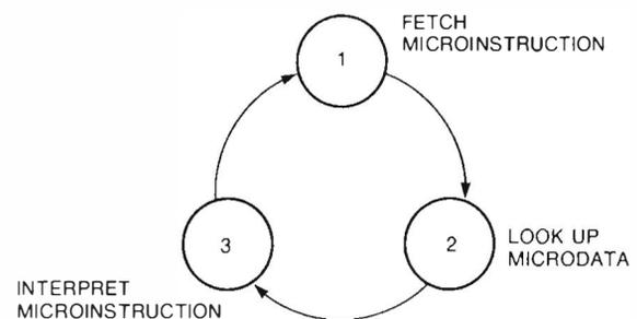
Figure 1 State-machine Model of an Abstract Micromachine
