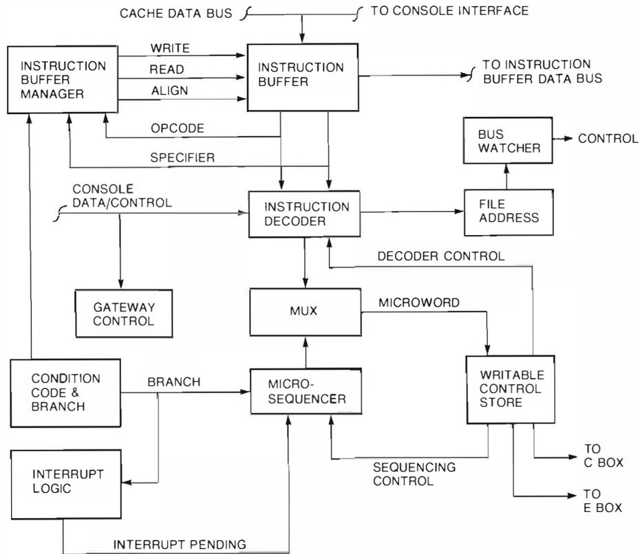
Figure 5 I Box Block Diagram
