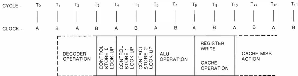
Figure 8 Canonical Times of a VAX 8800 Microinstruction
