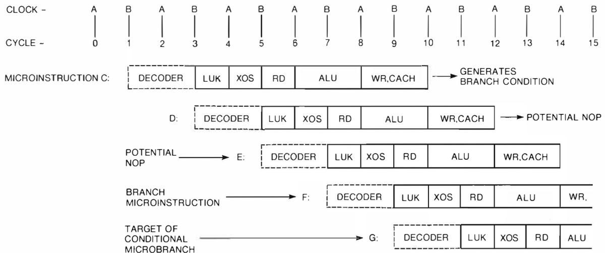
Figure 10 Microbranch Latency
