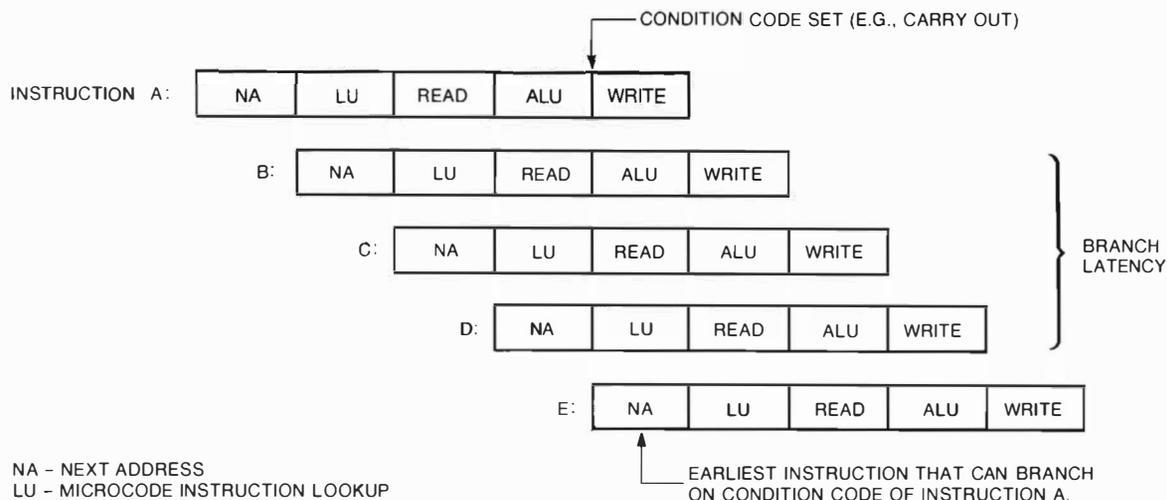
Figure 5 Five-stage Pipeline
