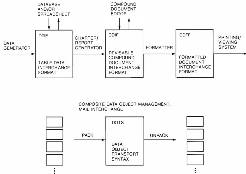
Figure 2 CDA Component Architectures
