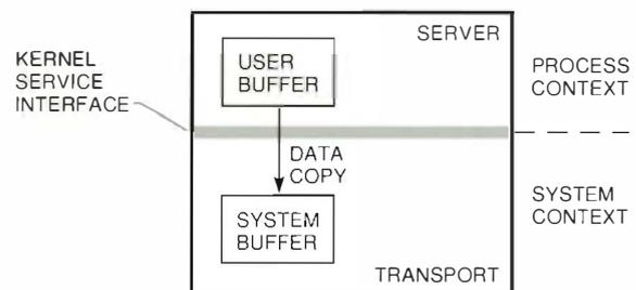
Figure 1 Data Copy with a Buffered I/O Interface
