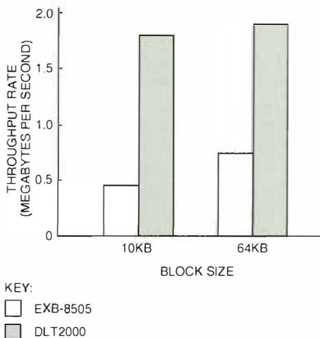
Figure 5 EXB-8505 and DLT2000 Data Throughput Rates
