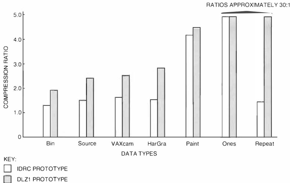
Figure 3 SDS-3 Data Compression Ratios
