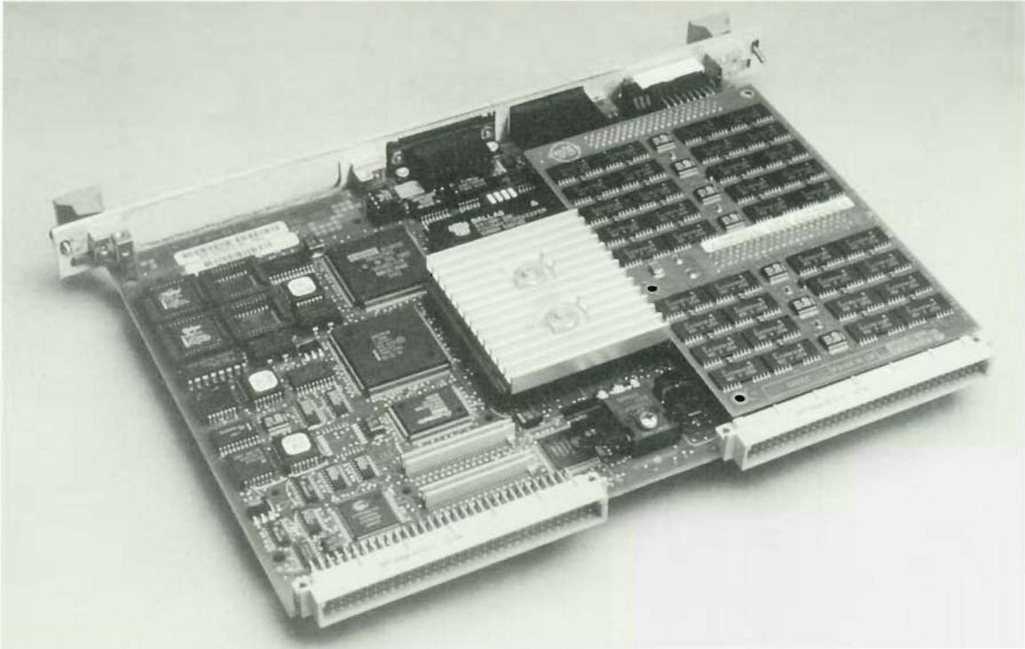
Figure 2 Digital's AXPvme 64 Single Module Computer
