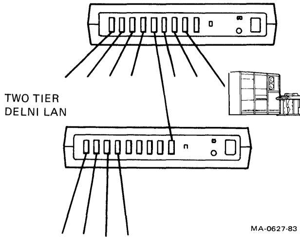
If you plan to have a large ETHERNET system which connects many work stations or covers a wide area, you can connect DELNI LANs to the ETHERNET system with an ETHERJACK junction box, or directly to an ETHERNET transceiver. Refer to Appendix A for information on connecting to these devices.
