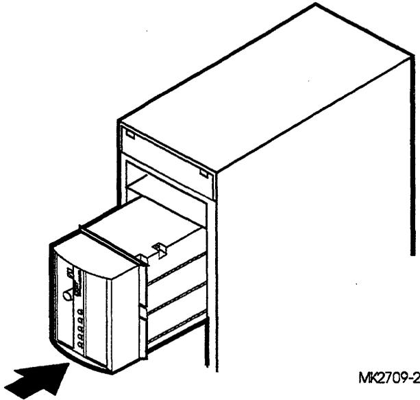
The InfoServer SW1000 takes up the top three slots in a StorageWorks pedestal. To add the InfoServer SW1000 to your existing StorageWorks pedestal, insert the SBB into the top guide slots and push it in until it is fully seated and the mounting tabs engage the shelf. Ensure that the InfoServer SW1000 is seated properly and is firmly connected to the backplane by pressing firmly on the front bezel.
