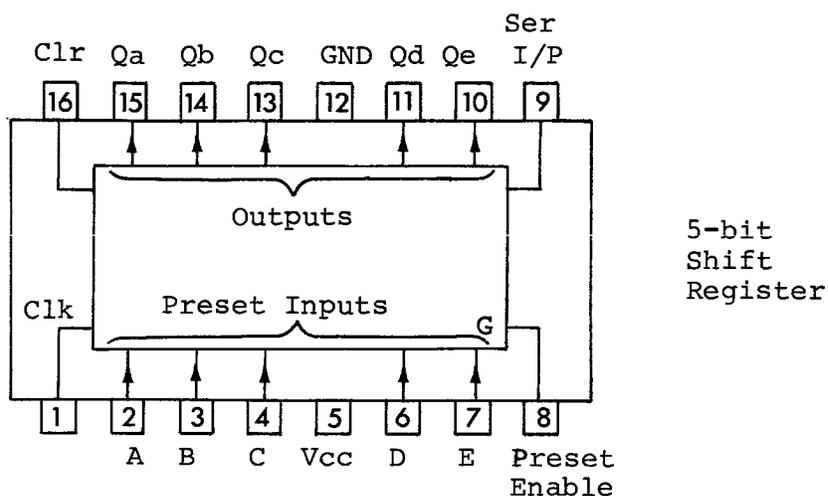
All five flip-flops in the register can be cleared by applying L to clear with preset enable or preset inputs L.
