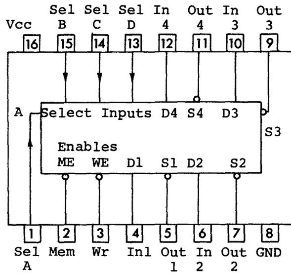
64 flip-flops arranged to give 16 4-bit words. Open collector outputs allow expansion of word length and the number of words.
