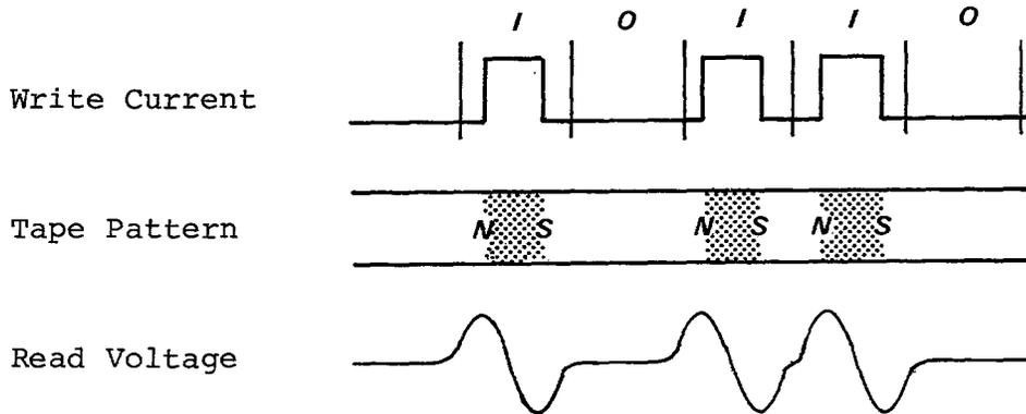
Pulses of Write Current are applied for 'ones'. Zeros are signified by absence of pulse.
