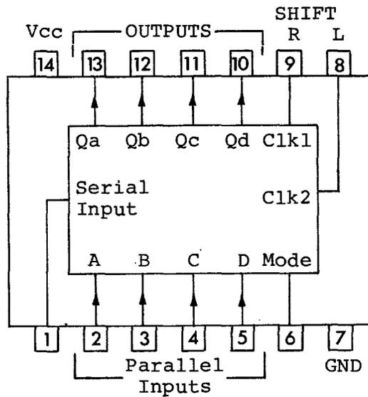
Parallel Load: Data at the parallel inputs is loaded, with mode H, and appears at the outputs after ↓ of clock 2.
