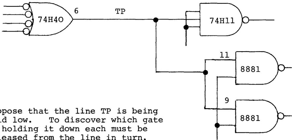
Suppose that the line TP is being held low. To discover which gate is holding it down each must be released from the line in turn.
