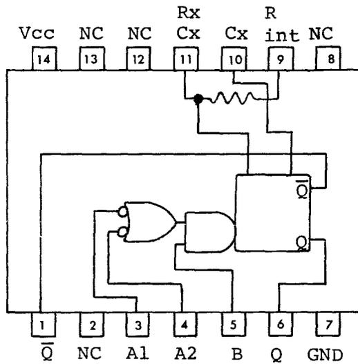
An internal timing resistor is provided. The timing capacitor is connected between pins 11 and 10.
