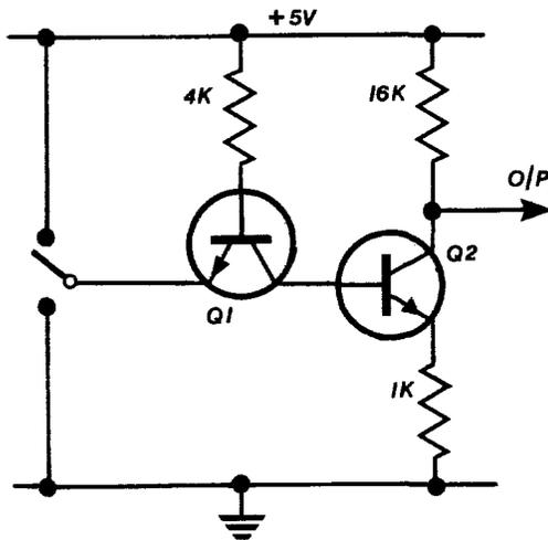
If the collector of Q1 is taken to the base of a second transistor Q2, then Q2 will be cut off when the switch is to ground (because Q2 base is taken to about  $\emptyset$  V via Q1) and the output will rise to +5V. When the switch is at +5V, the base of Q2 is high: Q2 conducts heavily and the divider effect of the 16k and 1k resistors combined with  $V_{ce}(\text{Sat})$  gives an output of about 0.7V.
