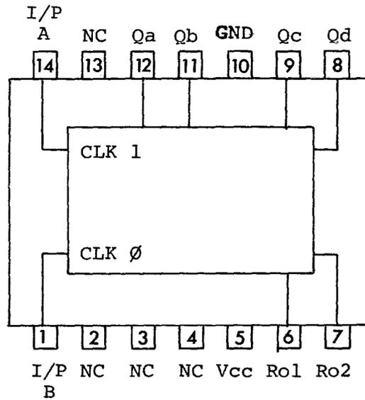
Counts the H to L transitions at I/P A. With the B I/P connected to Qa the count is:
