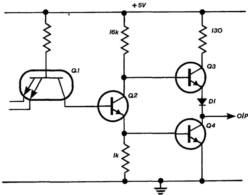
Q2 is used as a phase splitter and drives a cascade pair Q3 and Q4. When Q2 is cut off its emitter is at ground and Q4 must also be off. Q2 collector is at +5V - so is Q3 base. Q3 is therefore on and the output is High.
