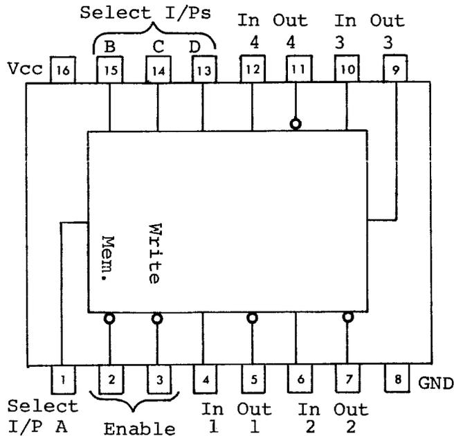
A matrix of 64 flip flops arranged to give 16 words of 4 bits each. The required word is addressed via the 4 select inputs.
