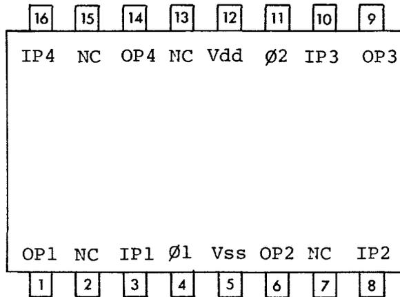
This device can be used as a quad 256-bit shift register, or a dual 512-bit shift register, or a 1024-bit shift register, by suitably interconnecting the inputs and outputs of the individual registers.
