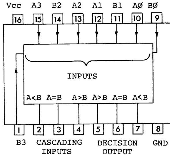
Compares two 4-bit numbers for magnitude and indicates the decision with a H on the appropriate output line.
