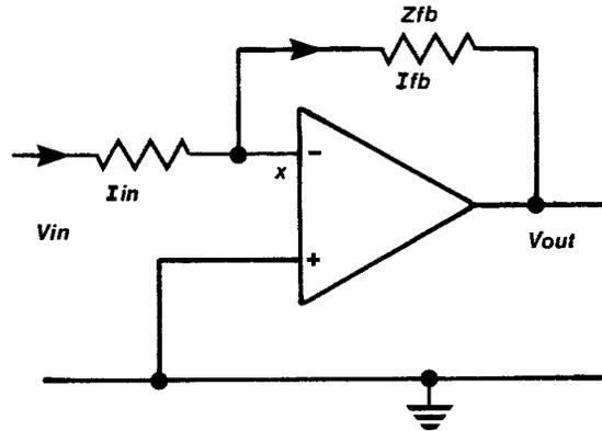
Because the gain is extremely high then the current into the amplifier at point X must be virtually zero; and if this is so then the voltage at point X must also be virtually zero. In fact, point X is a virtual Earth - approximately at ground without actually being grounded - under all operating conditions.
