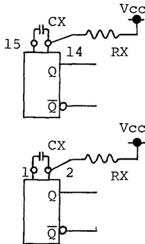
The duration of the output pulse for each monostable is set by the associated timing components:
