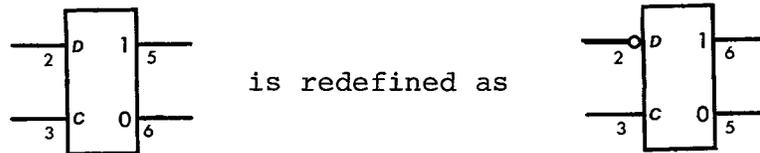
Notice that the sense of the D input is inverted to signify the change.
