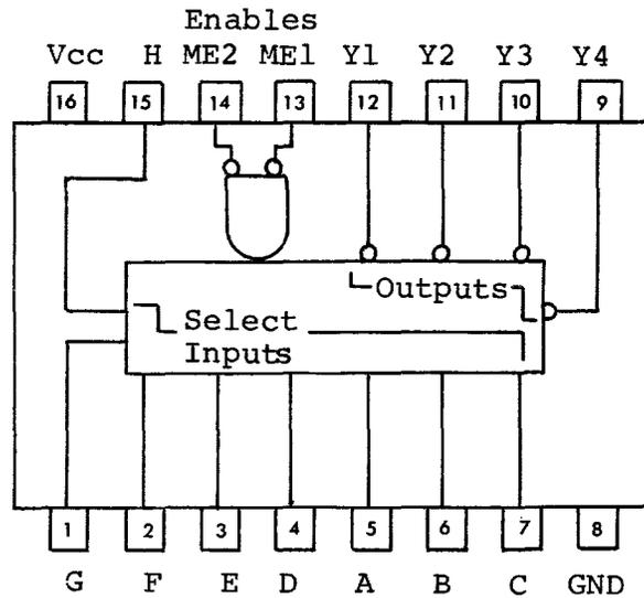
Data is entered by the manufacturer and cannot be changed. Open collector outputs.
