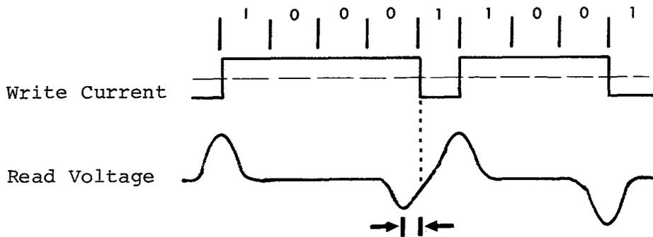
certain pulses degrade both in amplitude and timing: for two reversals close together the detected voltage for the first is just getting established when the field of the next reversal influences it causing an early peak of reduced amplitude.
