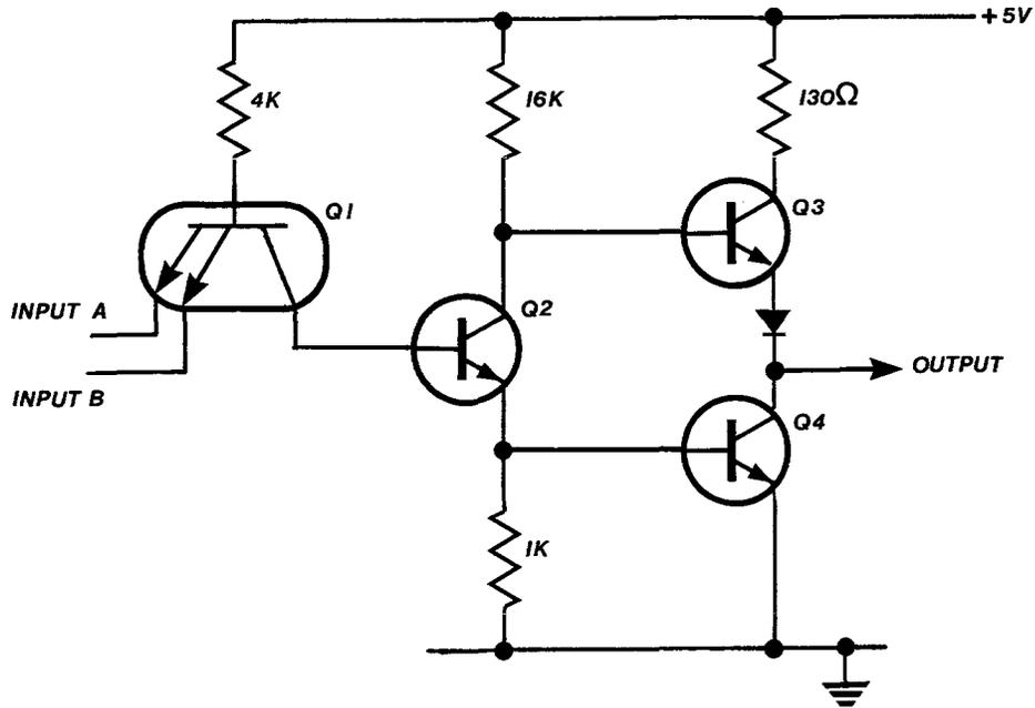
This circuit is fundamental to the system of TTL logic and yet the conventional analytical approach to its operation is not easy to grasp, especially for the technician encountering logic for the first time.
