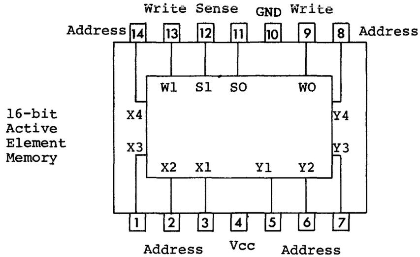
16 Flip-flops arranged in a 4 x 4 matrix. Each flip-flop is 1 bit of 16 words : the word length is determined by the number of memories connected in parallel.
