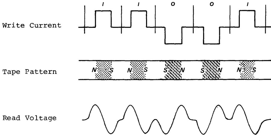
A development of the previous method with zeros written by current pulses in the opposite direction. As there is an event in each bit cell the data can be self-clocking. The greater signal range gives an improved signal to noise ratio.
