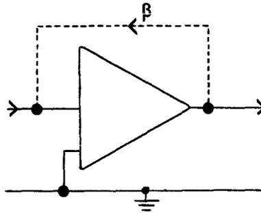
So, with Feedback,  $V_{in}$  becomes  $V_{in} + \beta \cdot V_{out}$  and since  $V_{out} = A \cdot V_{in}$
