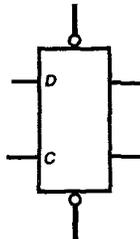
The D-type has a single information input, D. The output responds to the state of the D input
