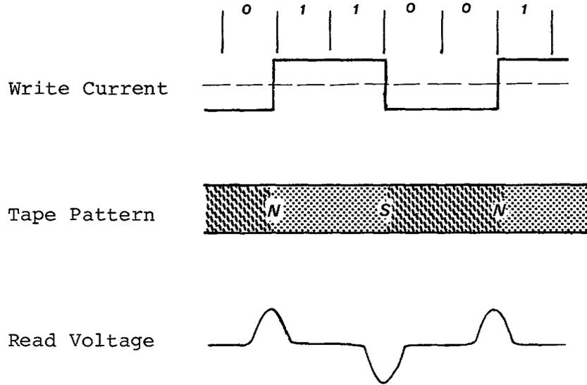
The write current reverses only on bit changes, i.e. 0 to 1 or 1 to 0.
