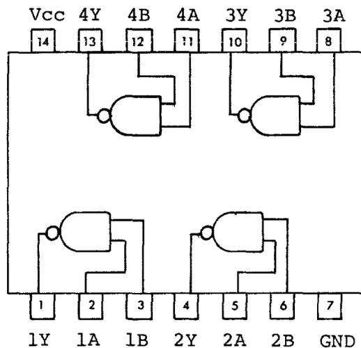
Low output leakage current. Open collectors.
