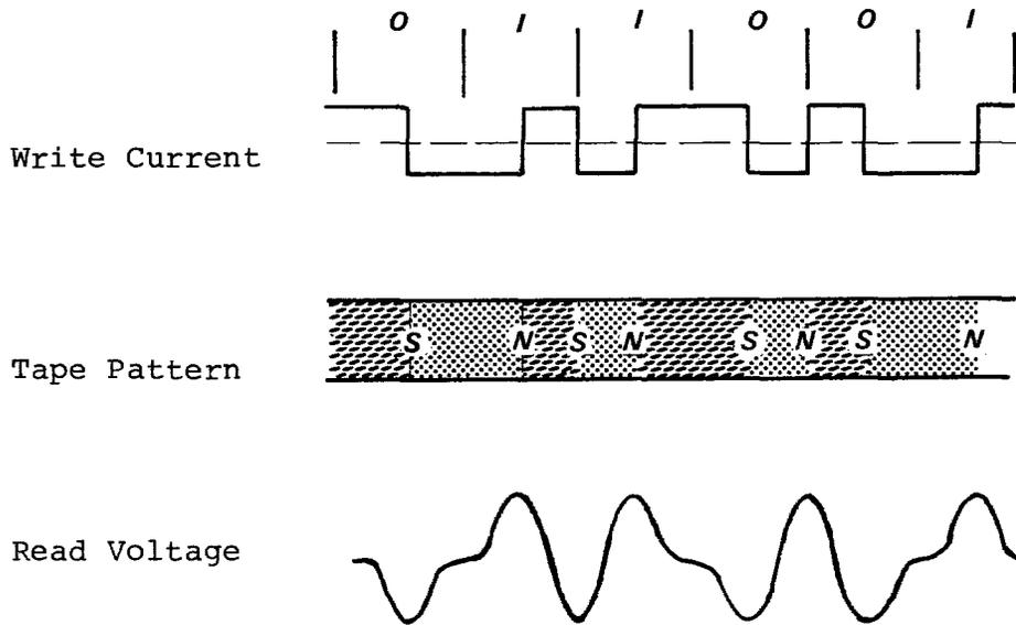
A 1 is indicated by a flux reversal in one direction and a 0 by a reversal in the other direction. Information is retrieved by merely detecting the polarity of the output pulses.
