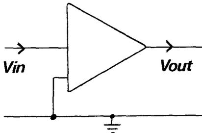
If we feed back a portion of  $V_{out}$  the performance of the amplifier is modified. The fraction of  $V_{out}$  fed back is designated  $\beta$  so
