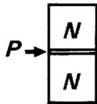
We usually think of the transistor as its symbol is drawn, with the base controlling the flow of electron current from emitter to collector. But, when a transistor is used as a switch it will still work if the collector and emitter are interchanged: both are N-type and even in discrete transistors where emitter and collector dopings are markedly different, the device will still function upside-down.
