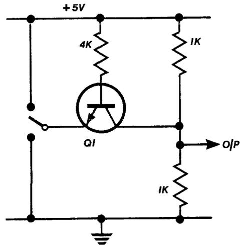
When the switch is taken to +5V the transistor works upside-down; the emitter behaves as a collector and the collector as an emitter. Now the transistor is on (still with its base high) but this time the output point is connected to +5V via an "ON" transistor so output goes to about +5V.
