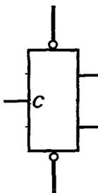
Most flip-flops have a clock input that controls the insertion of binary data. The clock pulse usually causes the flip-flop to record the input state prevailing before the pulse.
