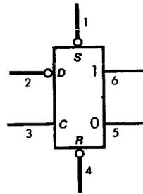
One final complication. Sometimes outputs are shown twice on the same flip-flop - one for each sense of the output. In other words an output is drawn for the circuits it affects when Hi and again for those it affects when Lo.
