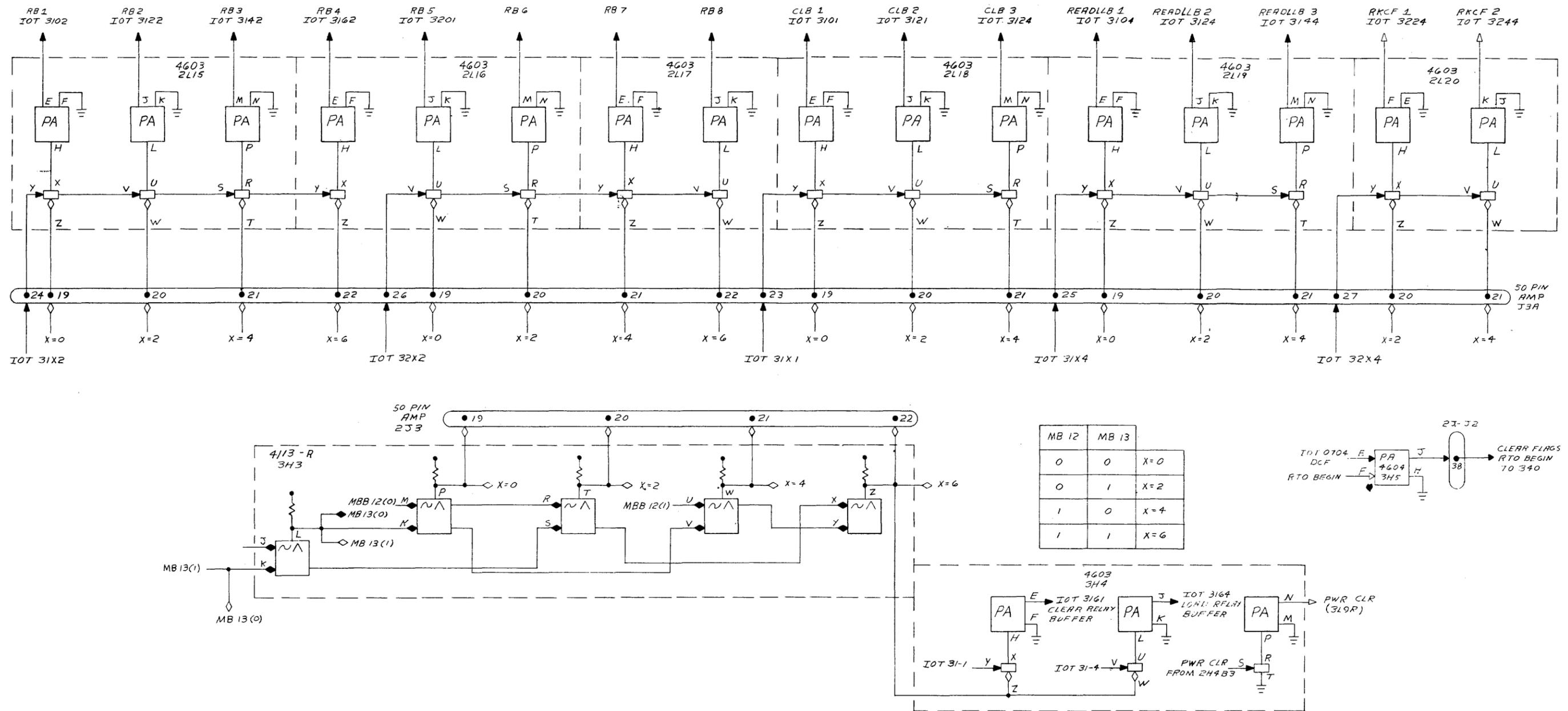
Figure 4-10 IOT and MB Decoding
