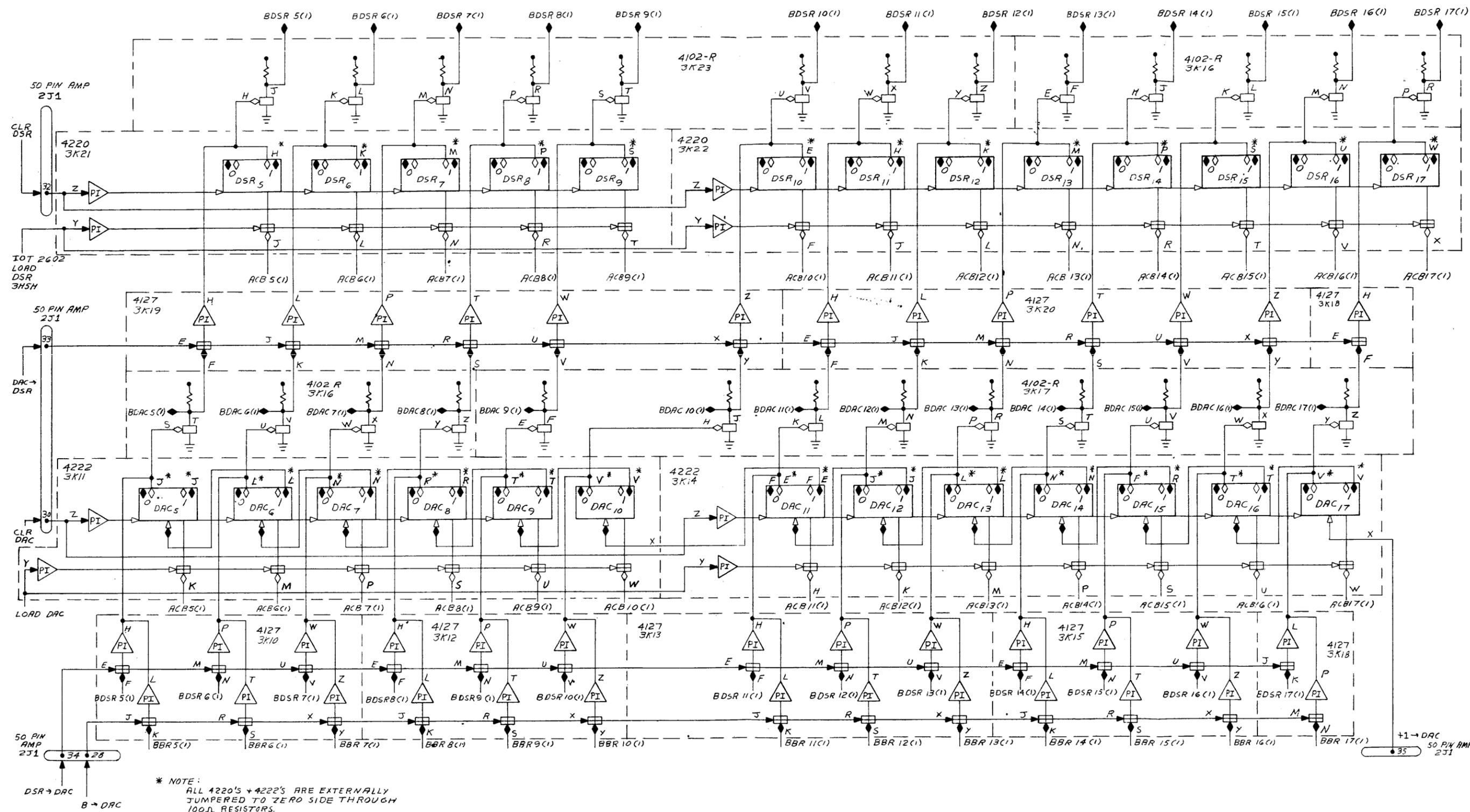
Figure 4-20 Address and Save Registers
