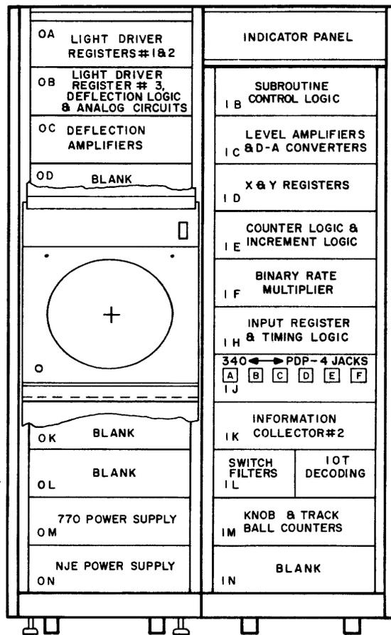
Figure 1-3 Modified Type 340 Display Rack Layout
