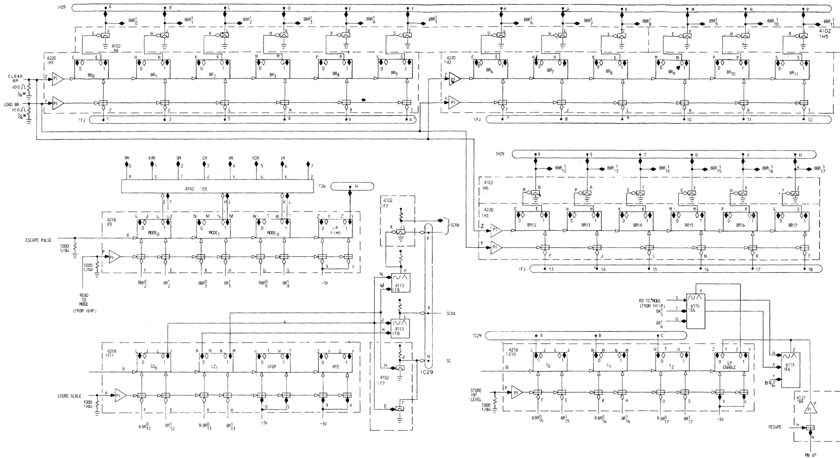
Figure 4-13 Buffer Register and Parameter Registers
