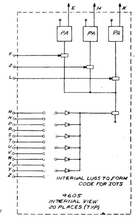
Figure 4-21 Device Selector IOT Decoding
