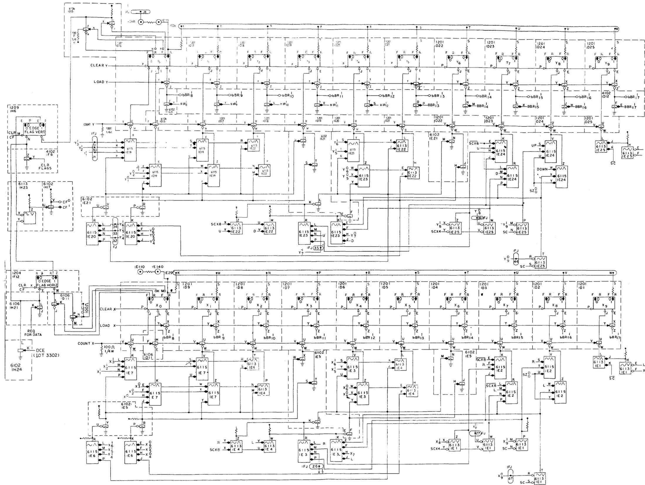
Figure 4-11 Horizontal and Vertical Deflection Registers
