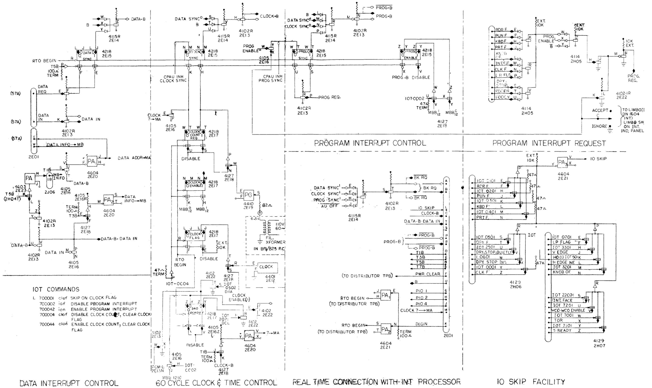
Figure 4-2 Type 125 Real Time Control
