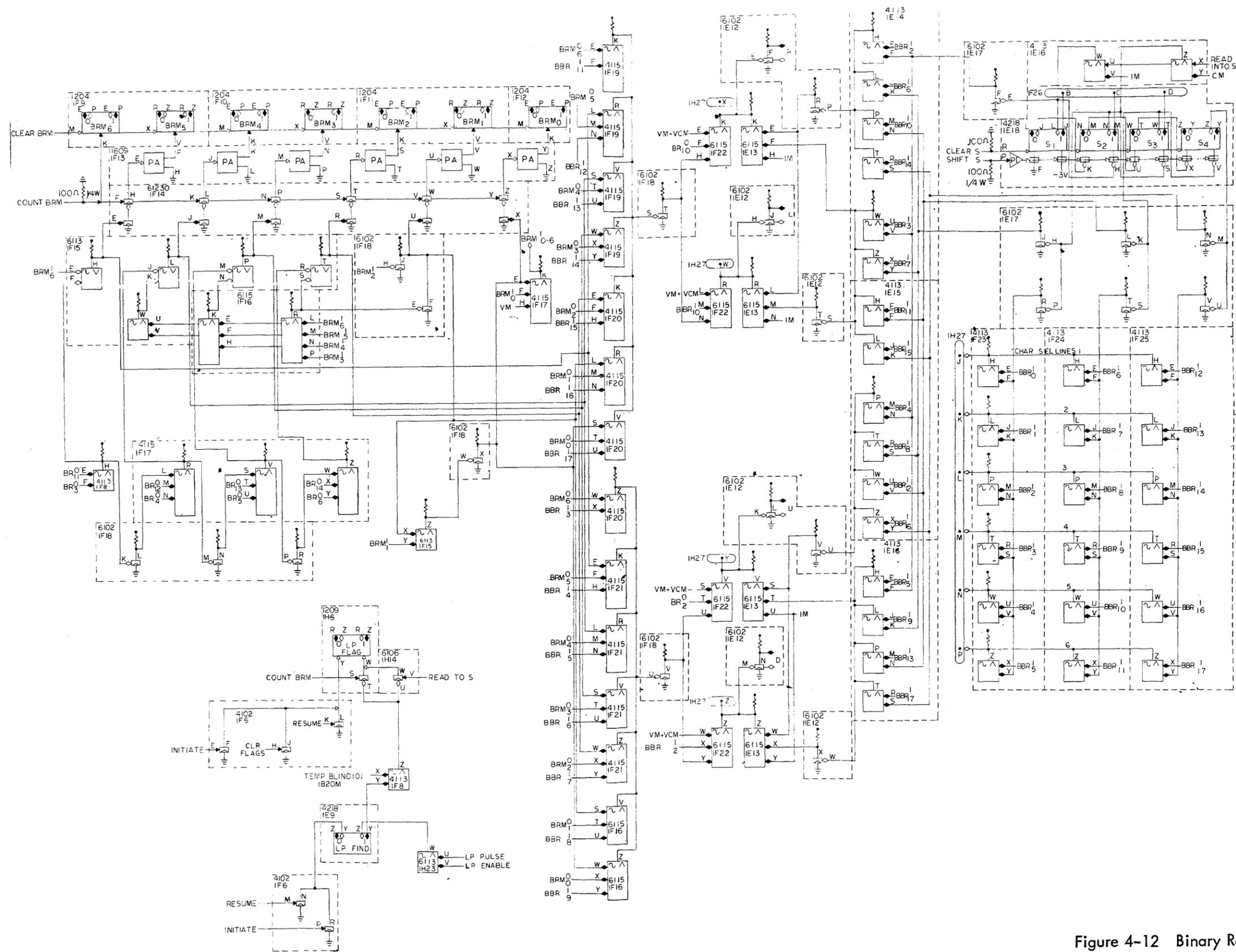
Figure 4-12 Binary Rate Multiplier and Increment Logic
