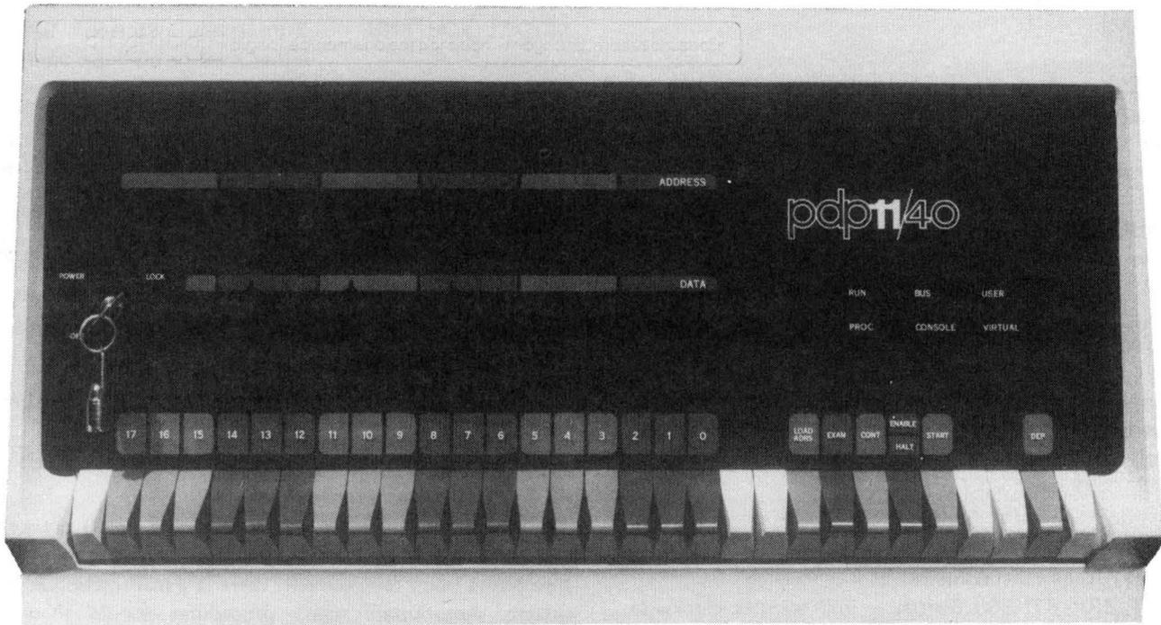
Figure 2 PDP-11/40 Programmer's Console
