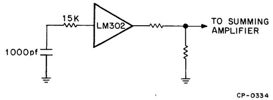
Figure 2-42 LM302 Diagram
