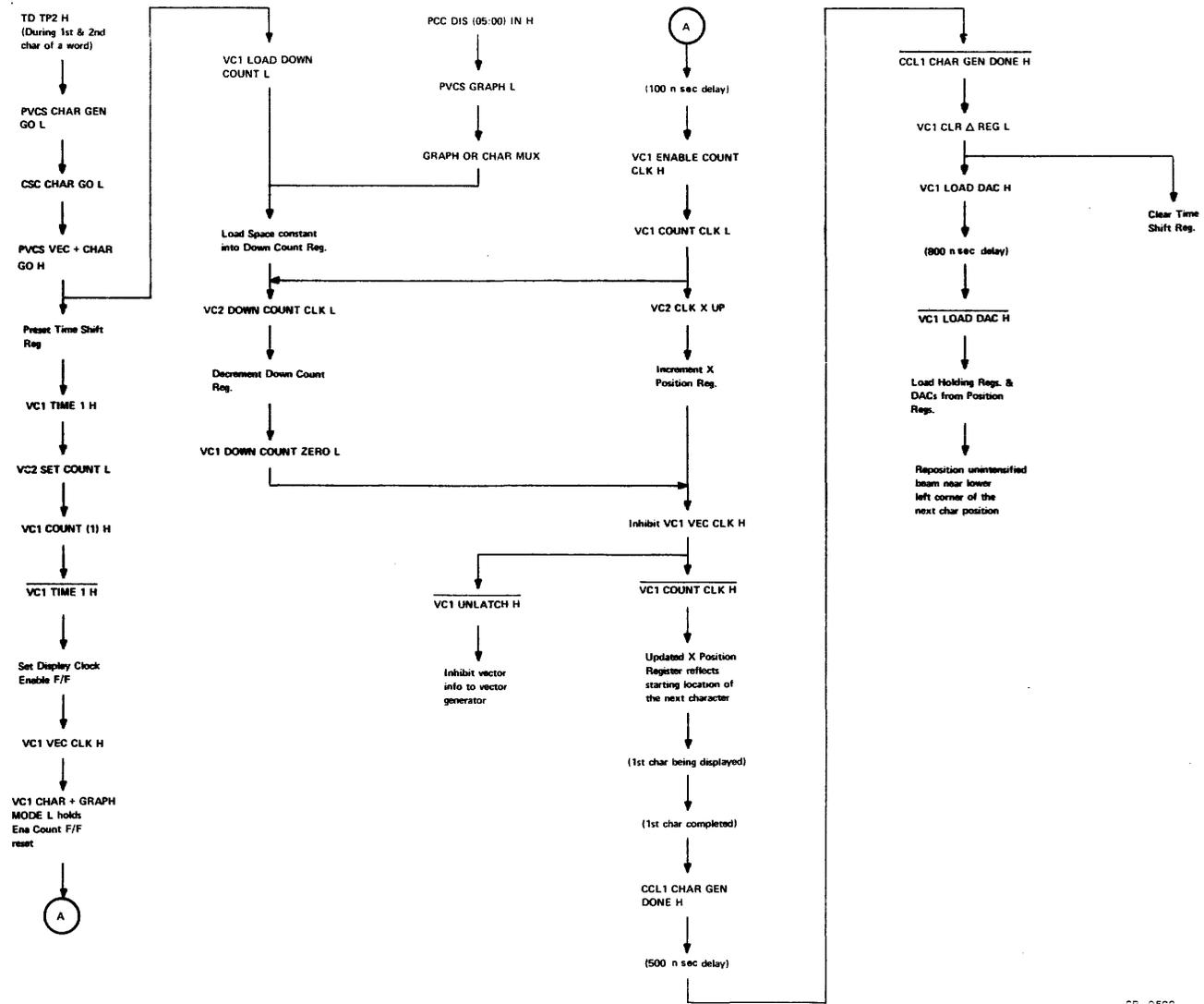
Figure 2-37 Intercharacter X Position Update, Flow Diagram
