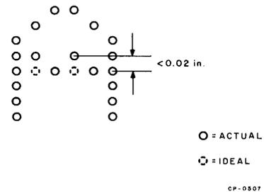
Two adjustments, R9 on the M7013 module and R134 on the A320 module, control character display. Their function is described in Paragraph 3.1.1.
