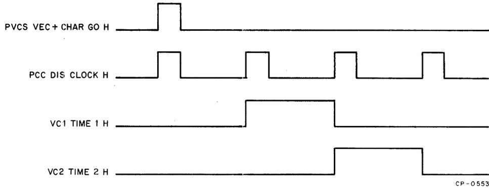
Figure 2-38 Time Shift Register, Timing Diagram (M7014YA-VC1)
