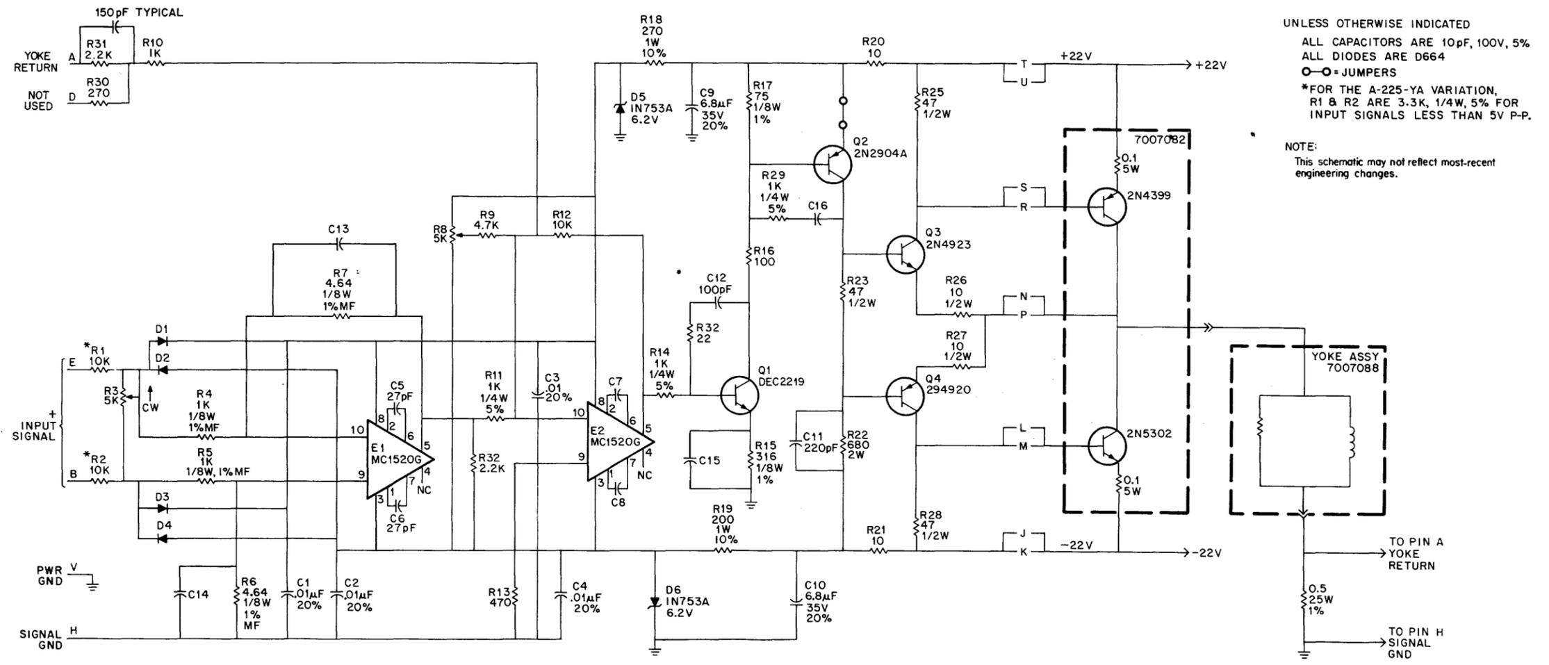
Figure 3-1 X and Y Deflection Circuit
