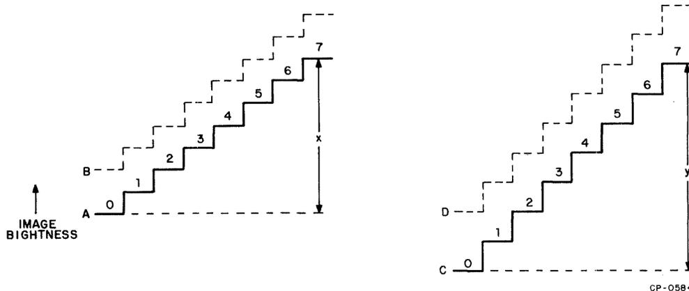
Figure 3-6 VR14L/VR17L Brightness and Contrast Control
